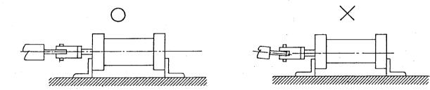
5-7 When the load acting direction changes with the cylinder operation, use an oscillating cylinder (clevis type or trunnion type) capable of making revolution to a certain angle. Furthermore, install the rod end connecting metal (knuckle) so that it moves in the same direction as the cylinder main body.
