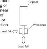
■ Mounting the attachment When mounting the attachment to the finger, to prevent any effect on the gripper, support with a wrench, etc., when tightening so that the finger is not twisted.
