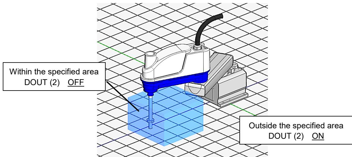
If the current position of the robot is within the specified area, DOUT (2) is turned off; otherwise, DOUT (2) is turned on.
