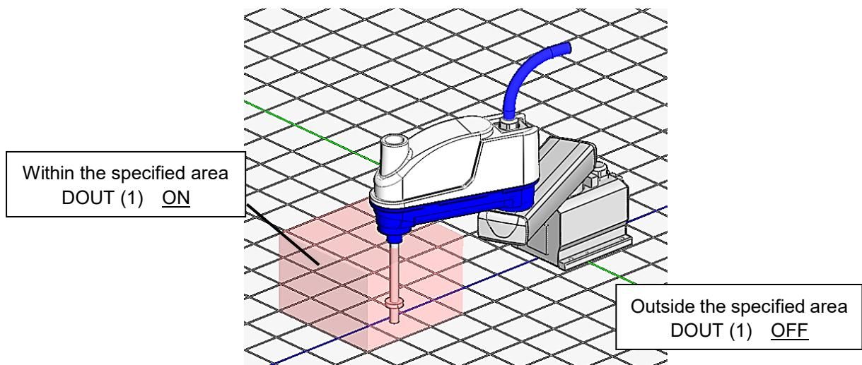
If the current position of the robot is within the specified area, DOUT (1) is turned on; otherwise, DOUT (1) is turned off.
