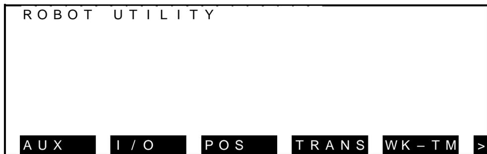
Press the **F2** key (**I/O**) on the teach pendant, and the external input/output signal display appears. The following standard input signal status display is shown.
