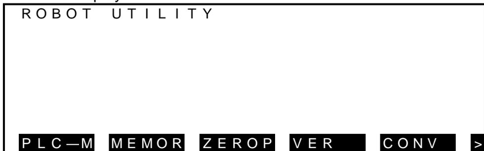
Press the **F4** key (**VER**) on the teach pendant, and the version information display appears. If the **F-ETH** is not shown, an optional board other than the EtherNet/IP board may be mounted on the robot controller.
