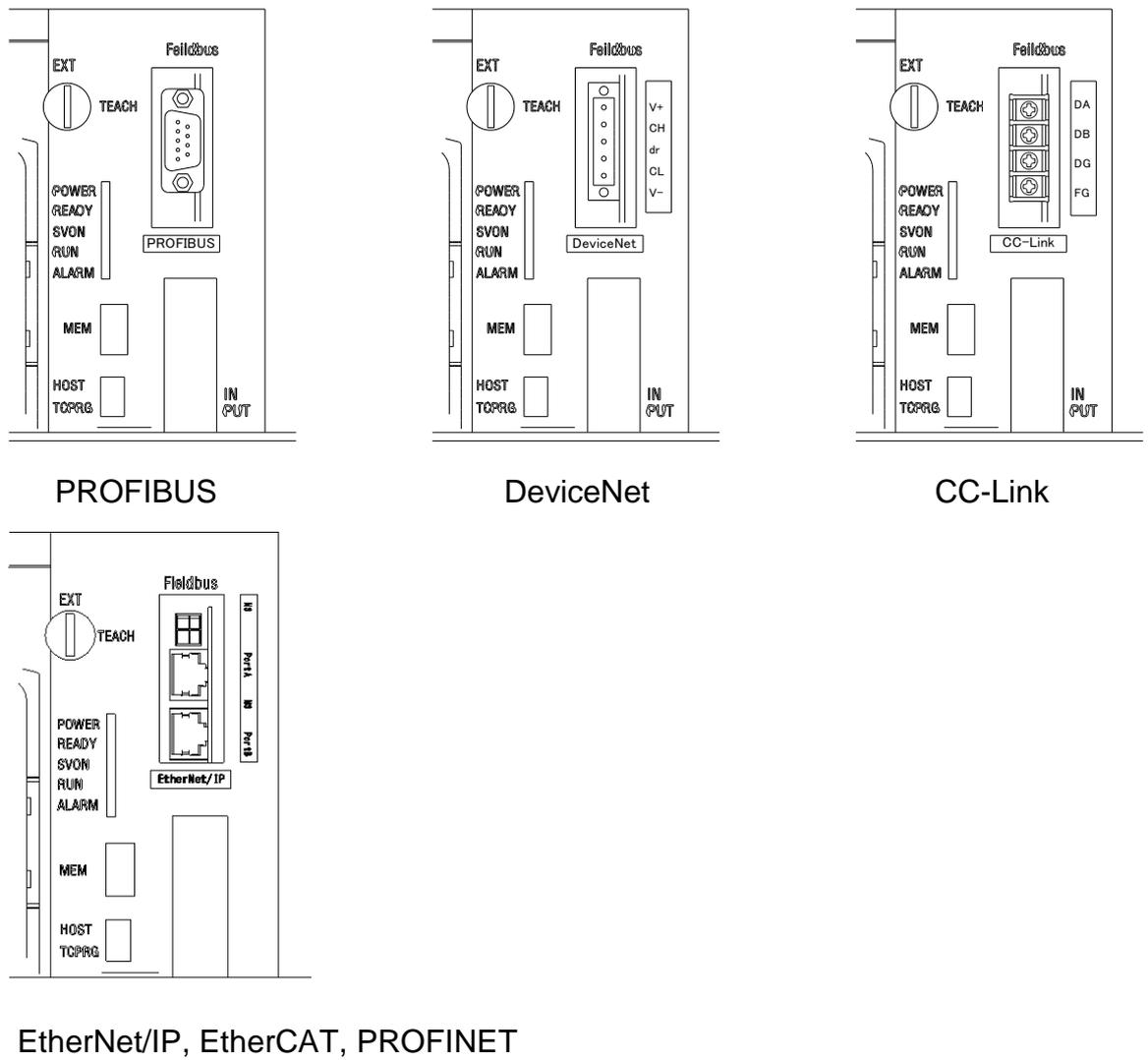
Fig. 8 KSL3000 Controller Front Panel
