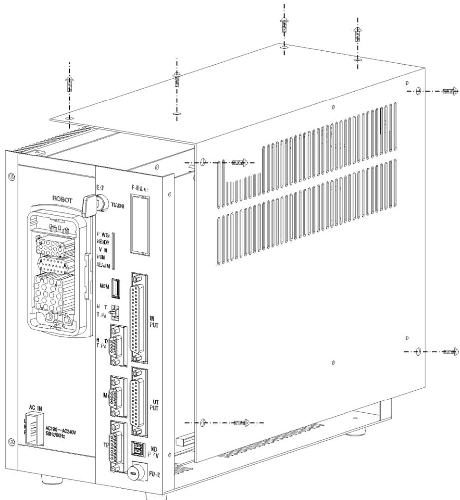
Fig. 5 Removing the KSL3000 Cover
