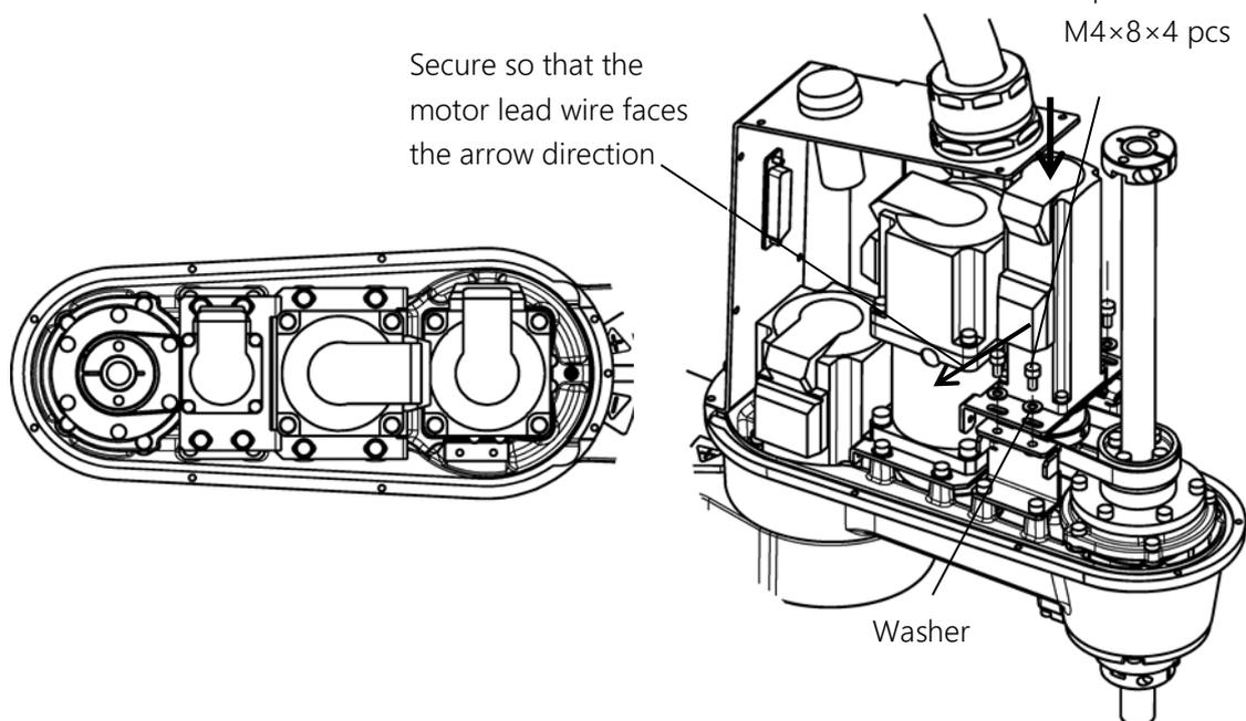
Fig. 7.23 Fitting the axis-3 motor assembly
