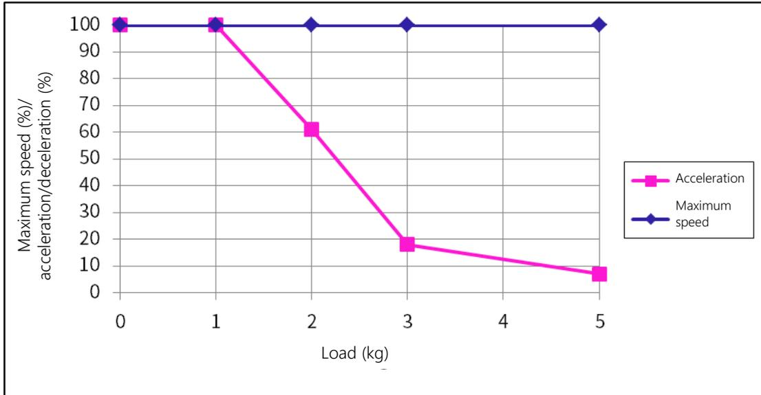
Setting of maximum speed and acceleration/deceleration in relation to load mass (Axis 3)
