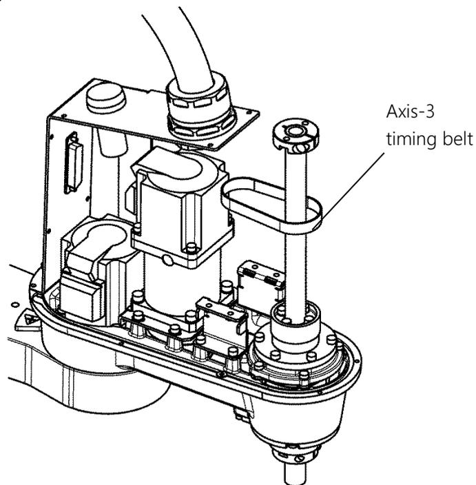
Fig. 7.28 Replacing the axis-3 timing belt
