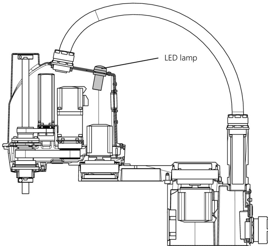
Fig. 7.58 Location of the LED lamp
