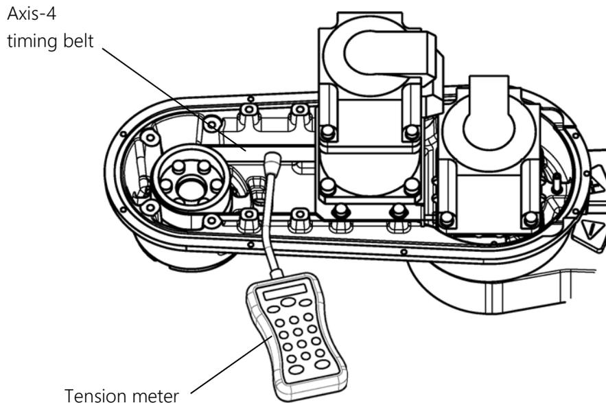
Fig. 7.54 Measuring the Tension of the Axis-4 Timing Belt
