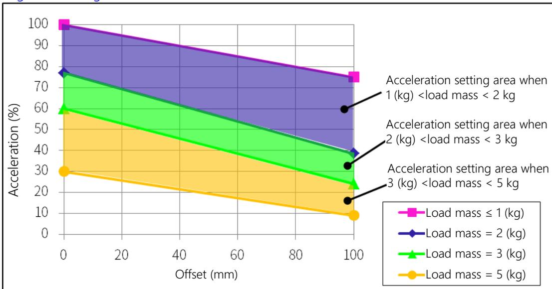
Setting of acceleration/deceleration in relation of offset (Axis 1)
