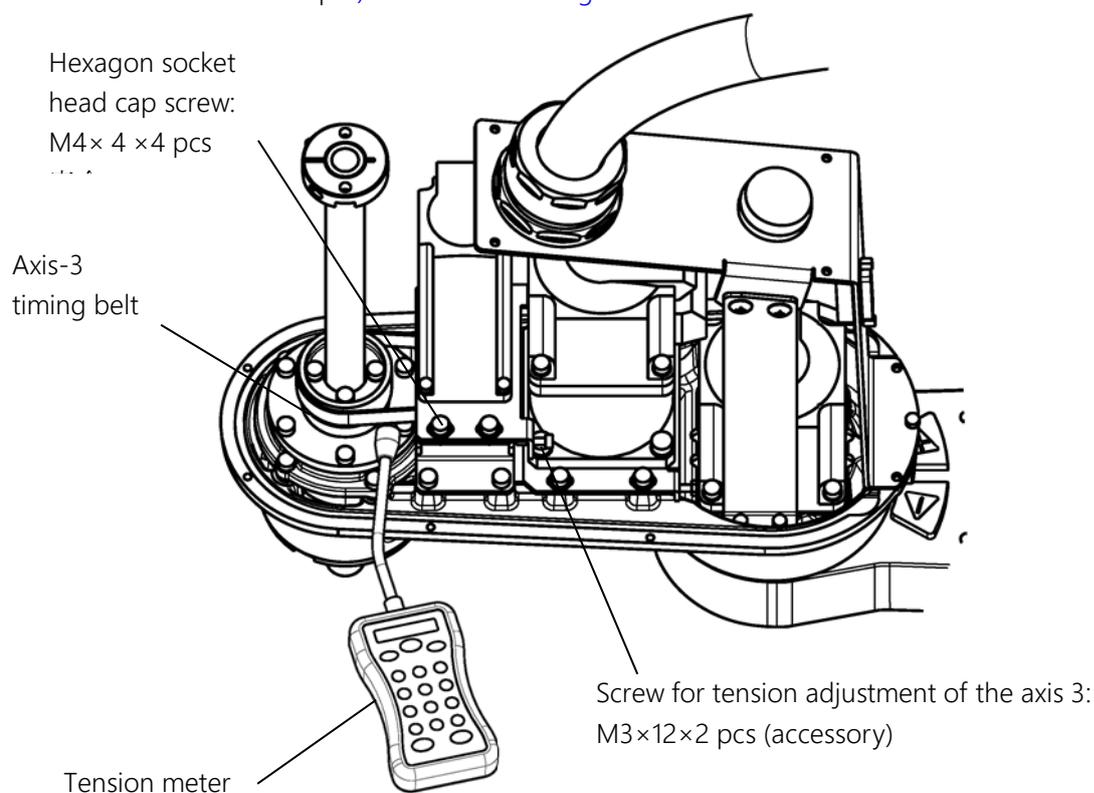
Fig. 7.24 Adjusting the tension of the axis 3
