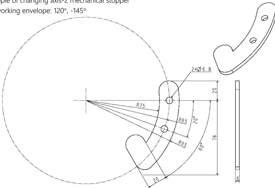
Fig. 3.5 Example of changing axis-2 mechanical stopper
