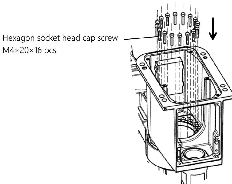
Fig. 7.49 Fitting the Arm 1
