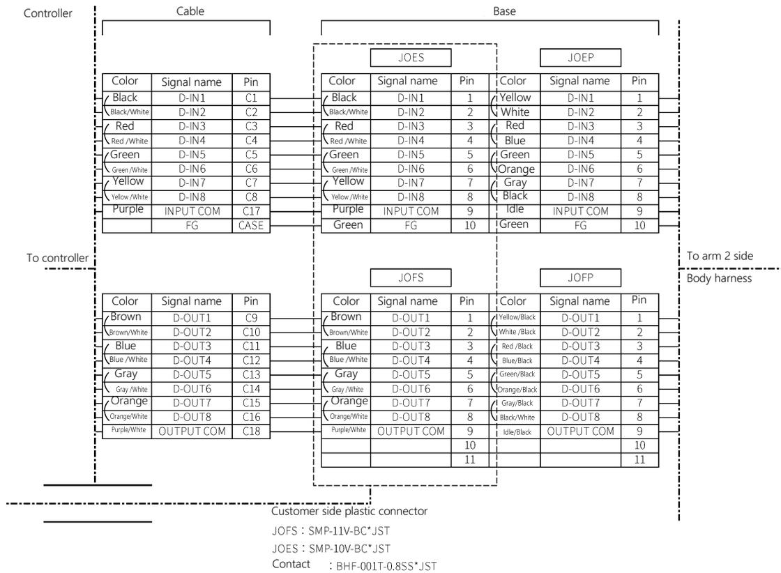
Fig. 5.6 Hand wiring diagram base side (common to Type-N, P KSL3000)
