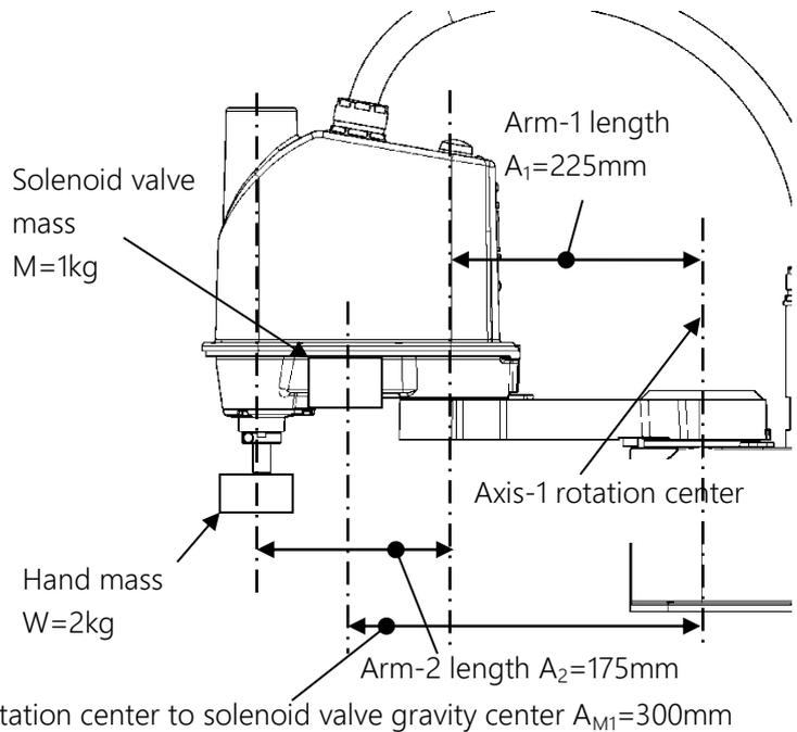
Fig. 4.7 Mounting between axis-1 rotation center and axis-3 center
