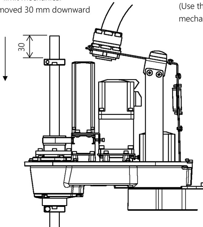
Fig. 3.8 Changing axis-3 working envelope
