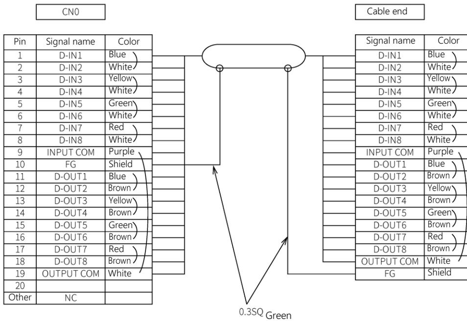
Fig. 5.12 Hand I/O cable (option) wiring diagram
