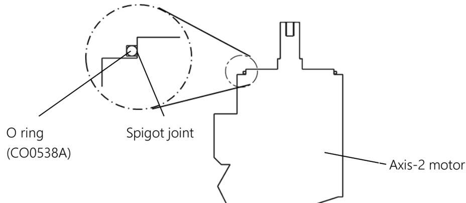
Fig. 7.16 Fitting O ring
