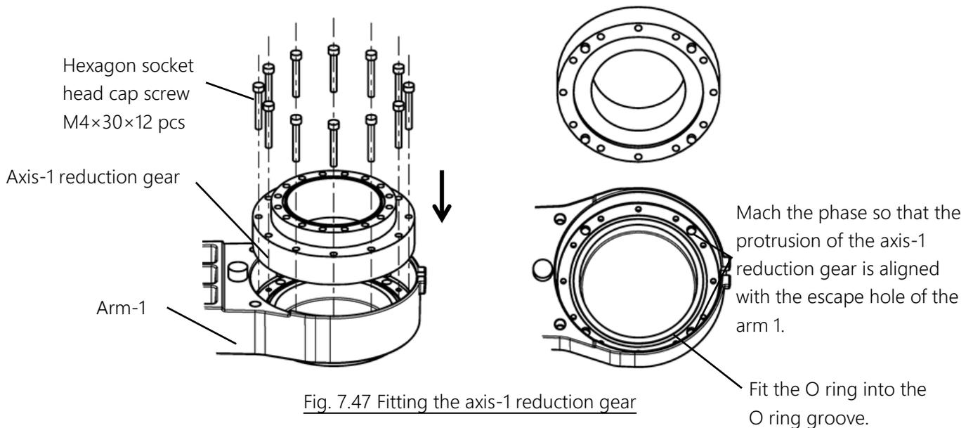
Fig. 7.47 Fitting the axis-1 reduction gear
