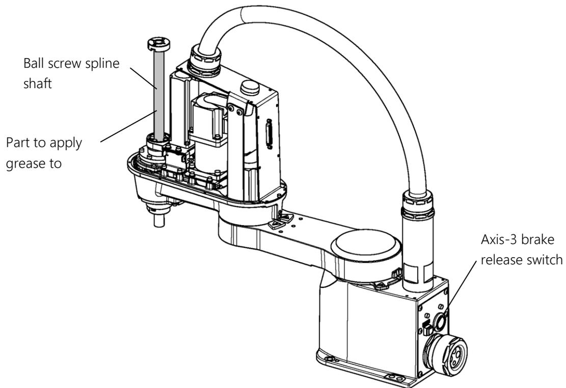
Fig. 7.38 Greasing up the upper side of the ball screw spline unit
