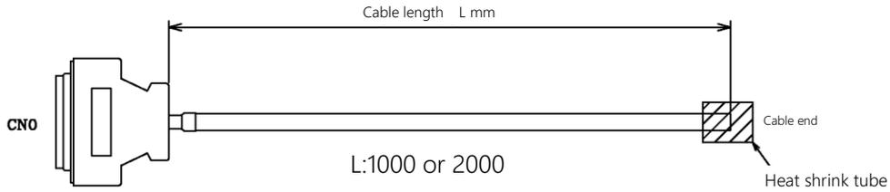
Fig. 5.11 External view drawing of hand I/O cable (option)
