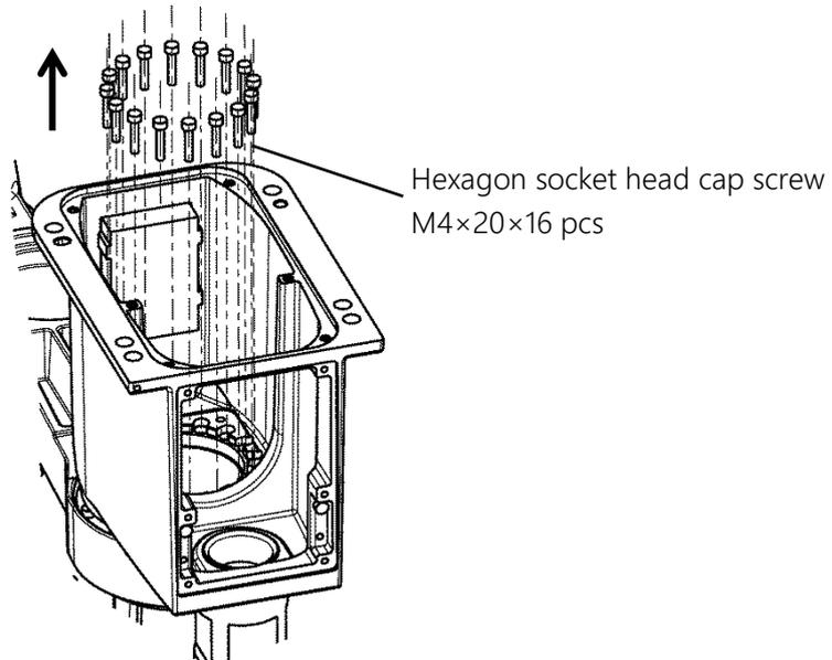
Fig. 7.45 Removing the arm 1
