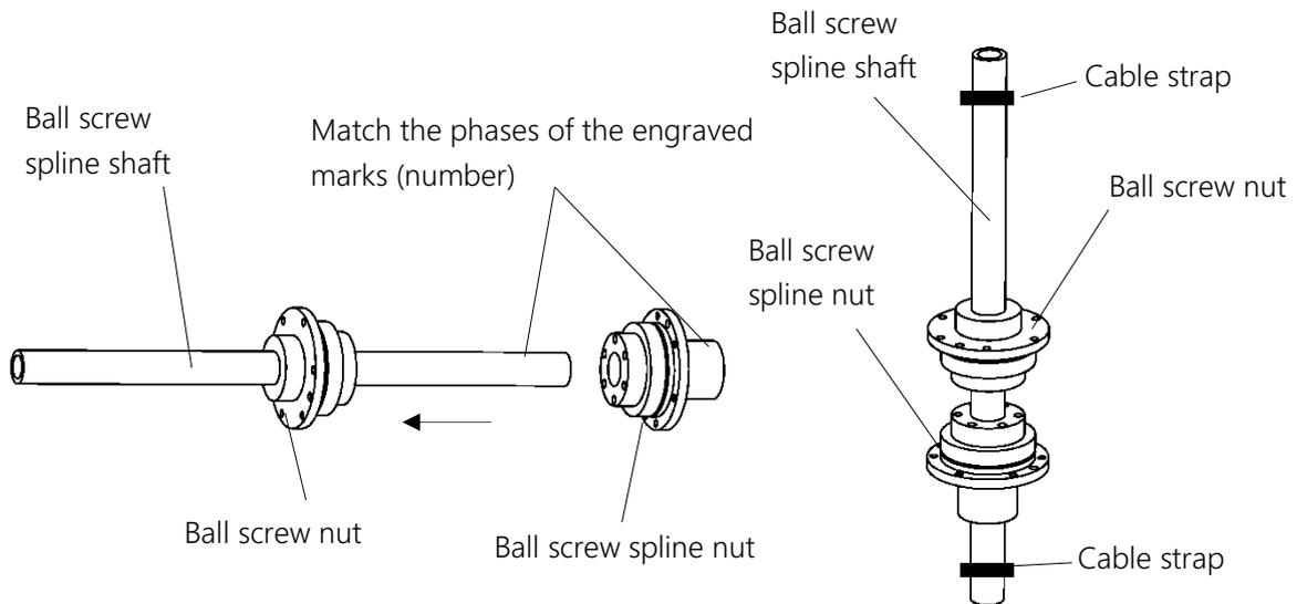
Fig. 7.41 Ball screw spline unit
