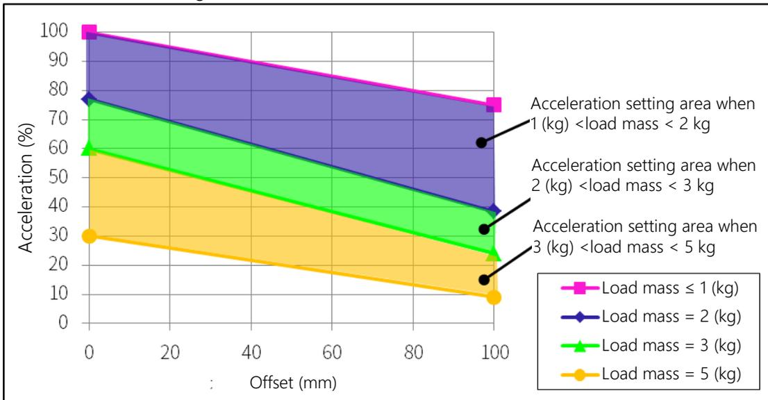
Setting of acceleration/deceleration in relation to offset (Axis 2)
