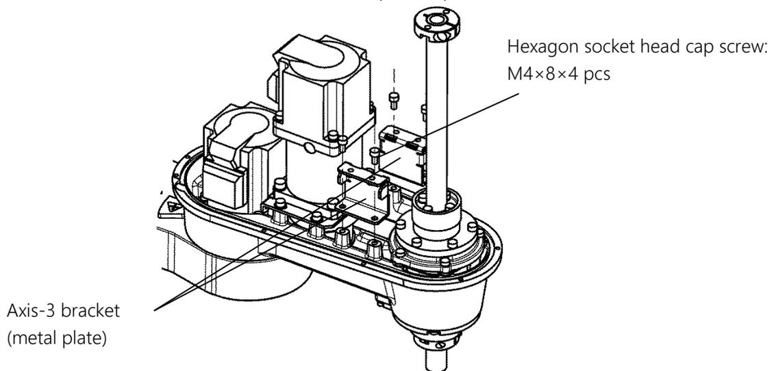
Fig. 7.30 Removing the axis-3 bracket (metal plate)
