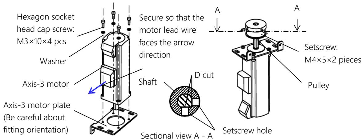
Fig. 7.22 Fitting the axis-3 pulley and plate
