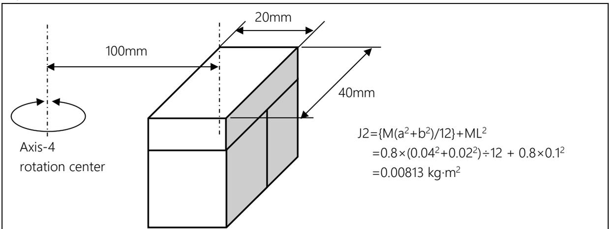
3) Moment of inertia of workpiece
