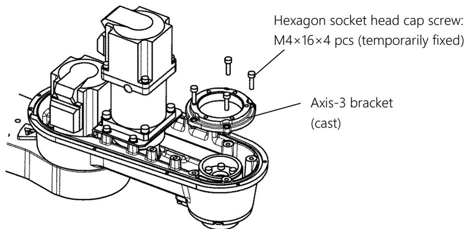
Fig. 7.34 Fitting the axis-3 bracket (cast)
