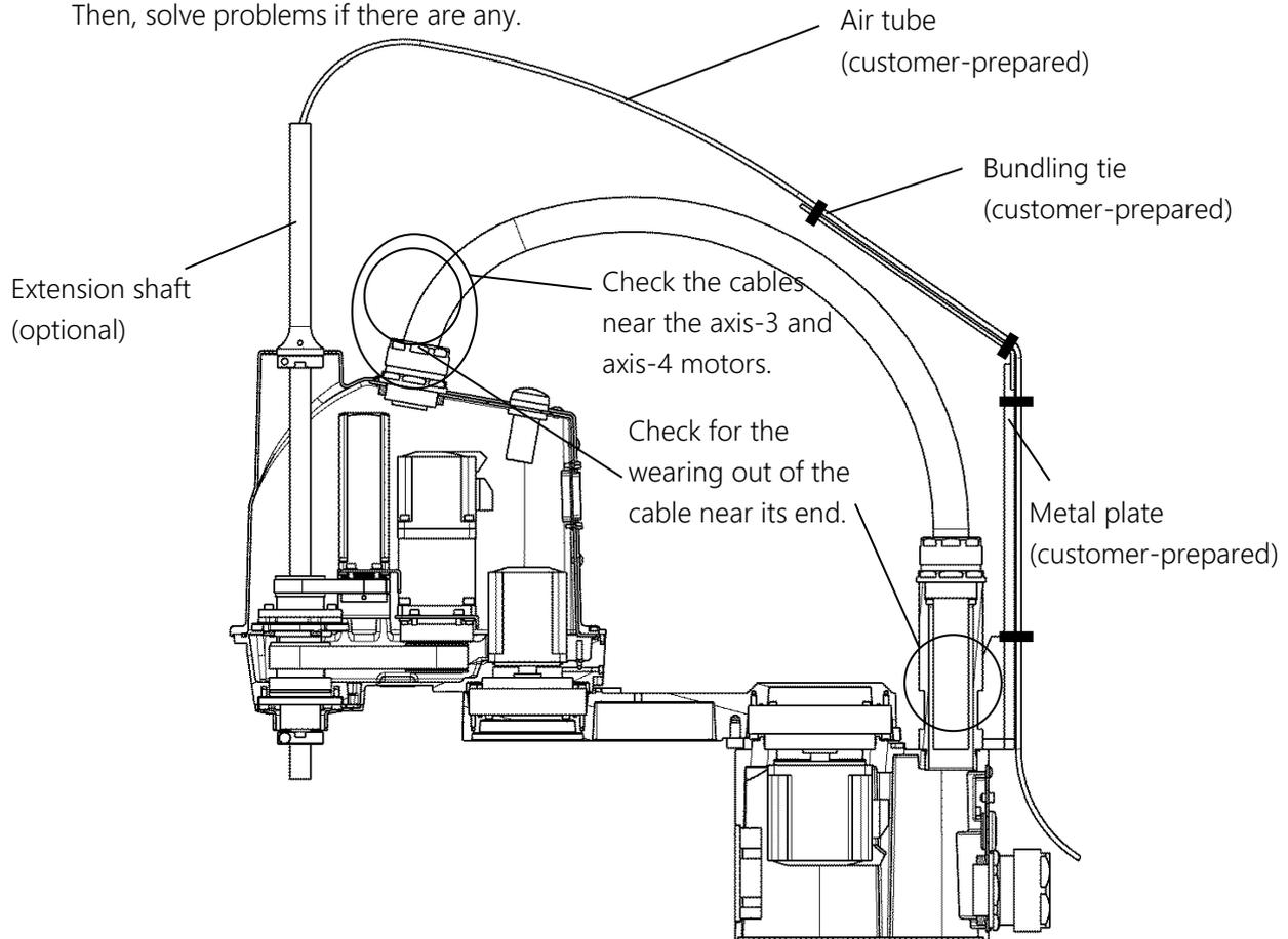
Fig. 7.3 Inspection points of cable
