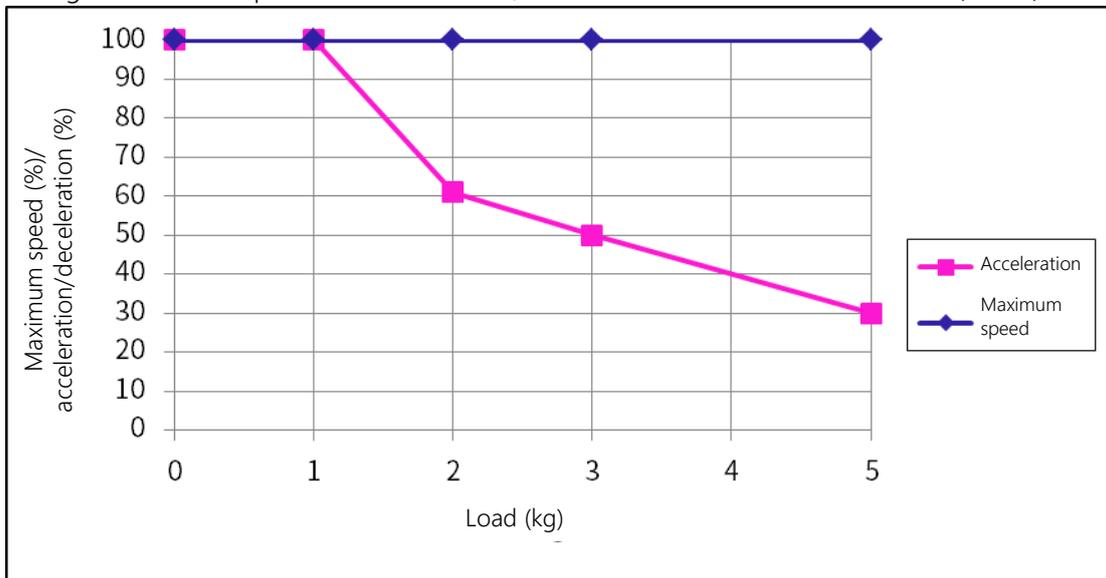
Setting of maximum speed and acceleration/deceleration in relation to load mass (Axis 4)
