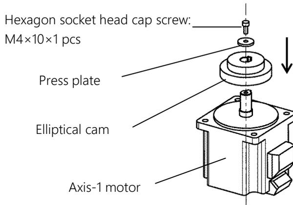
Fig. 7.12 Fitting axis-1 elliptical cam
