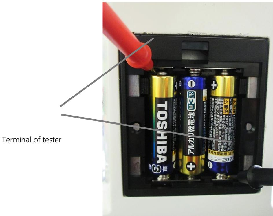
Fig. 8.4 Checking the Battery for Fitting Failure
