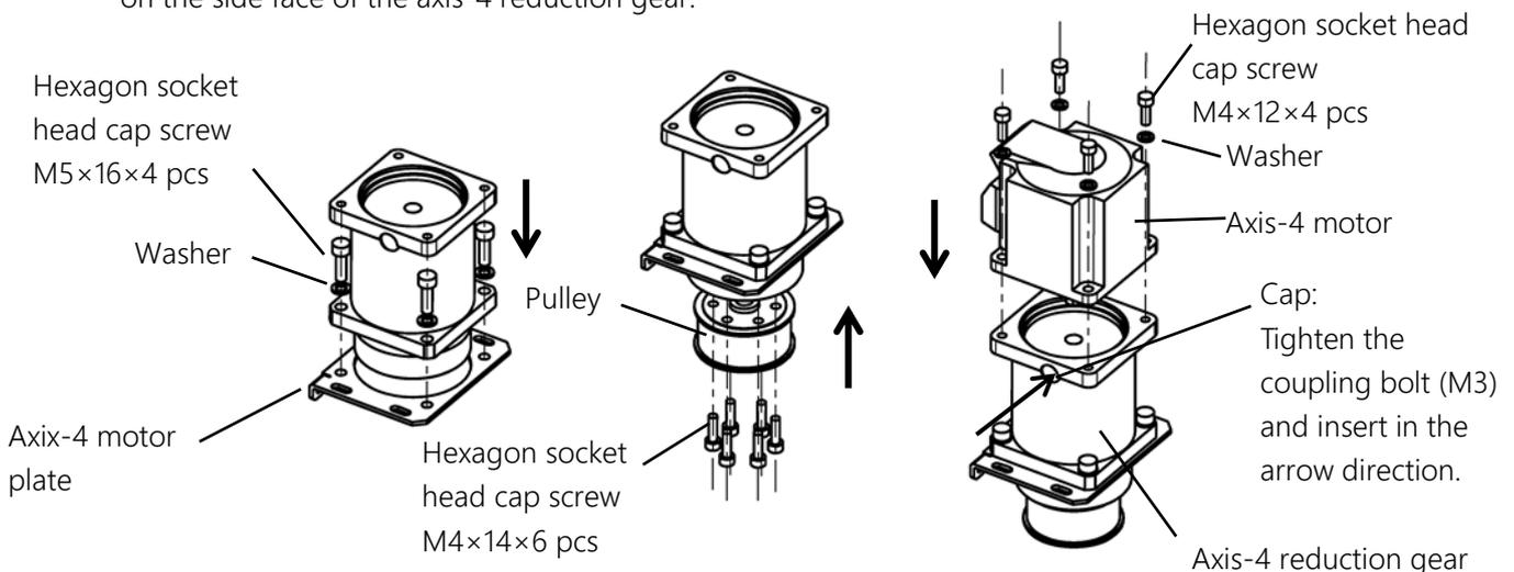
Fig. 7.56 Fitting the axis-4 reduction gear
