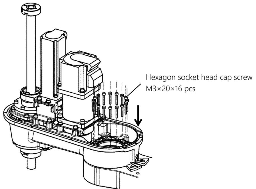
Fig. 7.53 Fitting the Arm 2
