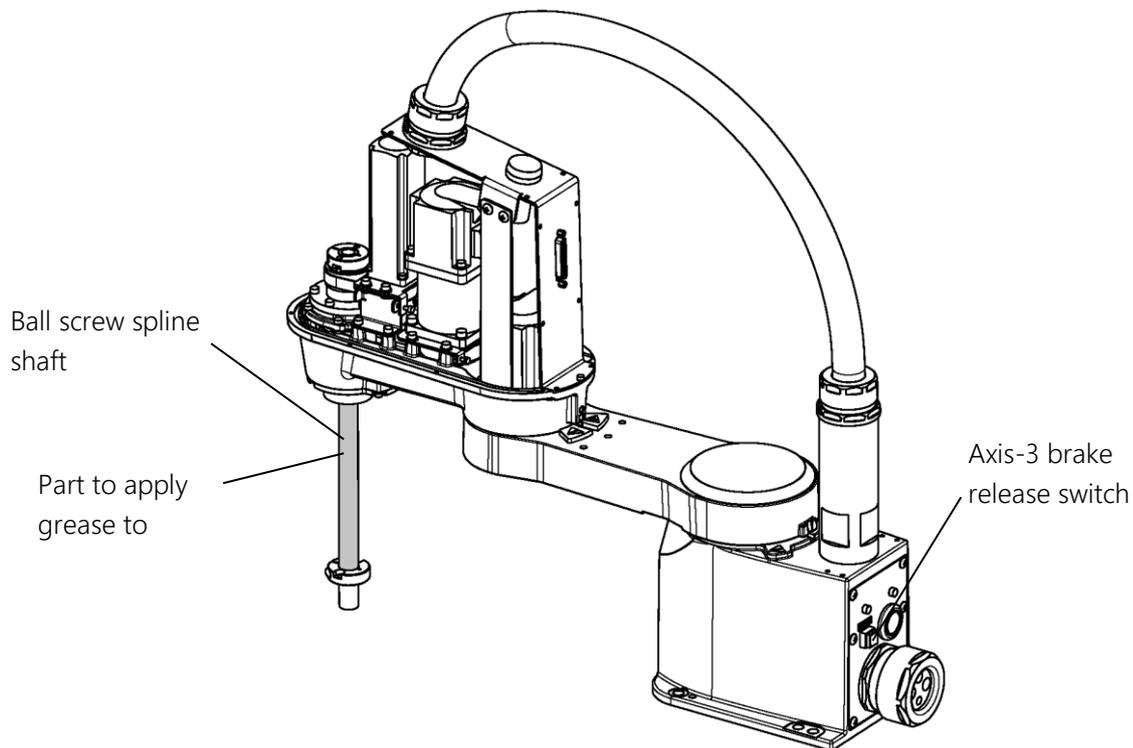
Fig. 7.37 Greasing up the lower side of the ball screw spline unit
