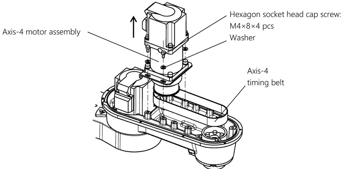
Fig. 7.31 Removing the axis-4 belt and motor assembly
