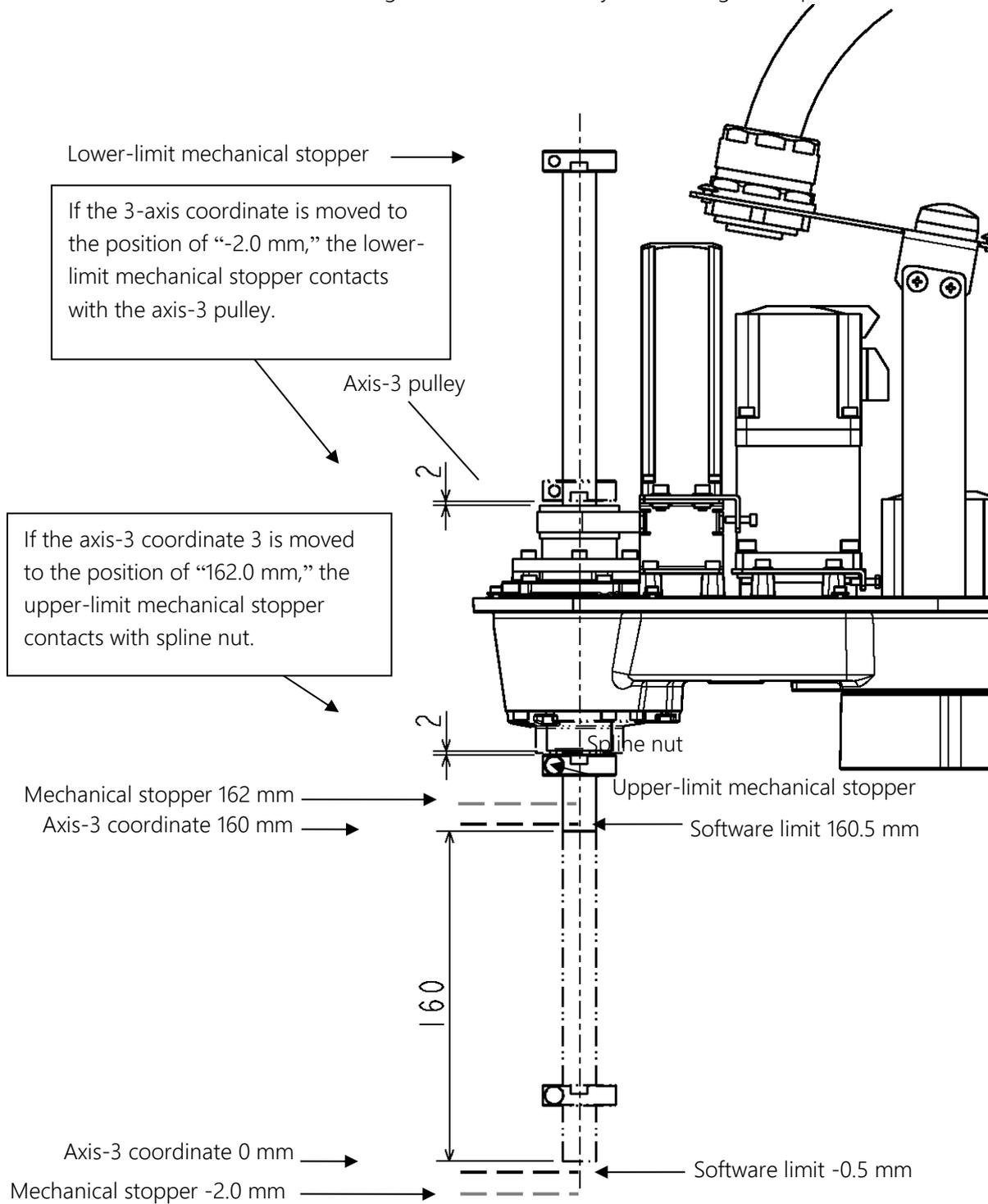
Fig. 3.7 Factory-set axis-3 working envelope
