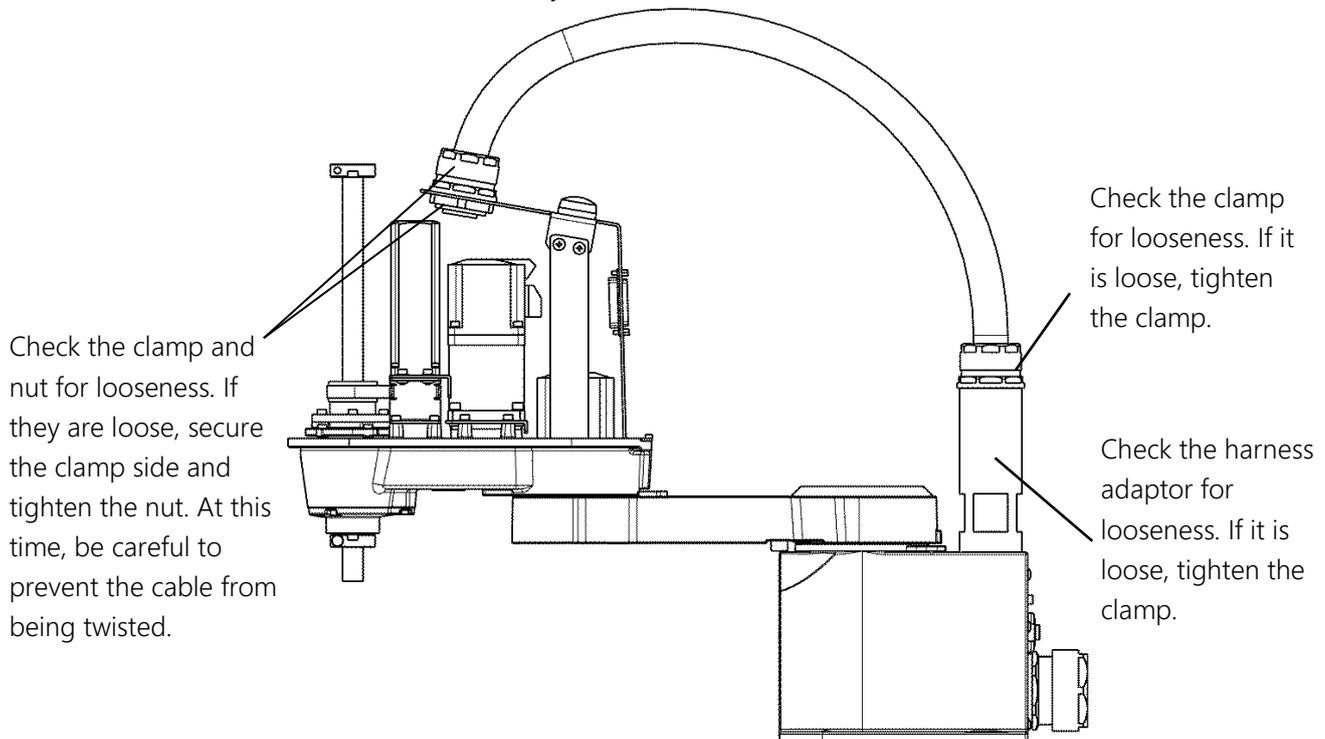
Fig. 7.4 Inspection spot of cable clamp
