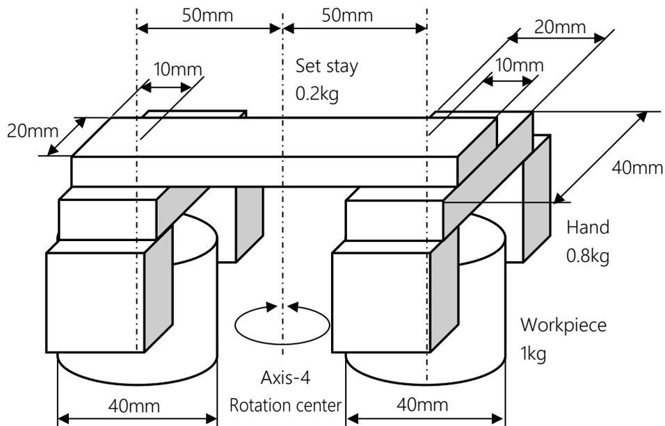
Fig. 4.9 Example of calculating the moment of inertia 2
