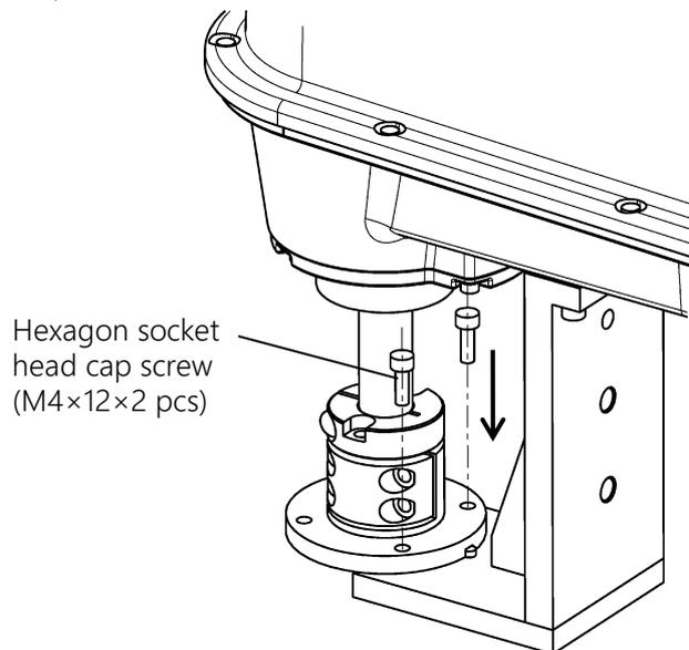
Fig. 8.11 Securing the Tool Flange
