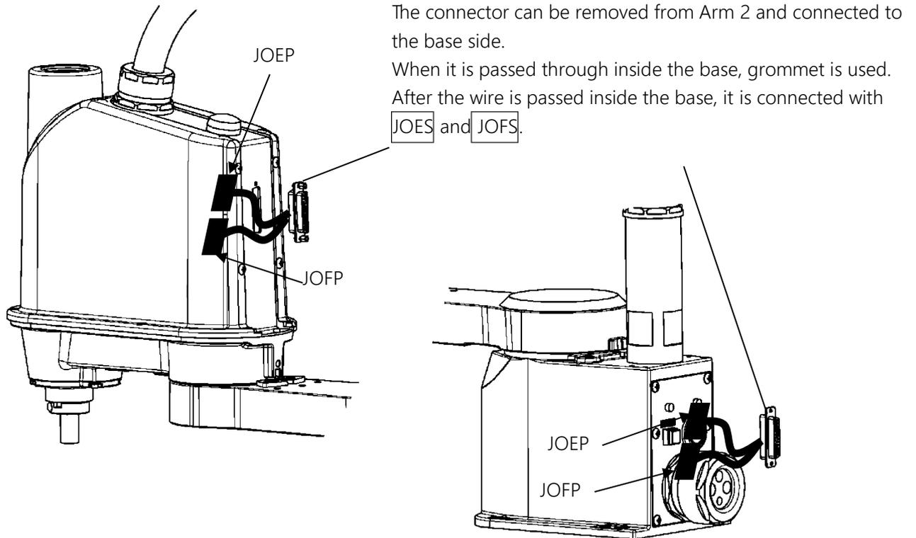
Fig. 5.2 Moving CN0 connector
