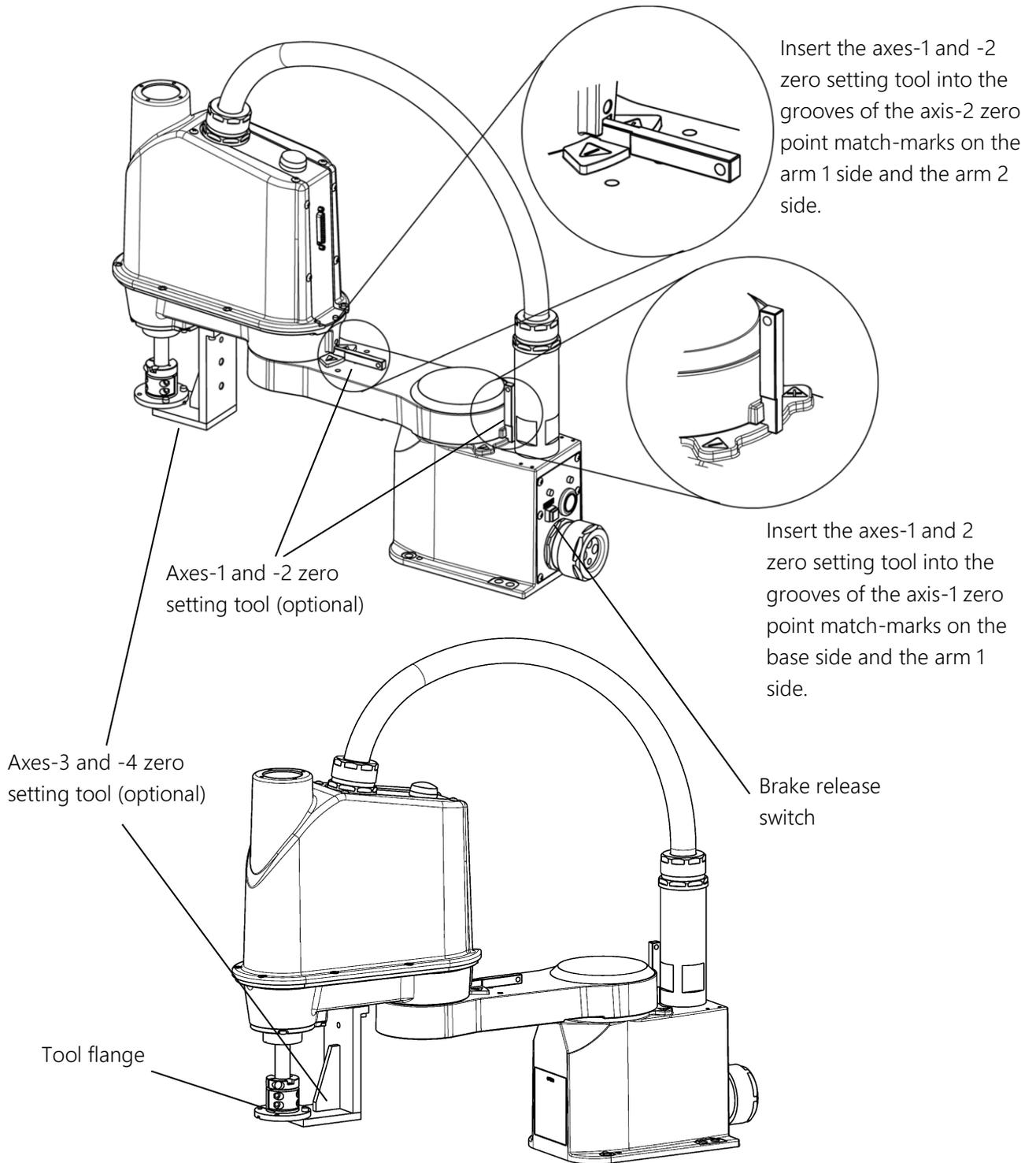
Fig. 8.7 Installing the Zero Setting Tool (Optional)
