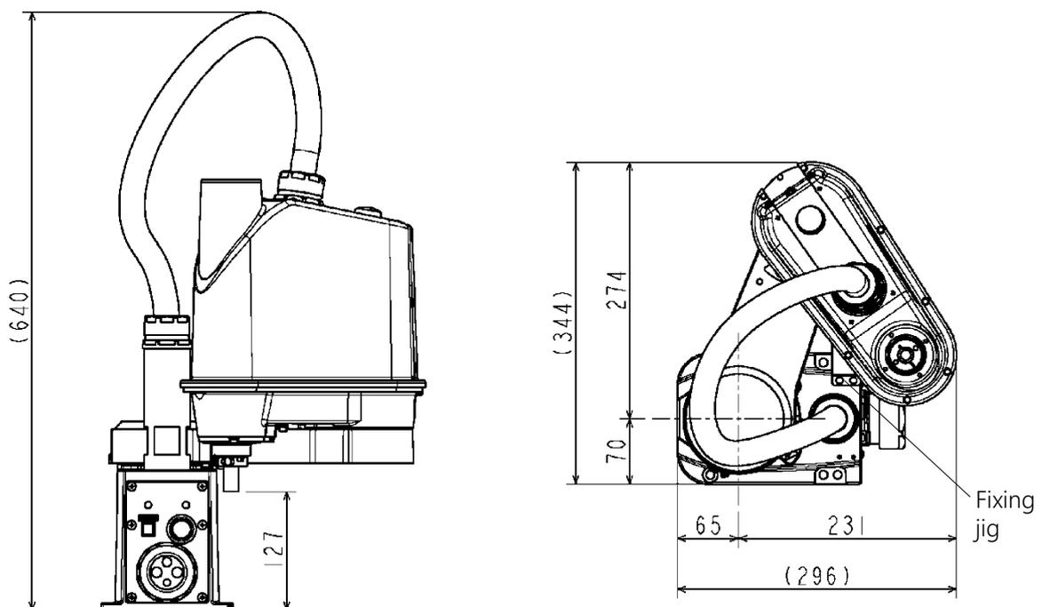
Fig. 2.2 Outer dimensions at transport (KHE-400)
