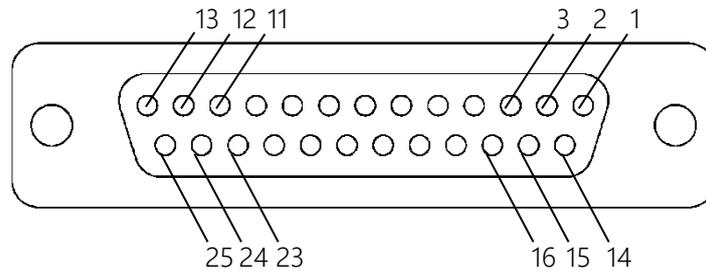
Fig. 5.4 Hand connector pin arrangement
