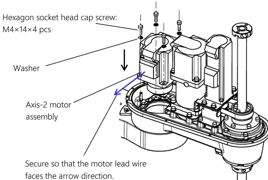
Fig. 7.17 Fitting the axis-2 motor assembly
