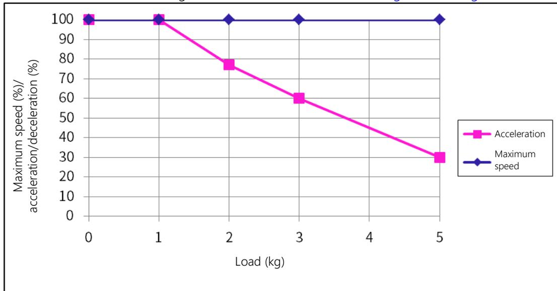
Setting of maximum speed and acceleration/deceleration in relation to load mass (Axis 1)
