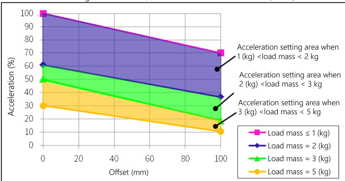
Setting of acceleration/deceleration in relation to offset (Axis 4)
