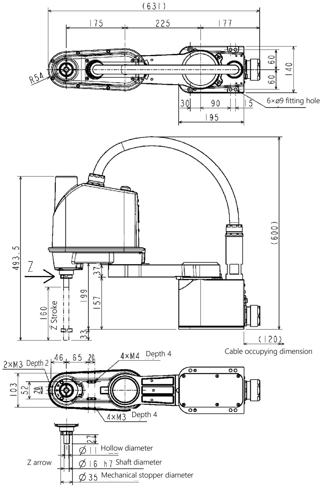
Fig. 1.3 External dimensions of the robot (KHE-400)
