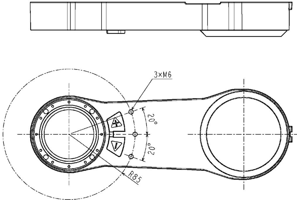
Fig. 3.4 Mounting position of axis-2 mechanical stopper
