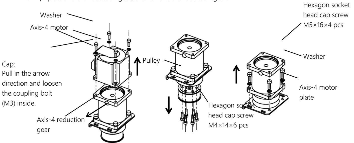
Fig. 7.55 Removing the axis-4 reduction gear
