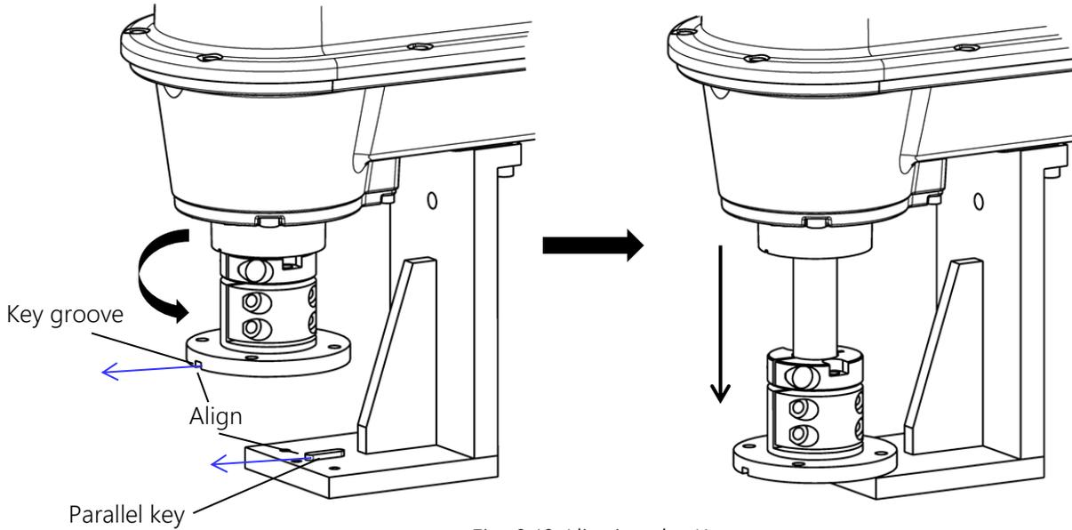
Fig. 8.10 Aligning the Key
