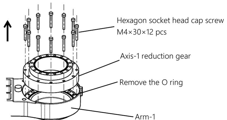
Fig. 7.46 Removing the axis-1 reduction gear
