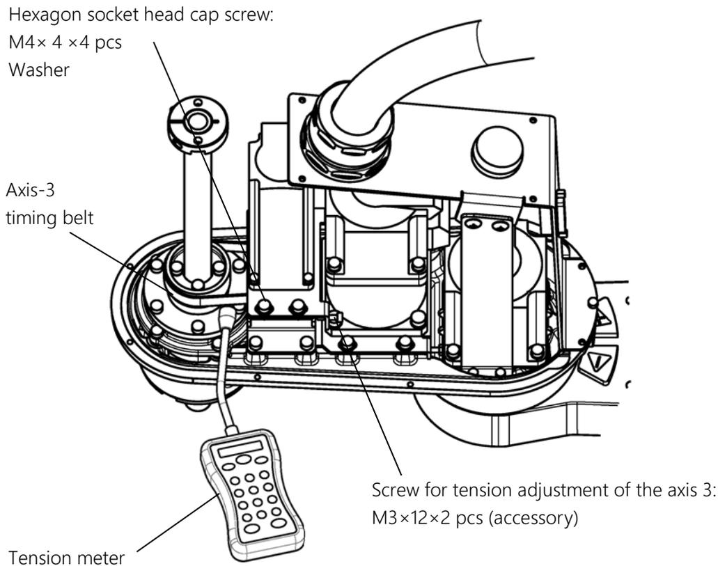
Fig. 7.29 Adjusting the tension of the axis 3
