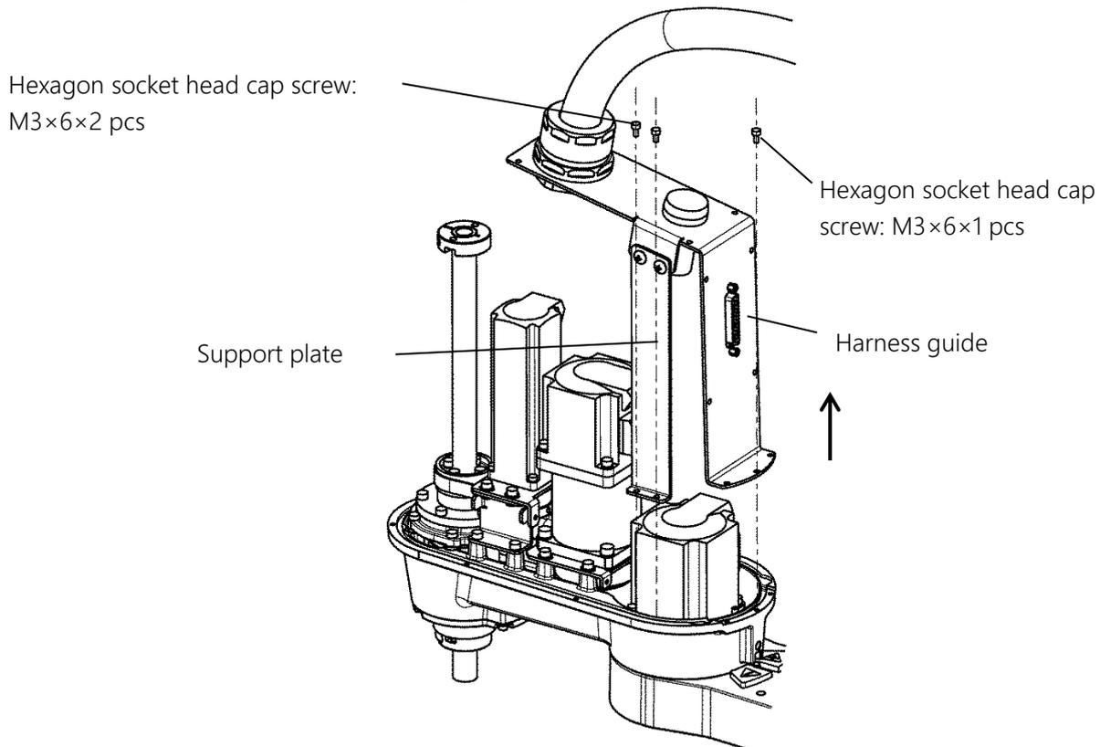
Fig. 7.15 Removing harness guide and support plate
