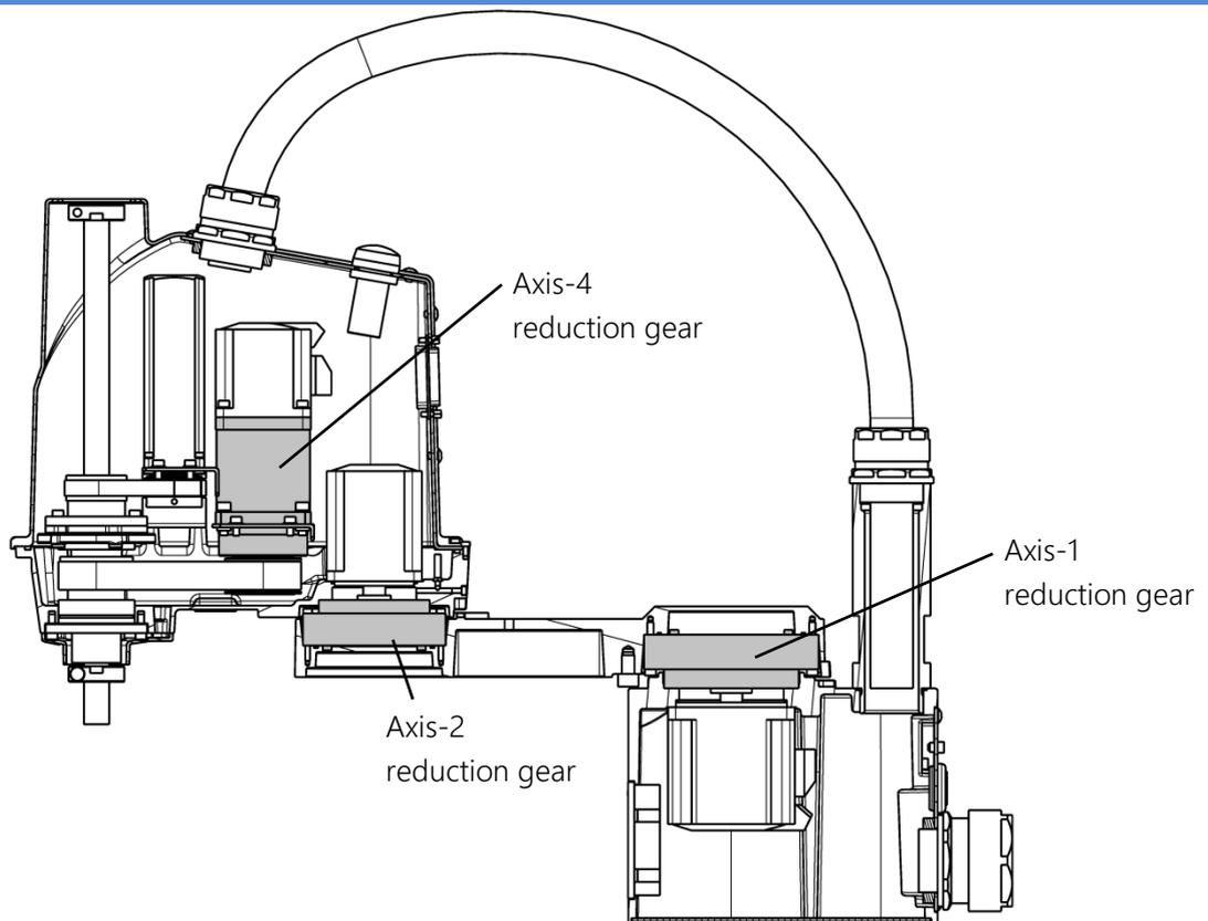
Fig. 7.44 Locations of reduction gears
