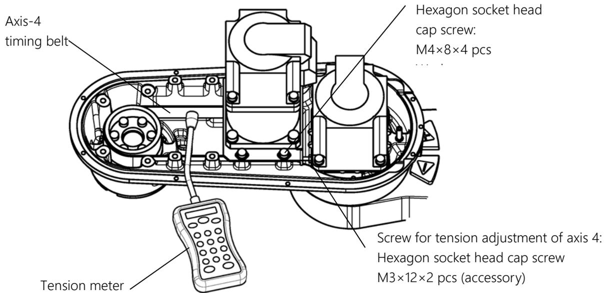
Fig. 7.57 Adjusting the tension of the axis-4 timing belt
