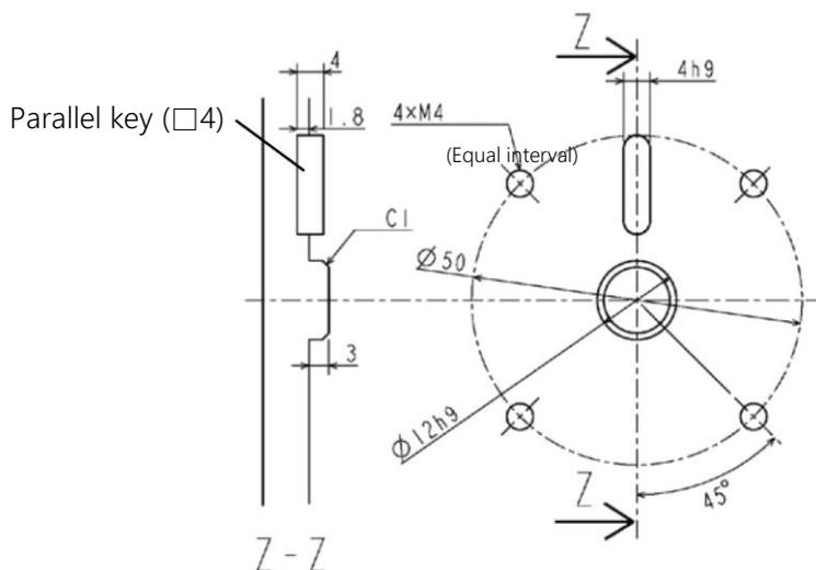
Fig. 8.2 Example of Shape of Securing the Tool Flange (Optional)
