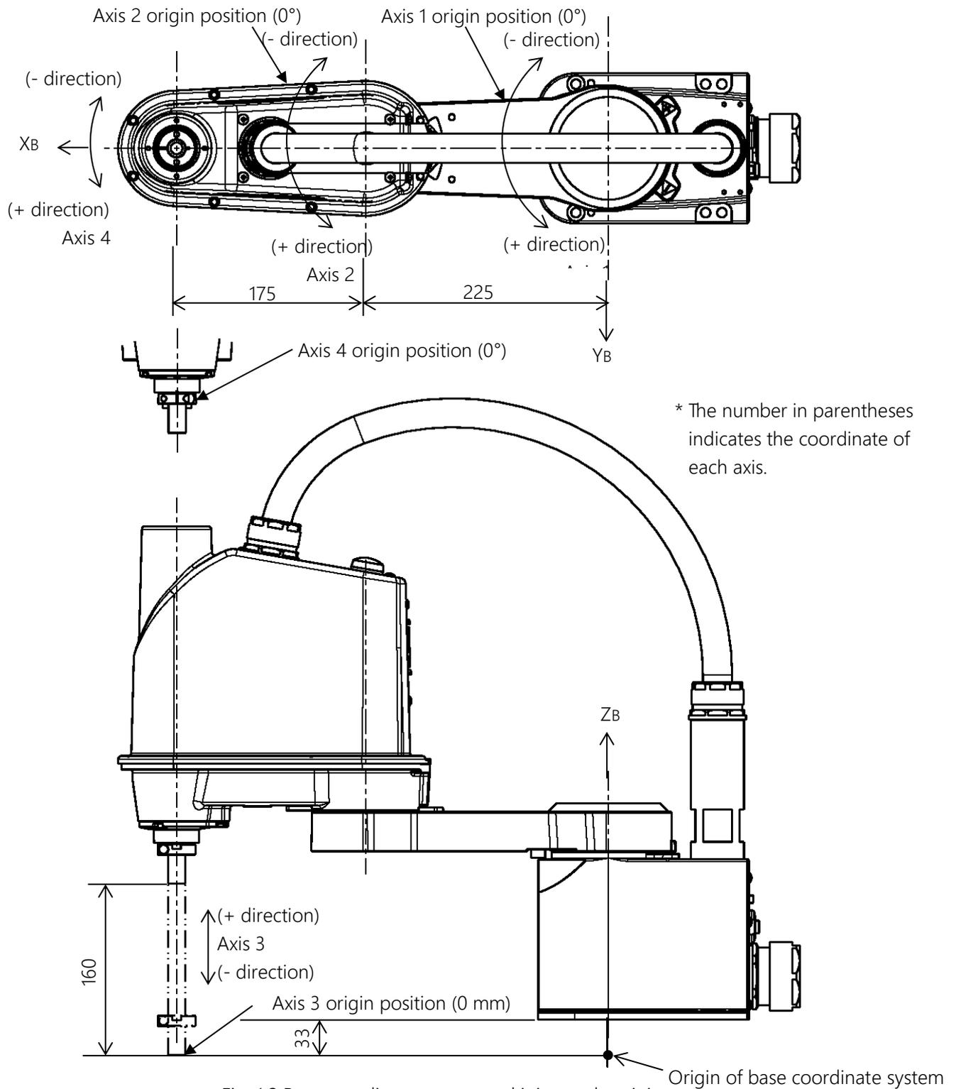
Fig. 1.2 Base coordinate system and joint angle origin
