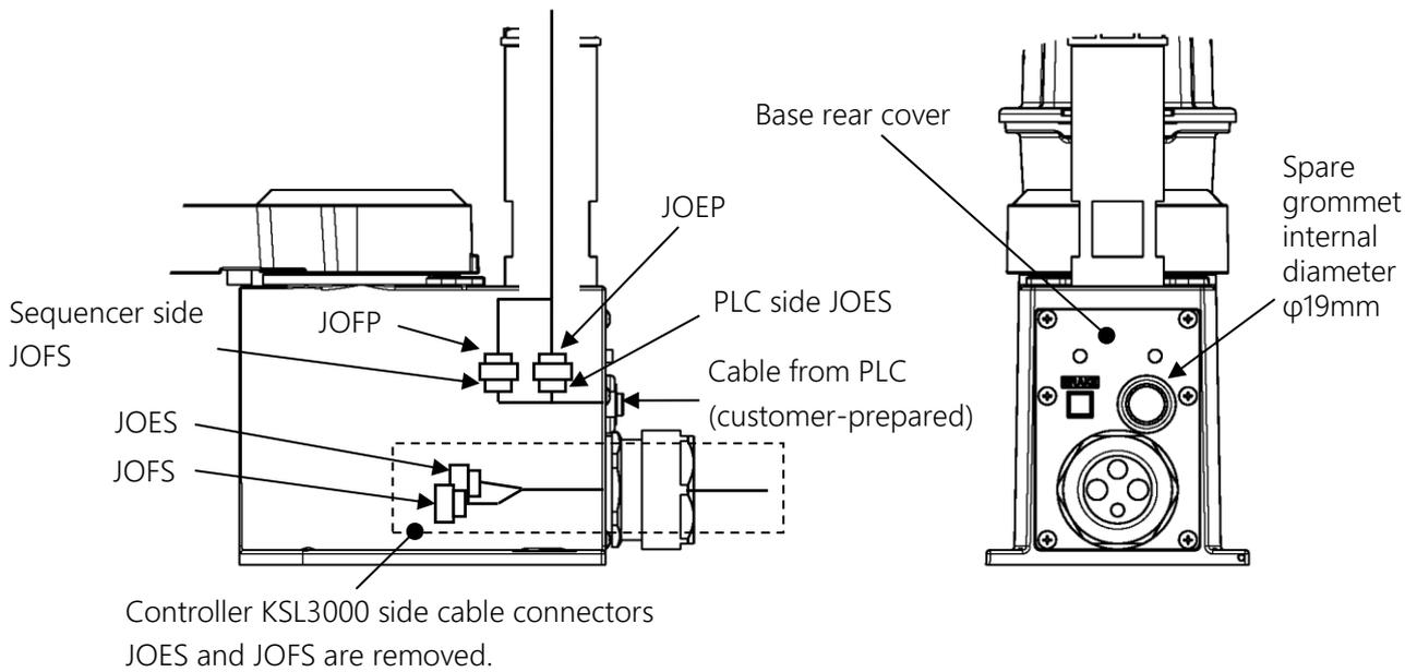
Fig. 5.3 Wiring to PLC
