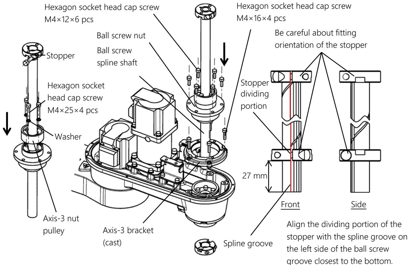
Fig. 7.43 Fitting the ball screw spline unit
