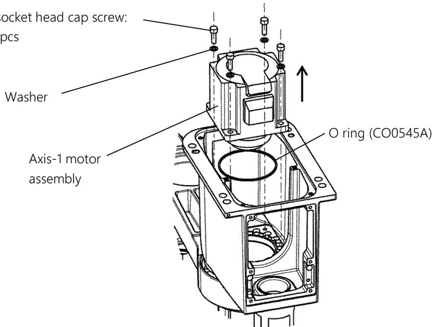
Fig. 7.10 Removing axis-1 motor assembly
