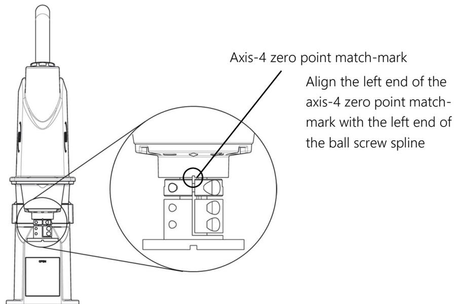
Fig. 8.7 Check Work (Axis 4)
