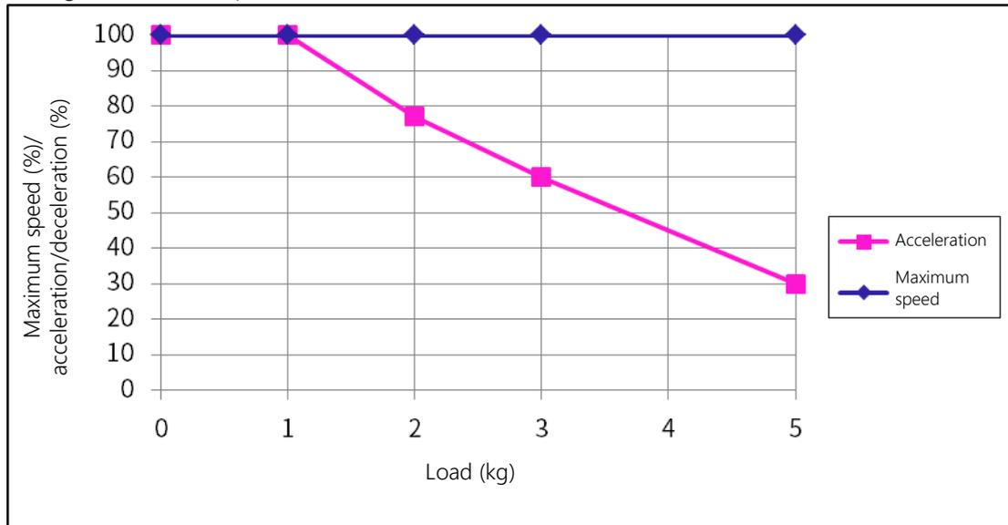
Setting of maximum speed and acceleration/deceleration in relation to load mass (Axis 2)
