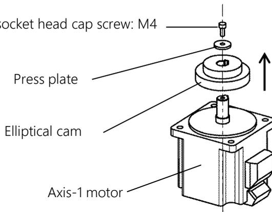
Fig. 7.11 Removing the axis-1 elliptical cam
