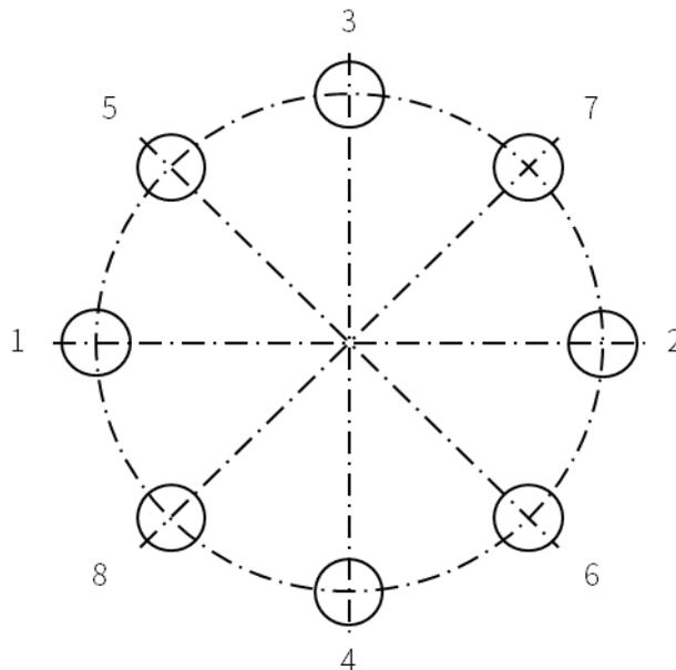
Fig. 6.2 Clamping bolts on a circle
