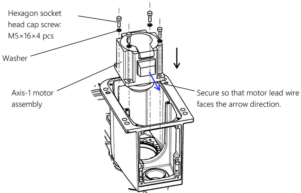
Fig. 7.14 Fitting axis-1 motor assembly
