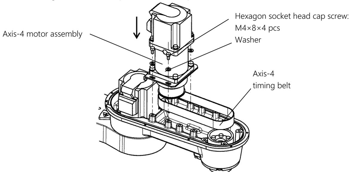
Fig. 7.32 Fitting the axis-4 motor assembly
