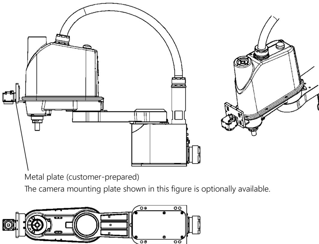
Fig. 4.3 Example of mounting the camera
