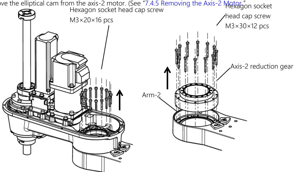
Fig. 7.50 Removing the axis-2 reduction gear
