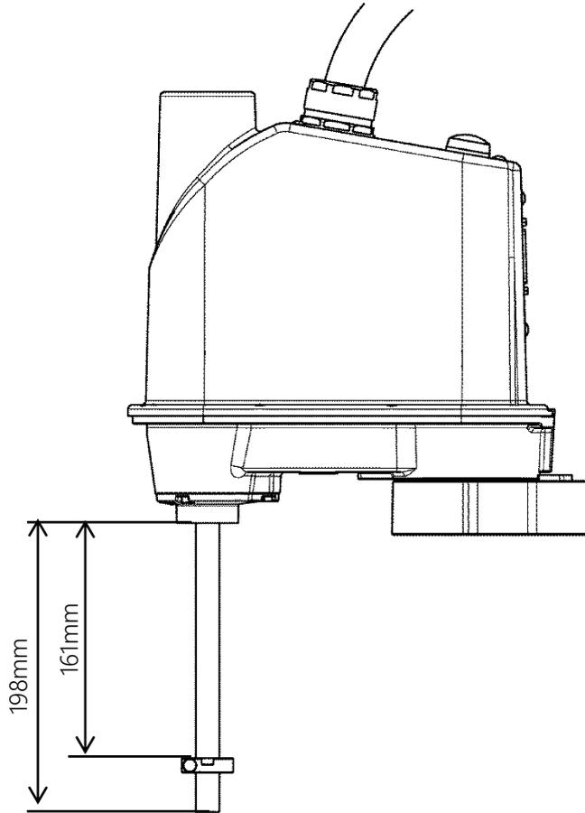
Fig. 8.6 Dimensions of the Axis-3 Zero Point
