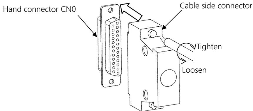
Fig. 5.5 Connecting/disconnecting hand input/output signal connector
