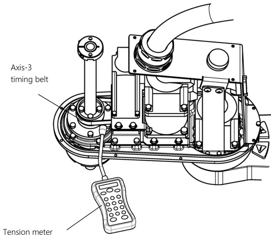
Fig. 7.19 Measuring the Tension of the Axis-3 Timing Belt
