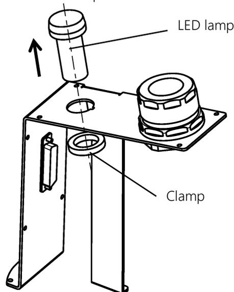
Fig. 7.60 Removing the LED Lamp
