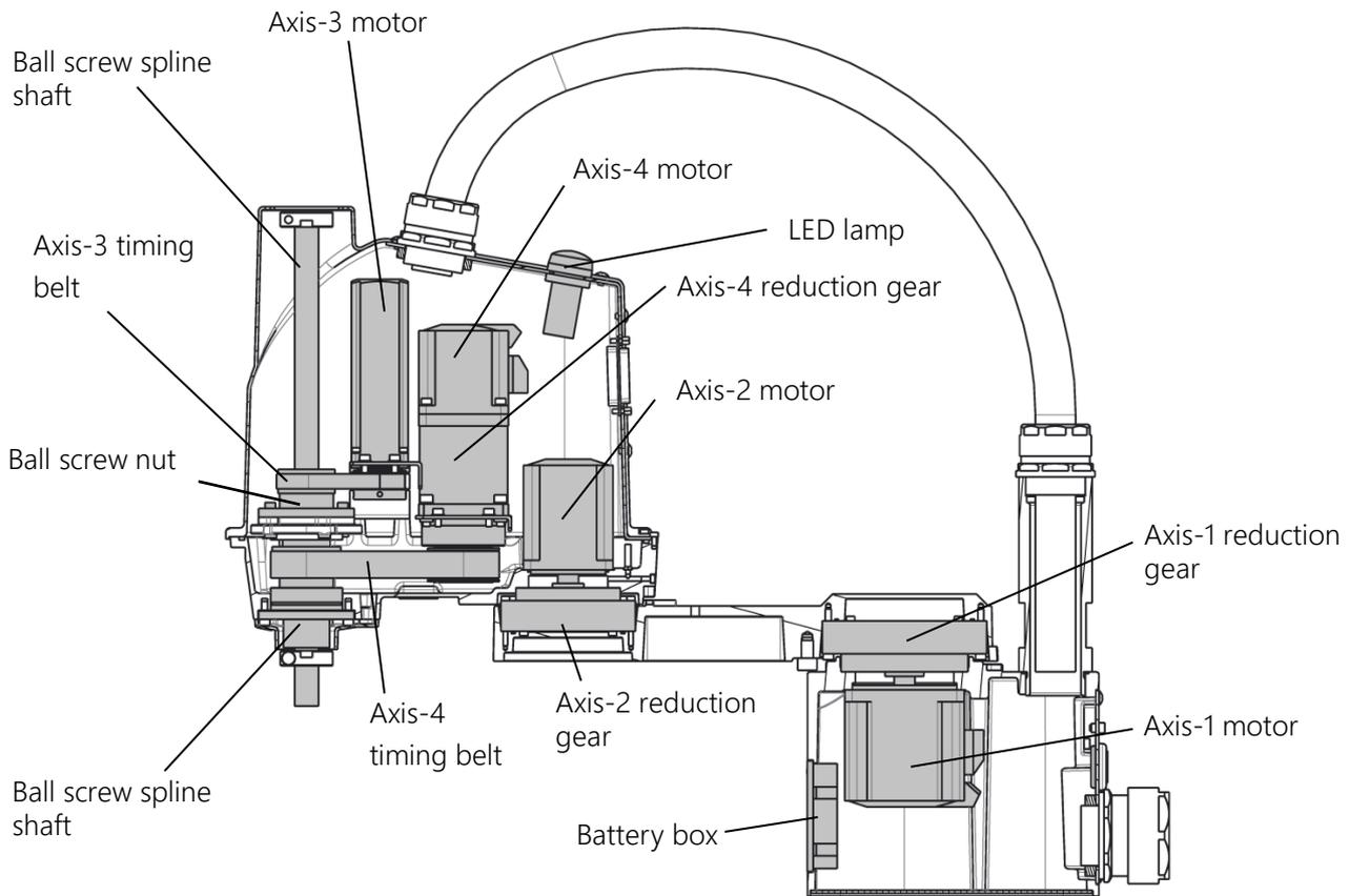
Fig. 7.5 Configuration of mechanical components
