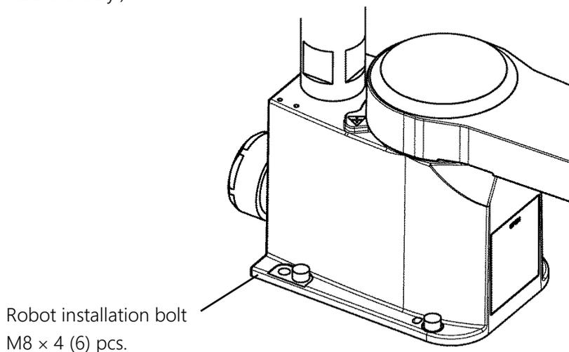
Fig. 7.2 Robot installation bolts
