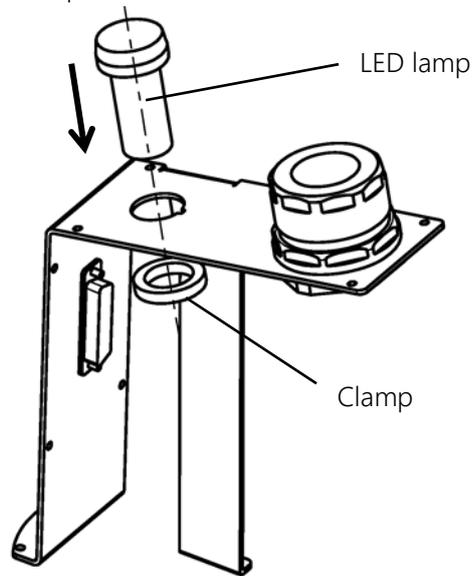
Fig. 7.61 Fitting the LED Lamp
