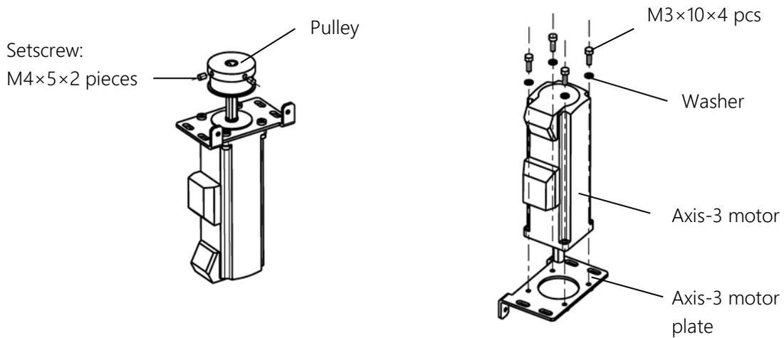
Fig. 7.21 Removing the axis-3 pulley and plate
