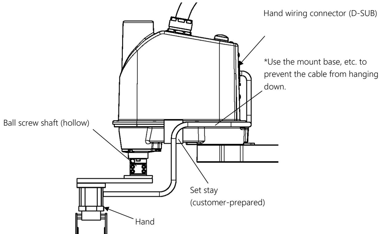
Fig. 5.10 Example of hand cable wiring from arm 2 rear
