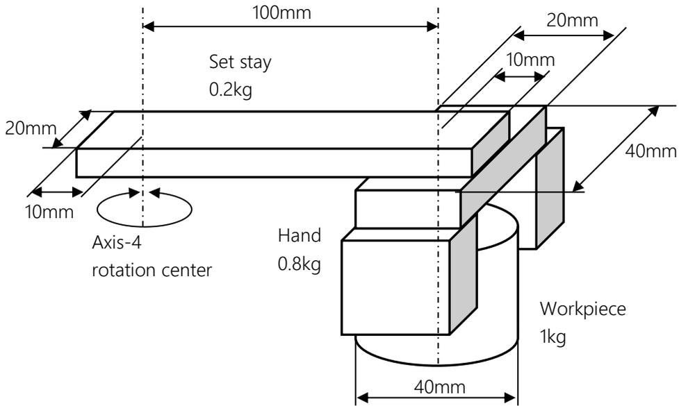
Fig. 4.8 Example of calculating the moment of inertia 1
