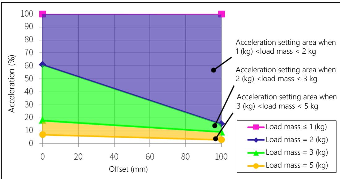
Setting of acceleration/deceleration in relation to offset (Axis 3)
