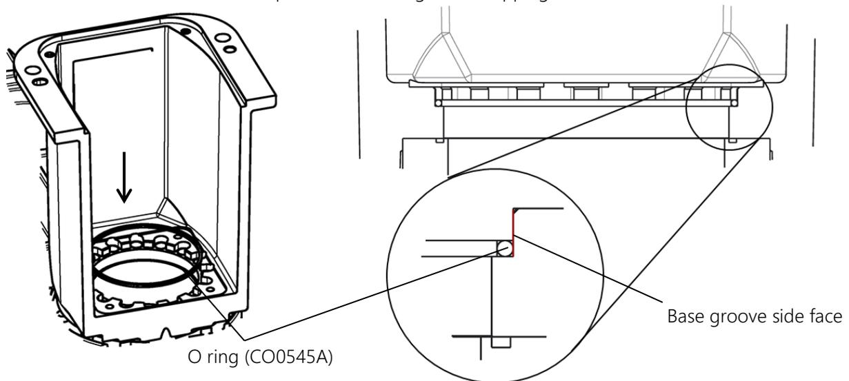
Fig. 7.13 Fitting O ring on axis-1 base side
