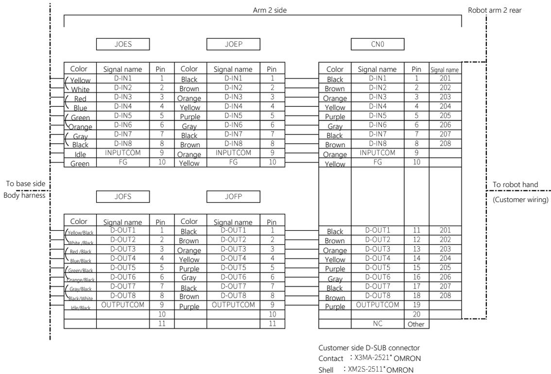
Fig. 5.7 Hand wiring diagram Arm 2 side (common to Type-N, P KSL3000)
