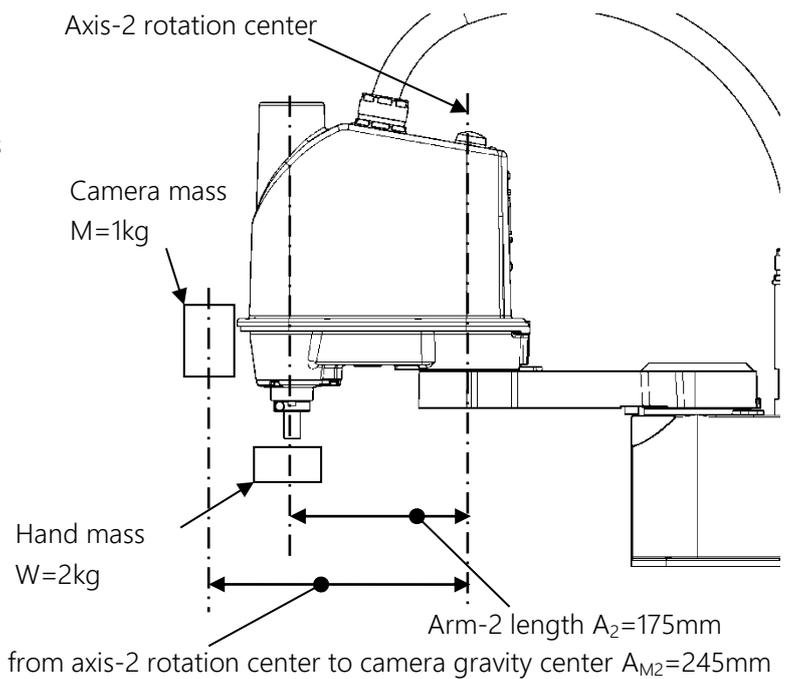
Fig. 4.6 Mounting on the tip from axis-3 center
