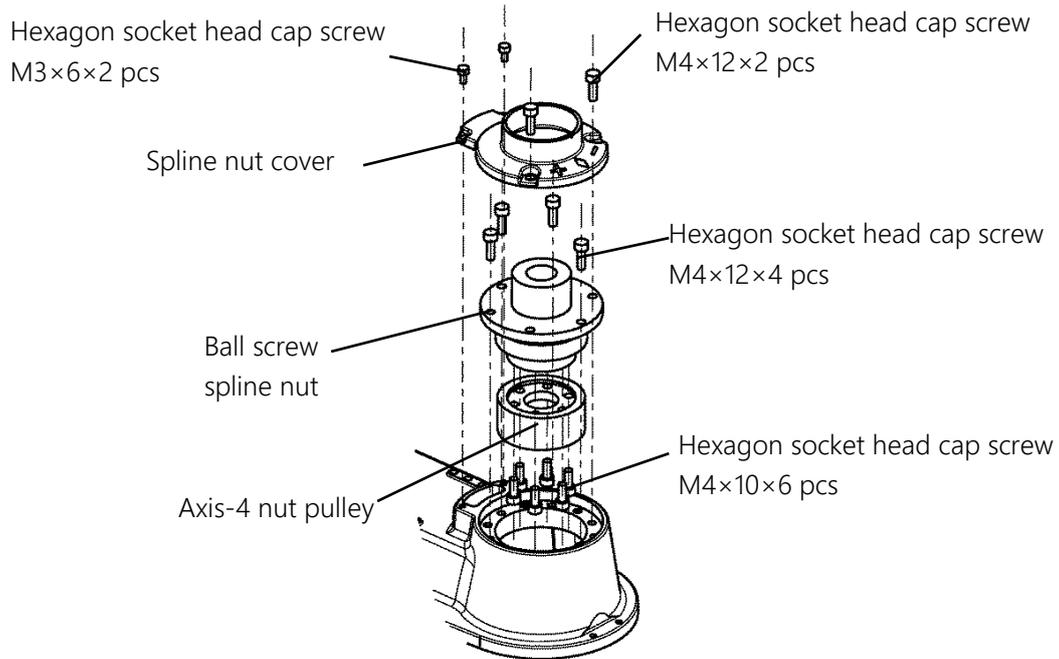
Fig. 7.40 Removing the ball screw spline nut
