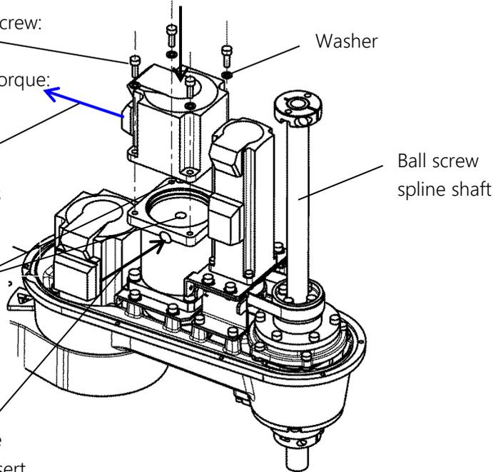
Fig. 7.26 Fitting the axis-4 motor
