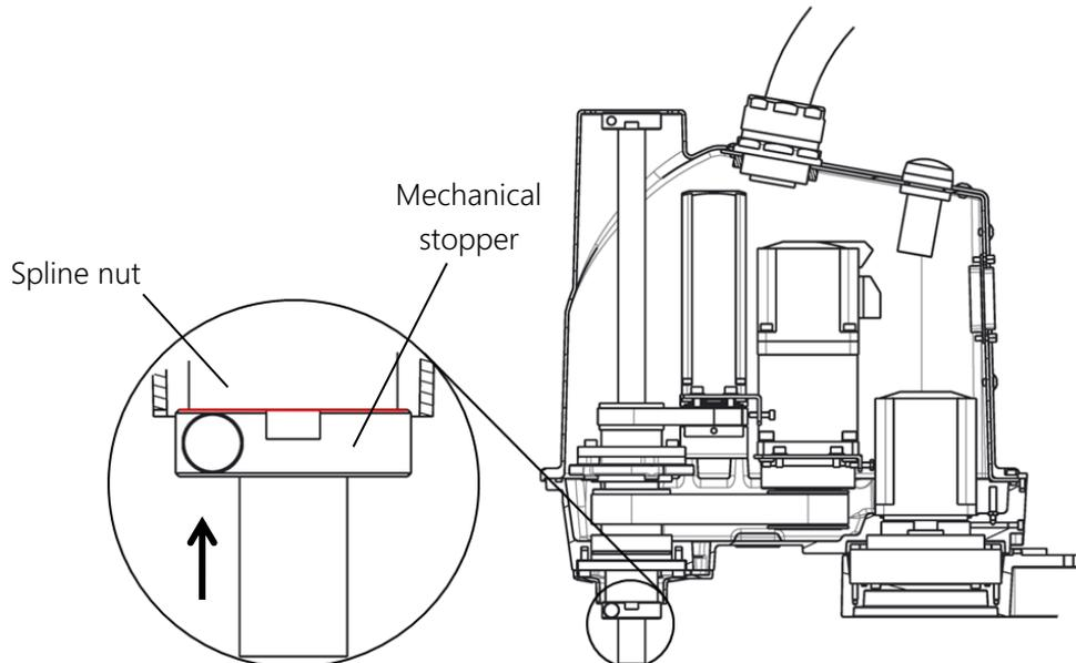
Fig. 8.4 Work to Bring the Mechanical Stopper into Contact with the Axis 3 (HOME3)
