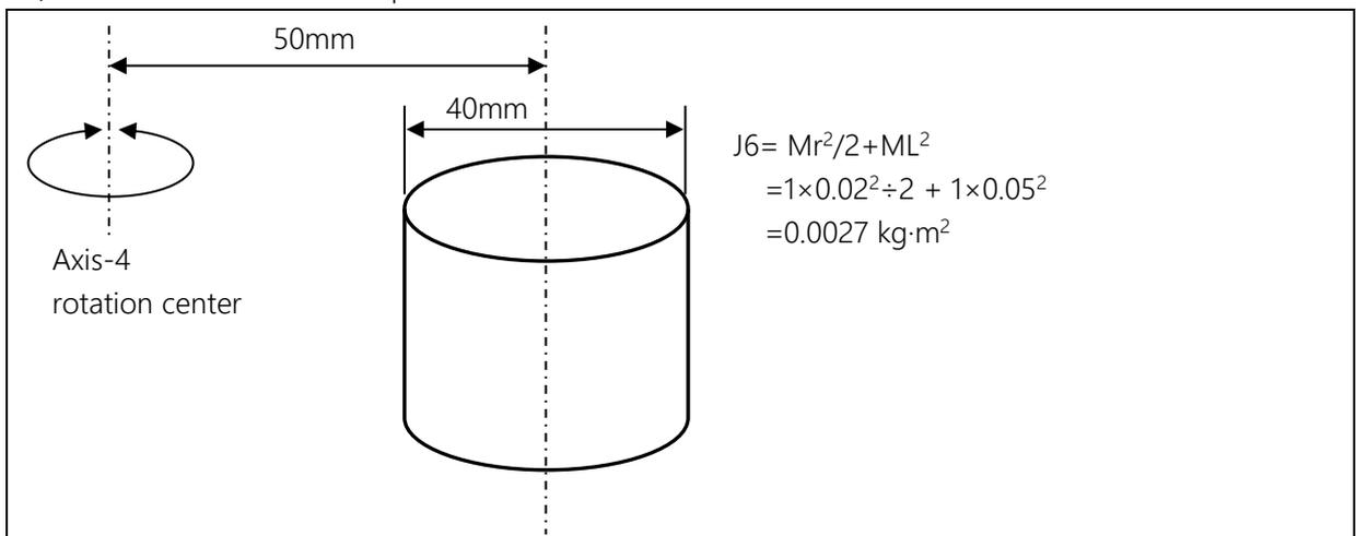
The entire moment of inertia is the sum of  $J4 + J5 \times 2 + J6 \times 2$  to result in 0.009906 kg·m<sup>2</sup>.
