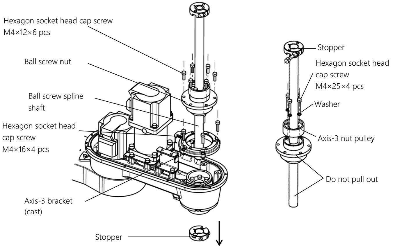
Fig. 7.39 Removing the ball screw spline unit
