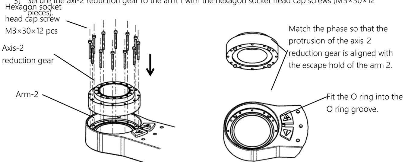
Fig. 7.51 Fitting the Axis-2 Reduction Gear
