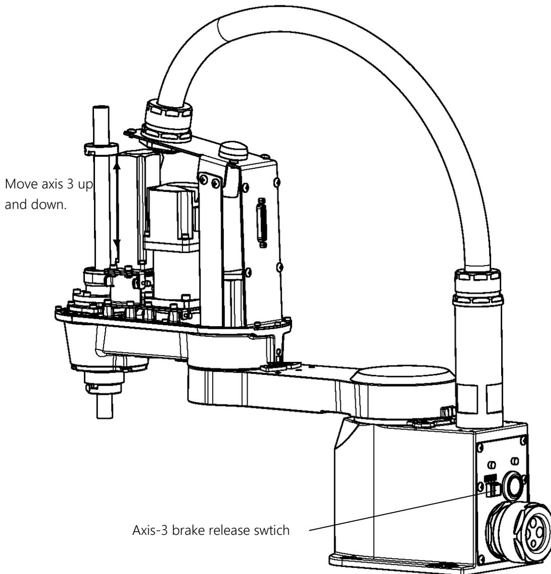
Fig. 3.9 Changing and checking the axis-3 software limit
