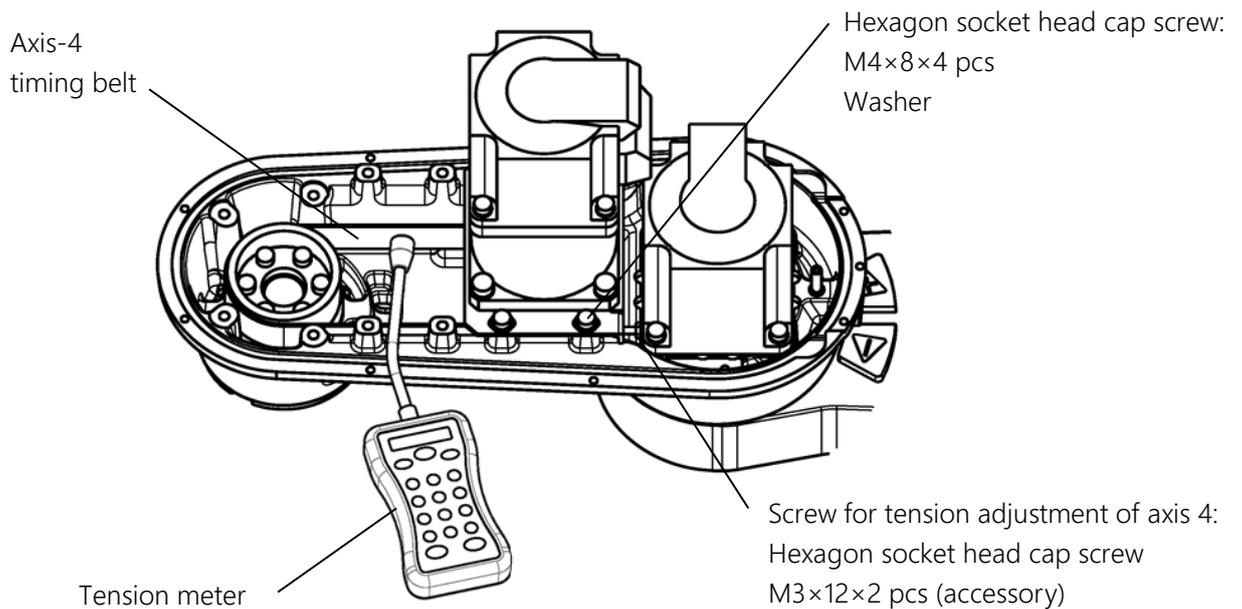
Fig. 7.33 Adjusting the tension of axis 4
