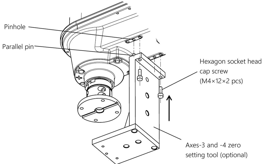
Fig. 8.9 Secure the Axes-3 and -4 Zero Setting Tool
