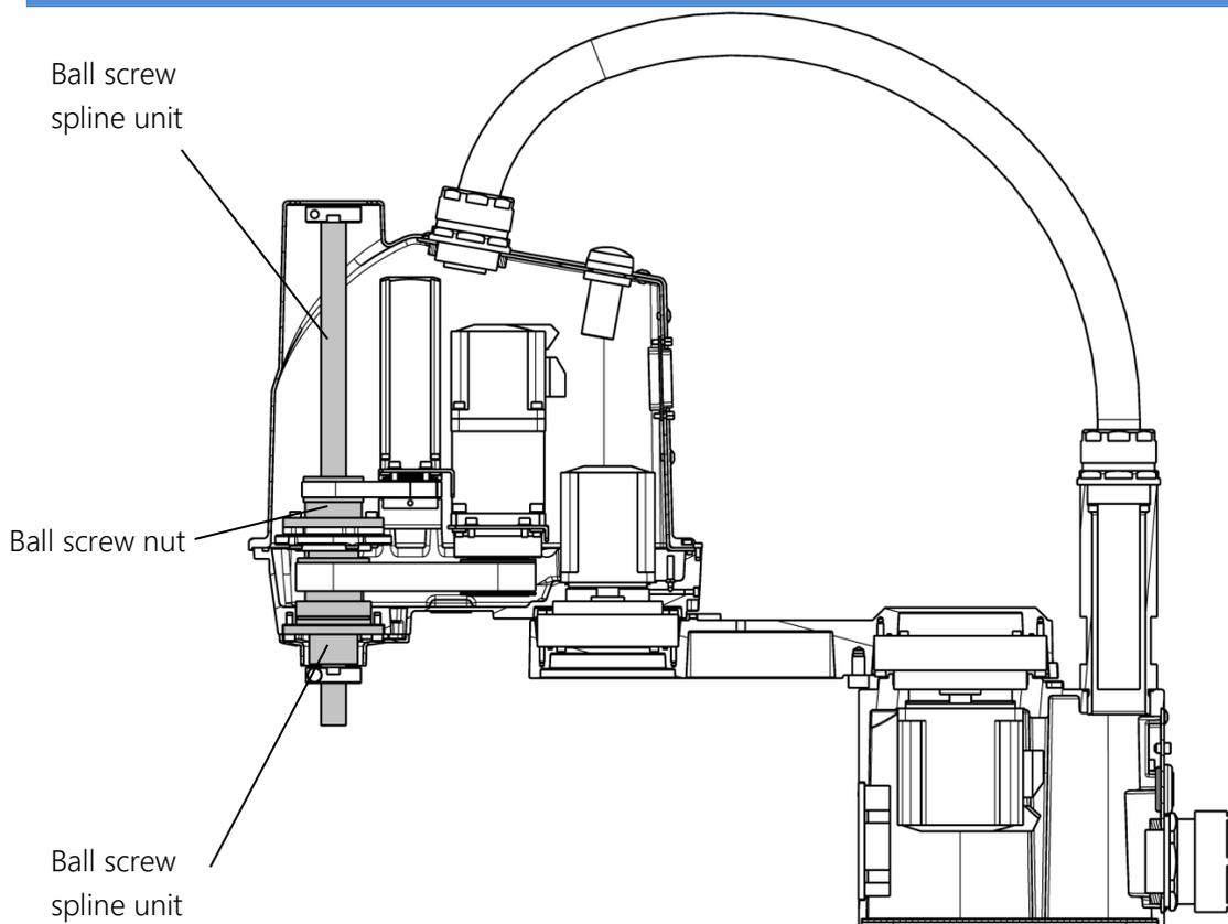
Fig. 7.35 Location of the ball screw spline unit
