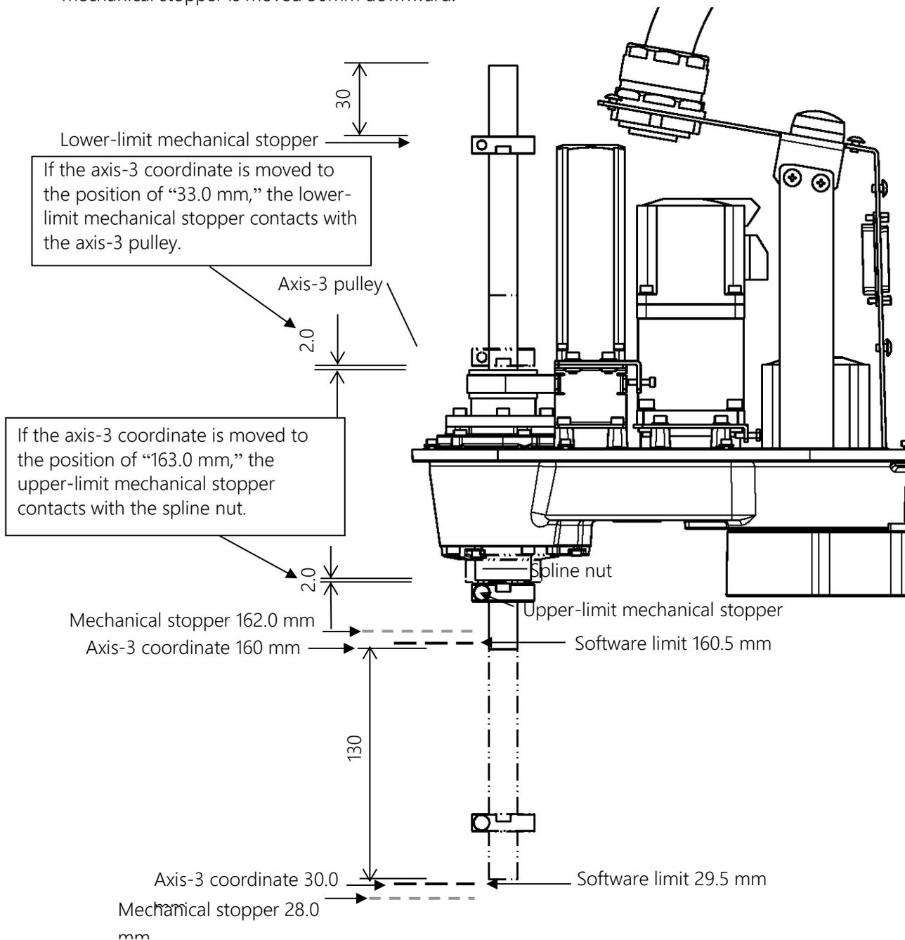
Fig. 3.10 Example of changing axis-3 working envelope
