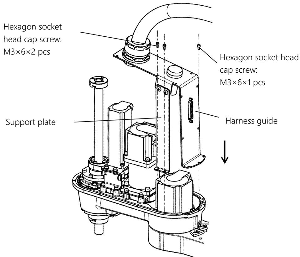
Fig. 7.18 Fitting harness guide and support plate
