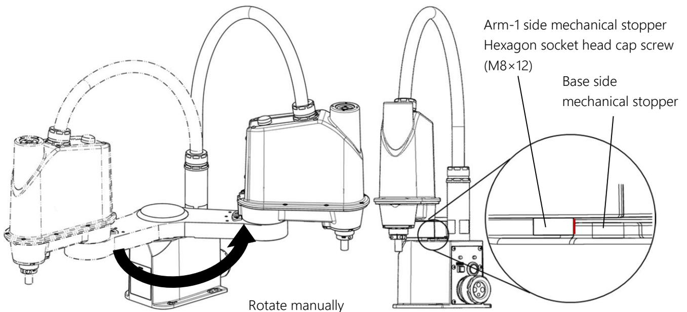
Fig. 8.3 Work to Bring the Mechanical Stopper into Contact with the Axis 1 (HOME3)
