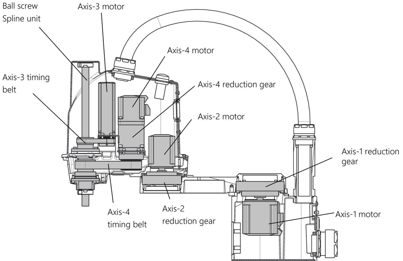
Fig. 8.2 Replacement Parts that Require ② ZEROP Operation Using the Zero Setting Tool or
