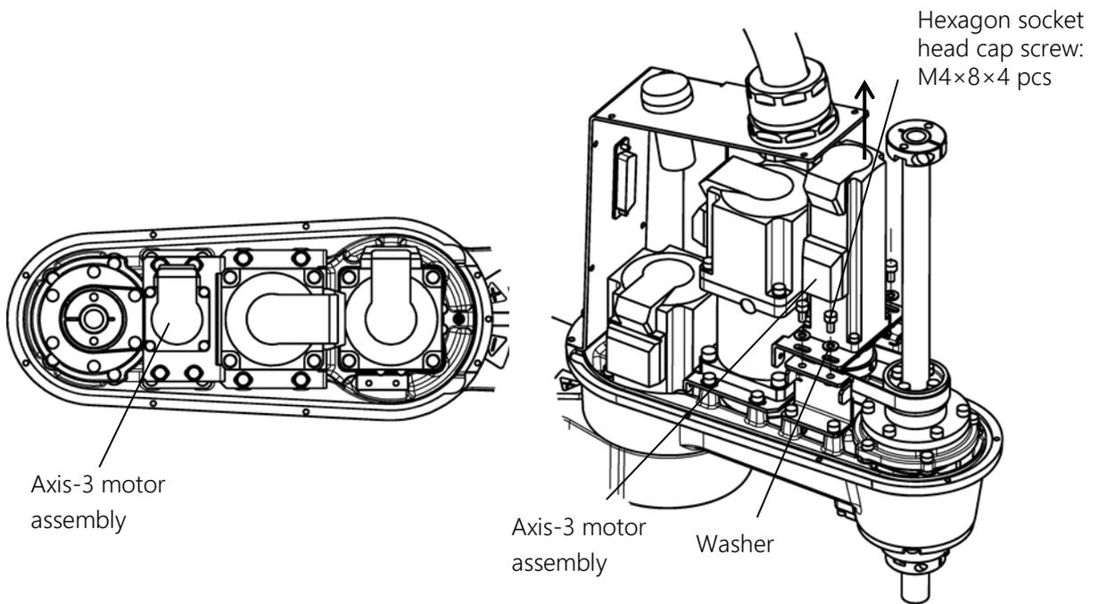
Fig. 7.20 Removing the axis-3 motor assembly
