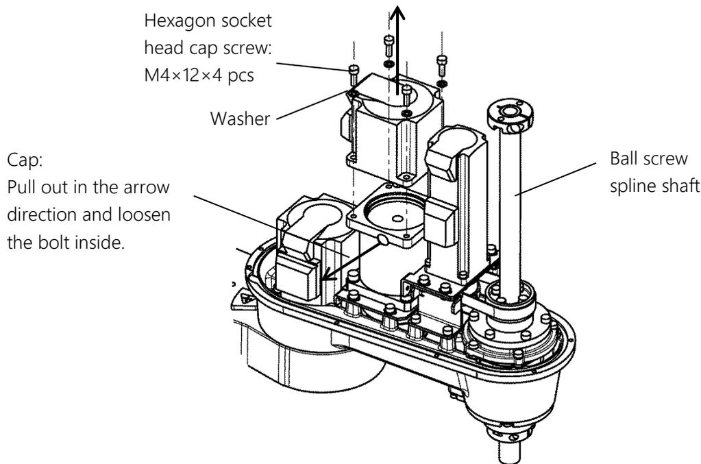
Fig. 7.25 Removing the axis-4 motor
