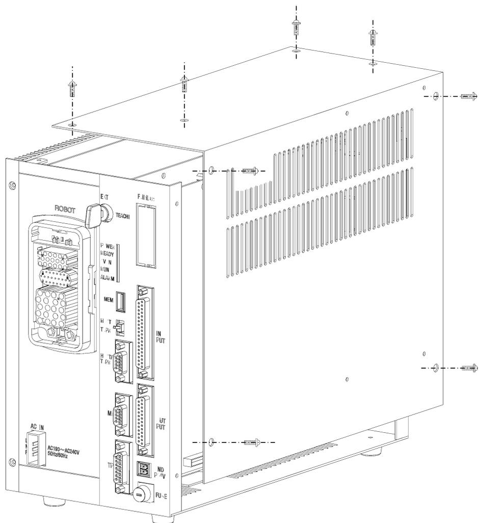
Fig. 7.4 Removing upper cover (KSL3000)
