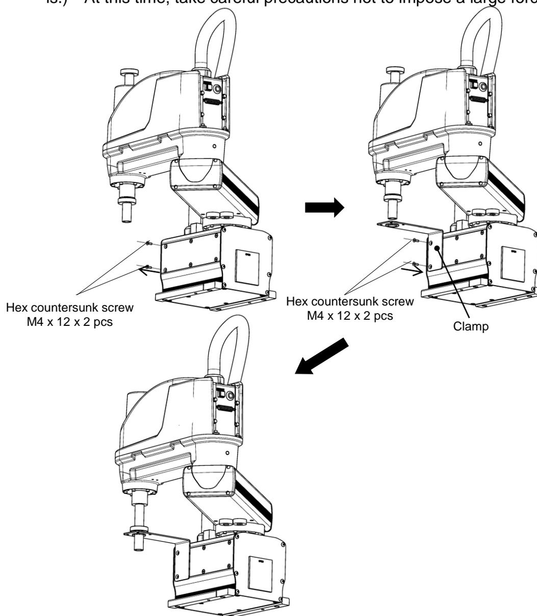
Fig. 4.5 Attaching the clamp (KHL-500/KHL-600/KHL-700)
