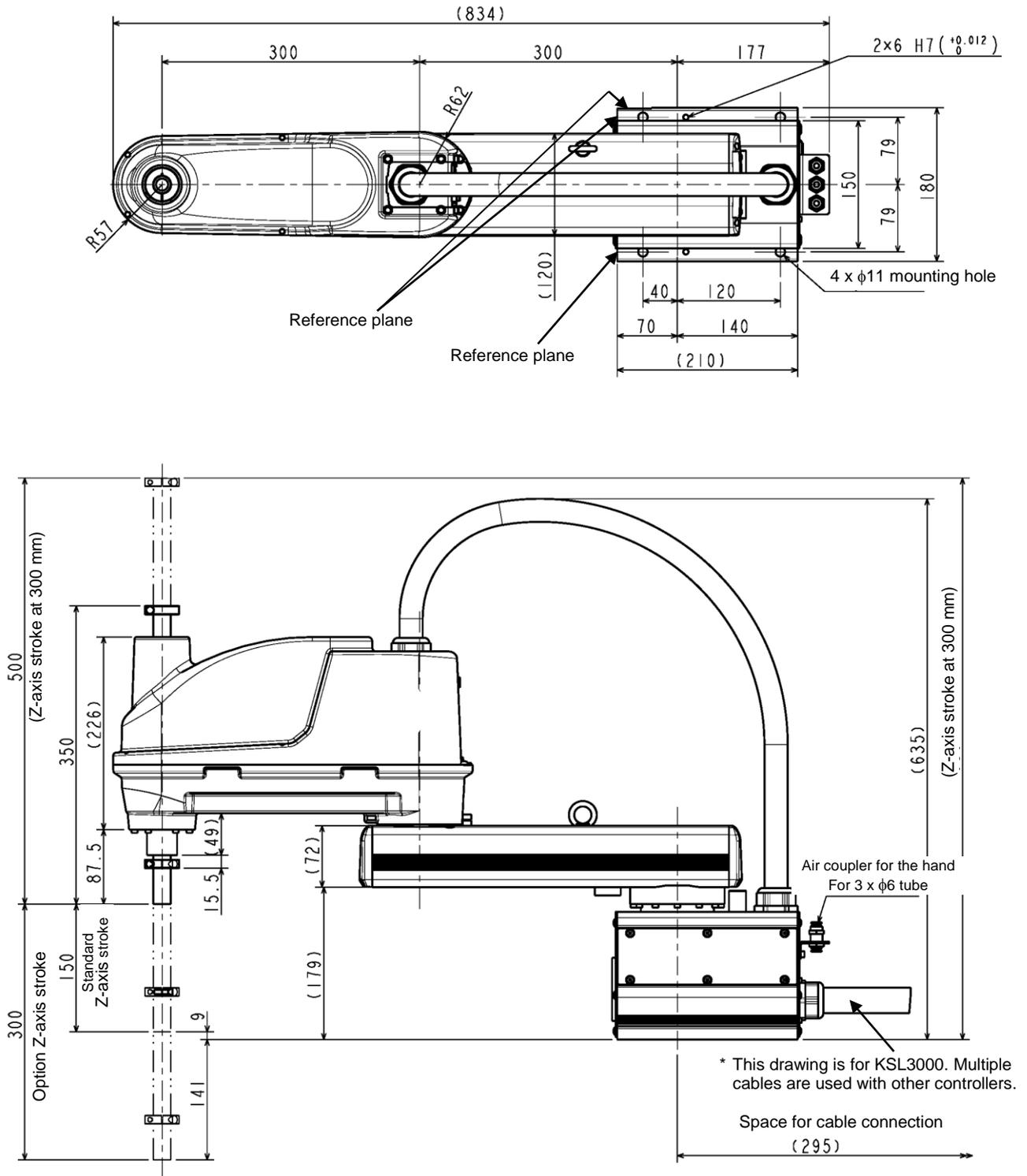
Fig. 2.3 External dimensions of robot (KHL-600)
