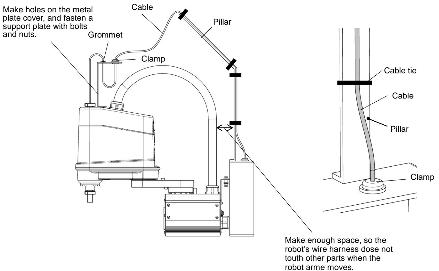
Fig. 11.8 Tool cable wiring installation example (KHL-300/KHL-400)
