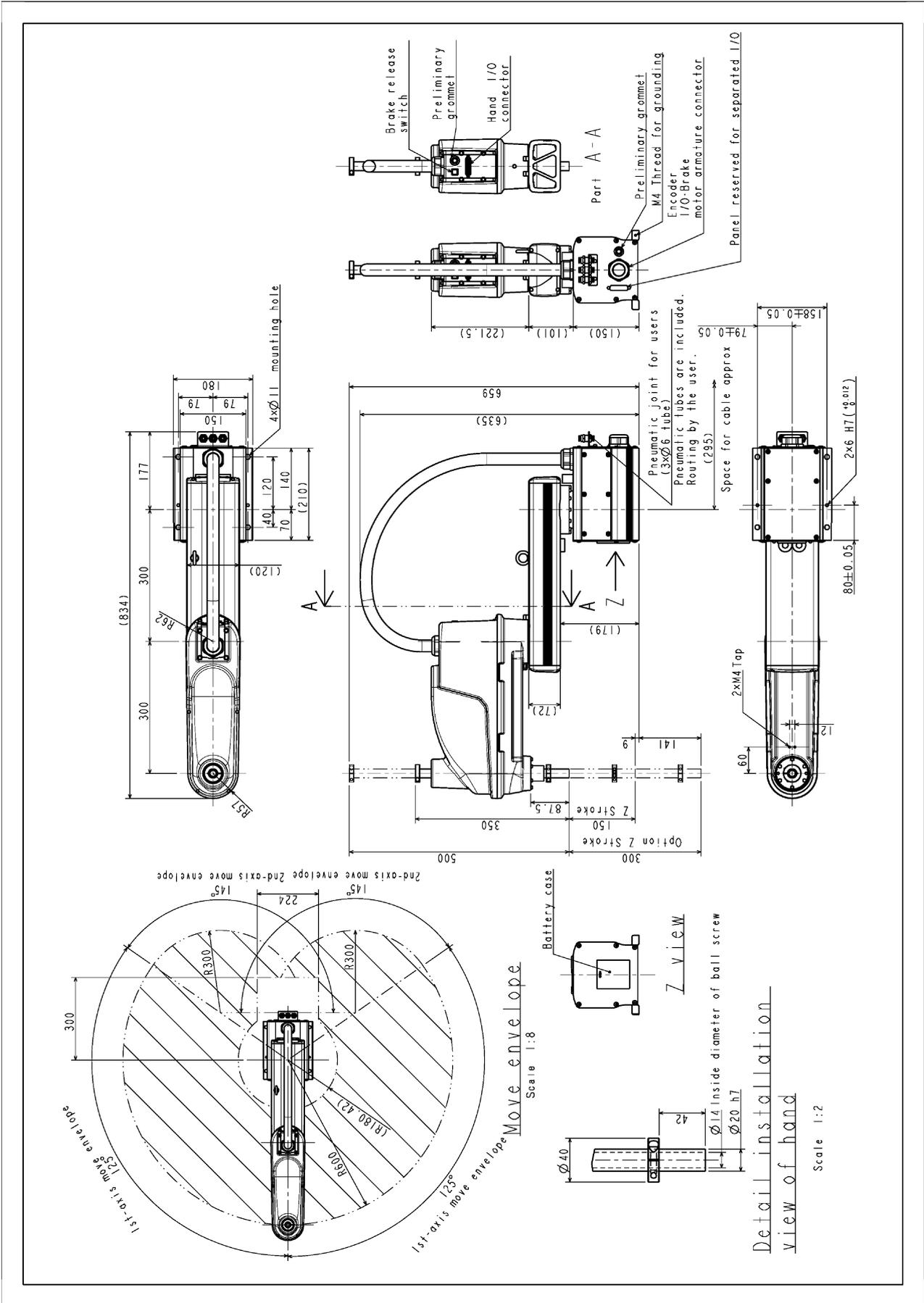
Fig. 6.2 External view and working envelope (KHL-600)
