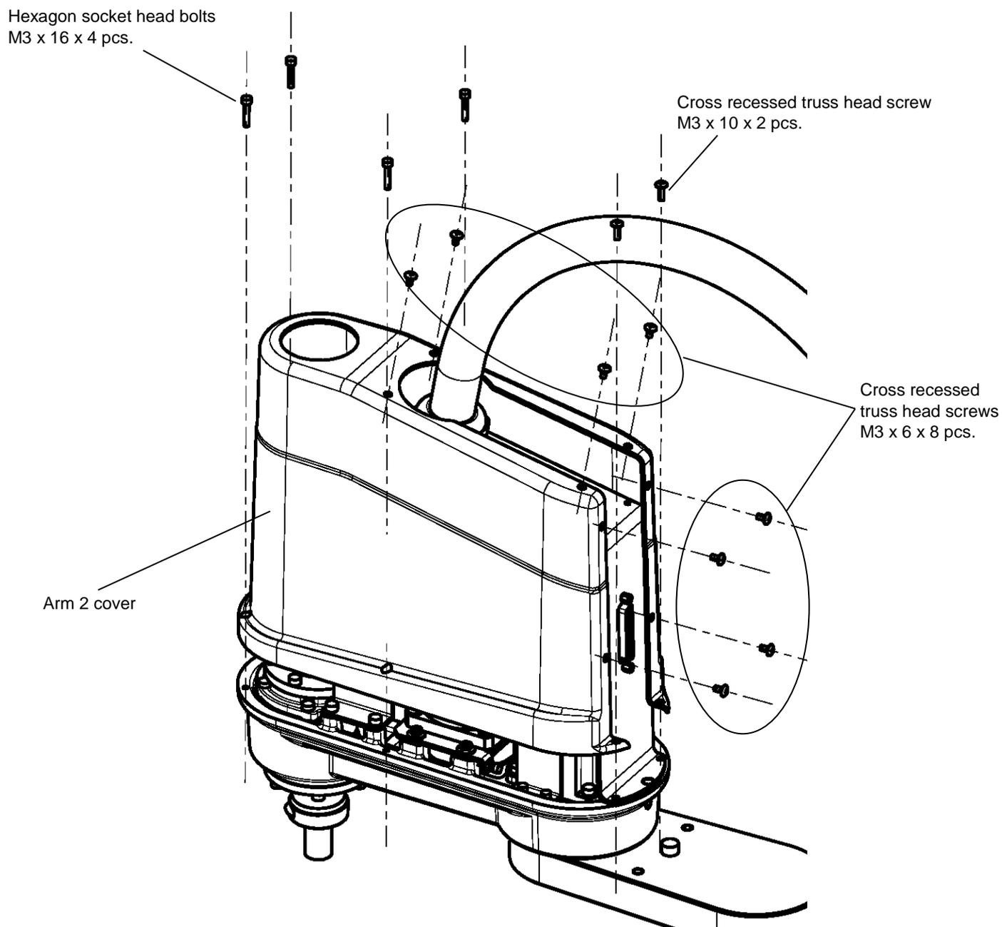
Fig. 5.5 Removing the Arm 2 Cover (KHL-300 and KHL-400)
