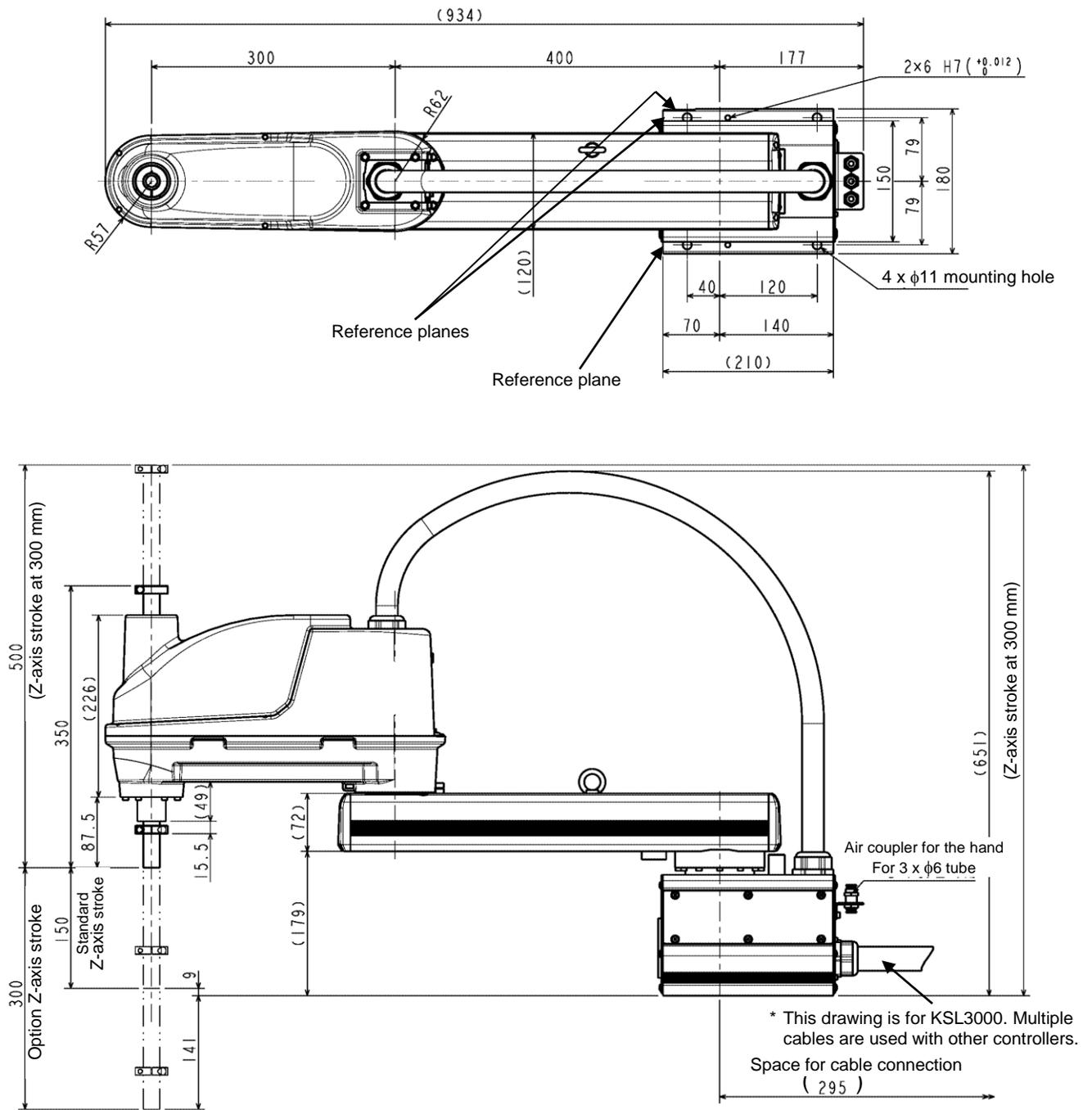
Fig. 2.4 External dimensions of robot (KHL-700)
