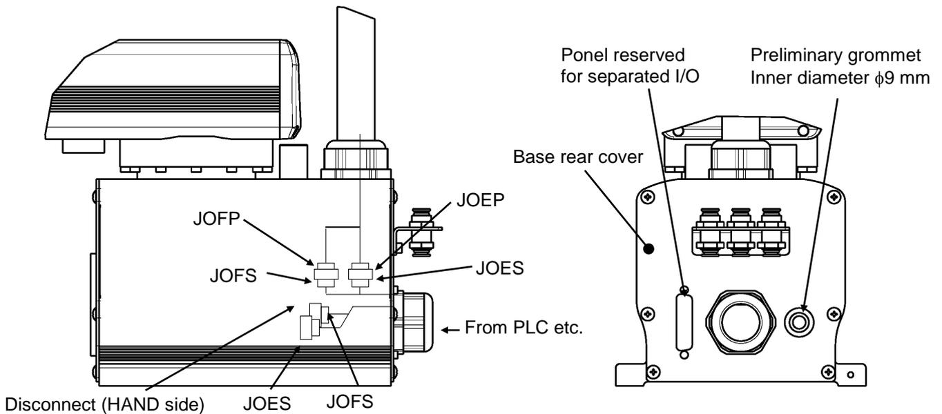
Fig. 11.2 Wiring to PLC, etc. (KHL-500, KHL-600, KHL-700 and KSL3000)
