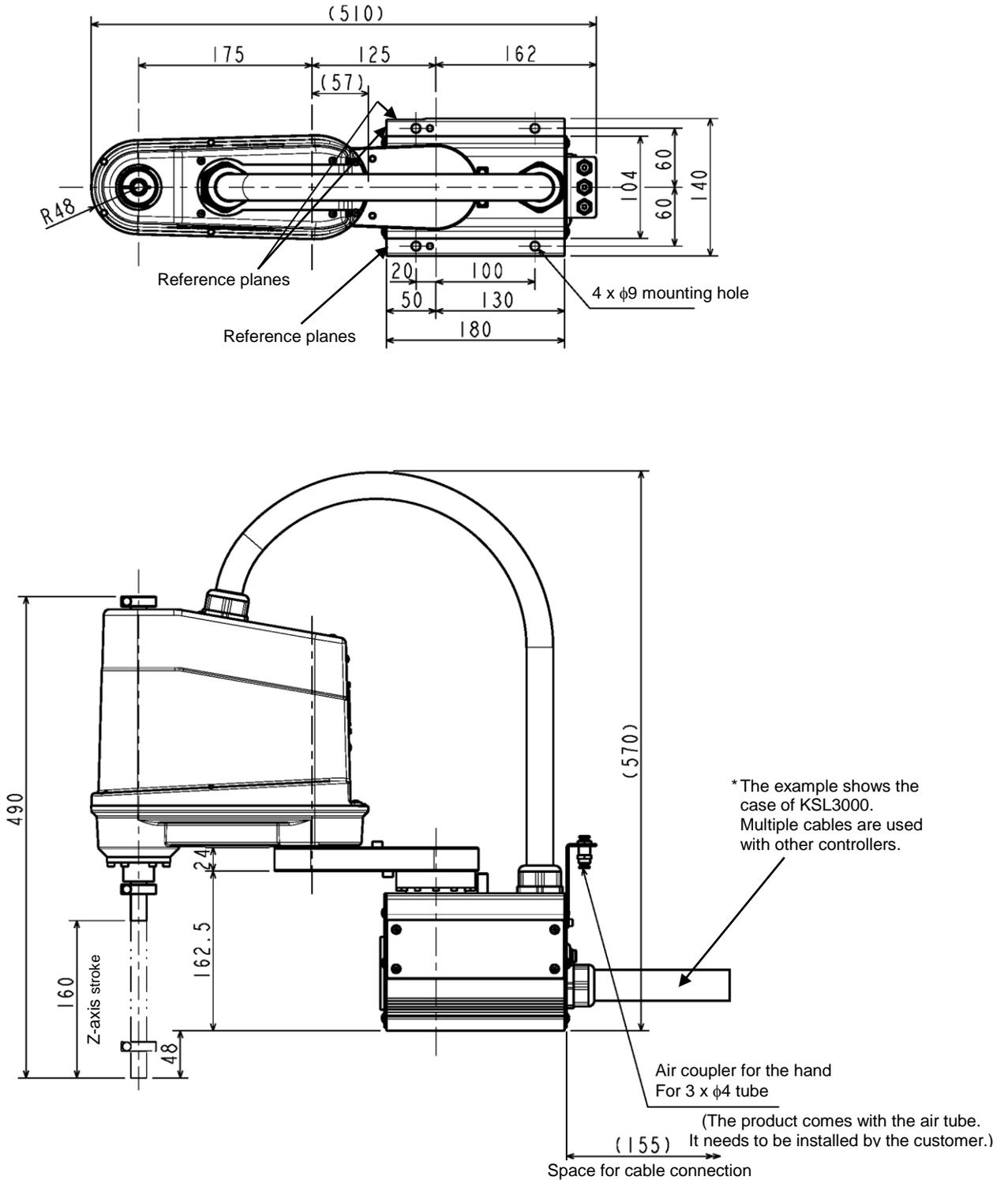
Fig. 1.3 External dimensions of robot (KHL-300)
