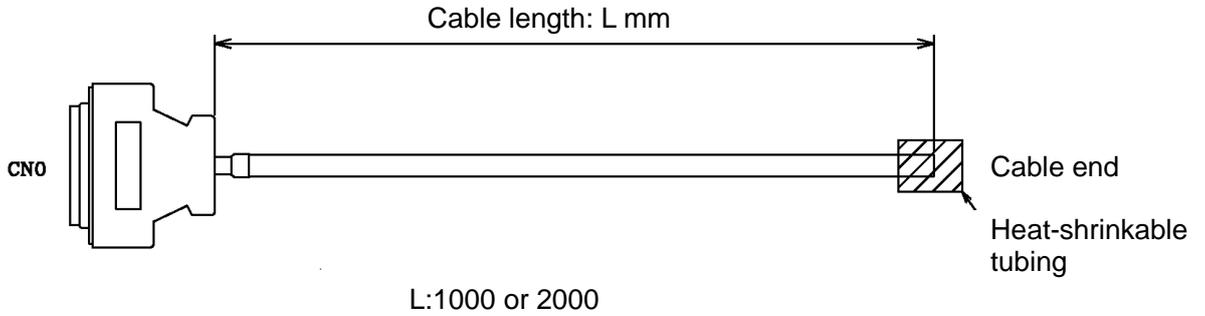
Fig. 11.10 Outline drawing for the hand I/O cable (Option)
