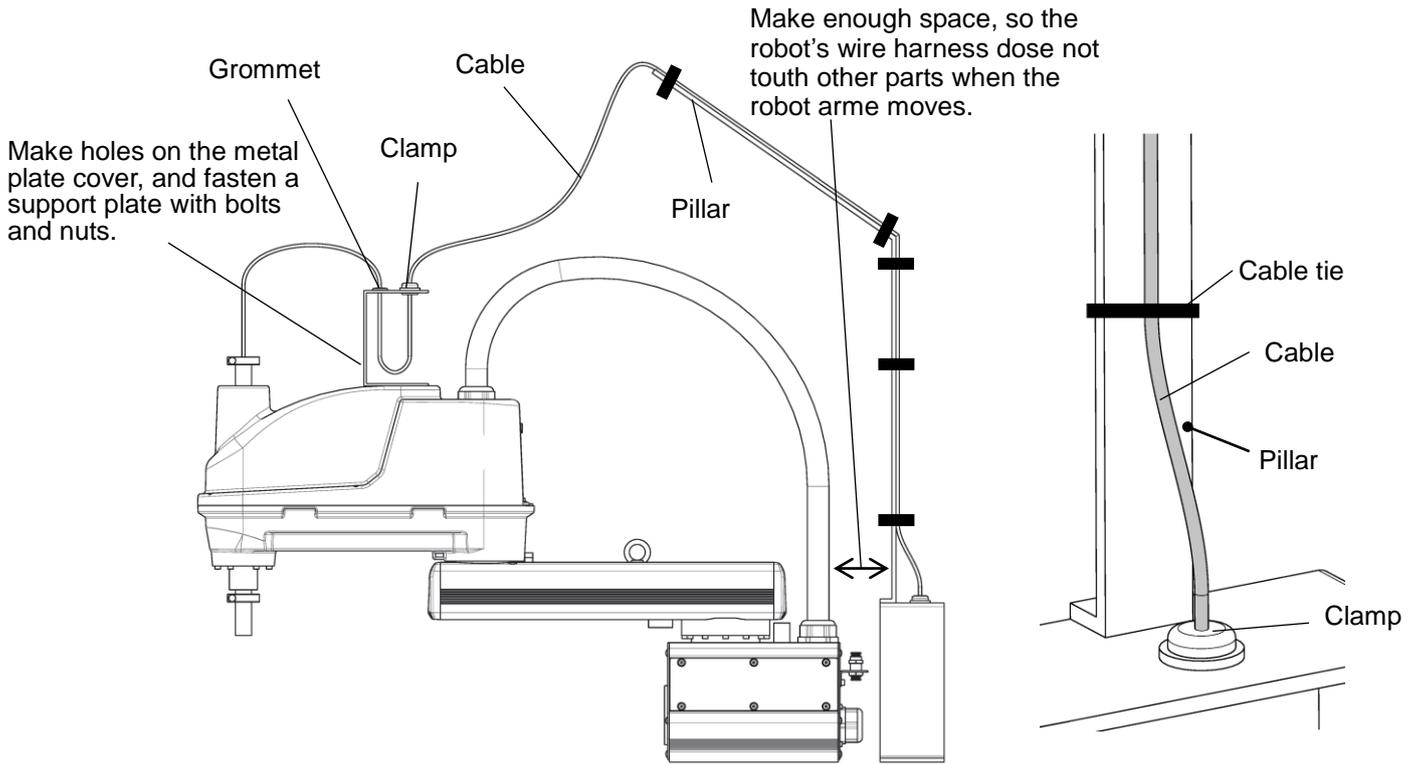
Fig. 11.9 Tool cable wiring installation example (KHL-500/KHL-600/KHL-700)
