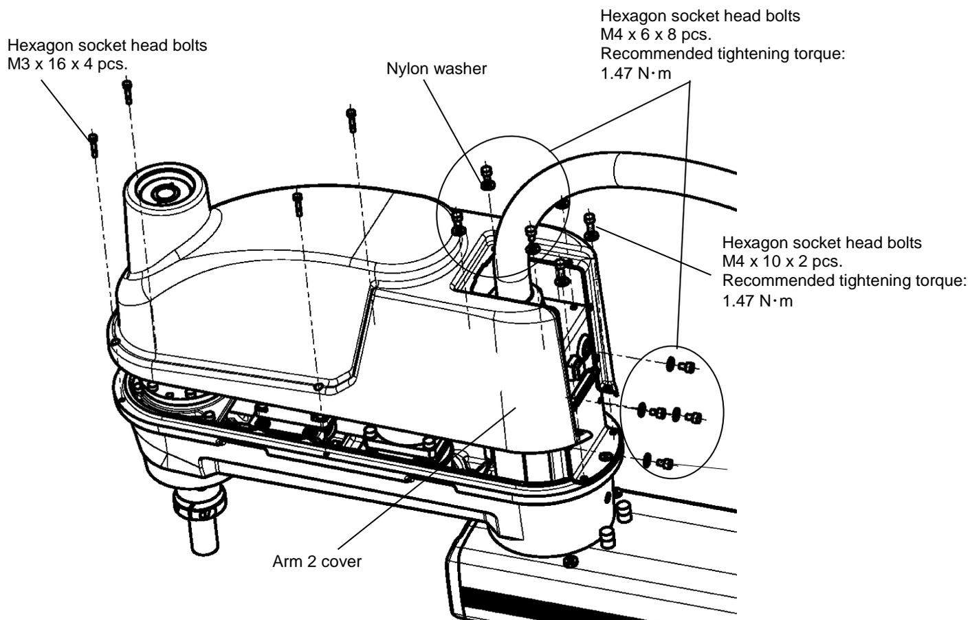
Fig. 6.6 Removing the Arm 2 Cover (KHL-500, KHL-600 and KHL-700)
