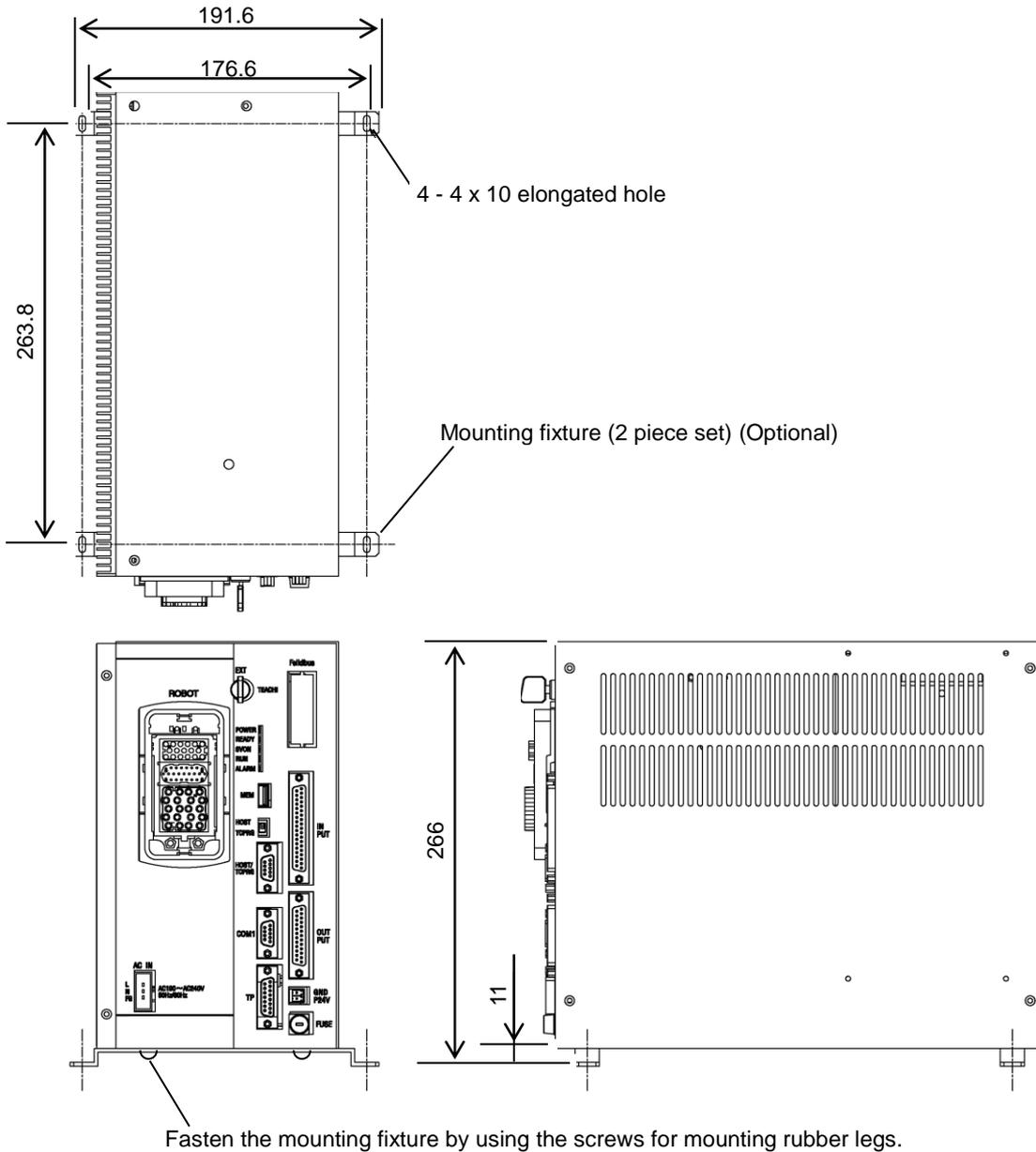
Fig. 7.3 Screw hole dimensions for securing controller (KSL3000)
