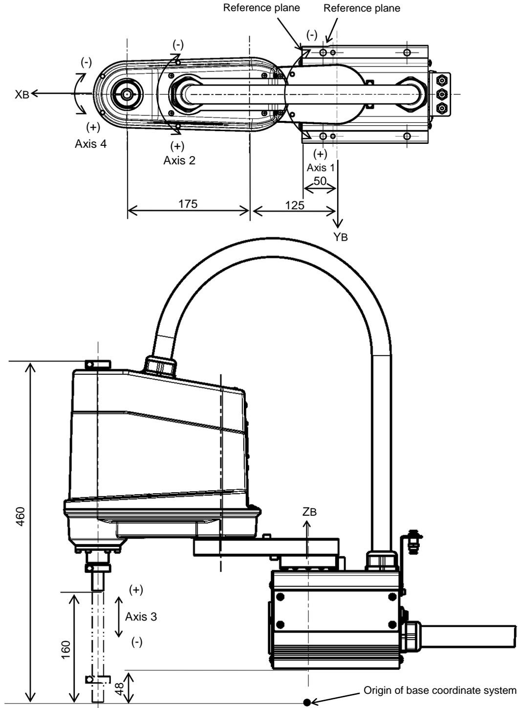
Fig. 5.10 Base coordinate system and joint angle origin (KHL-300)
