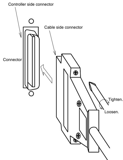
Fig. 8.4 Connecting and disconnecting a square connector (KSL3000)
