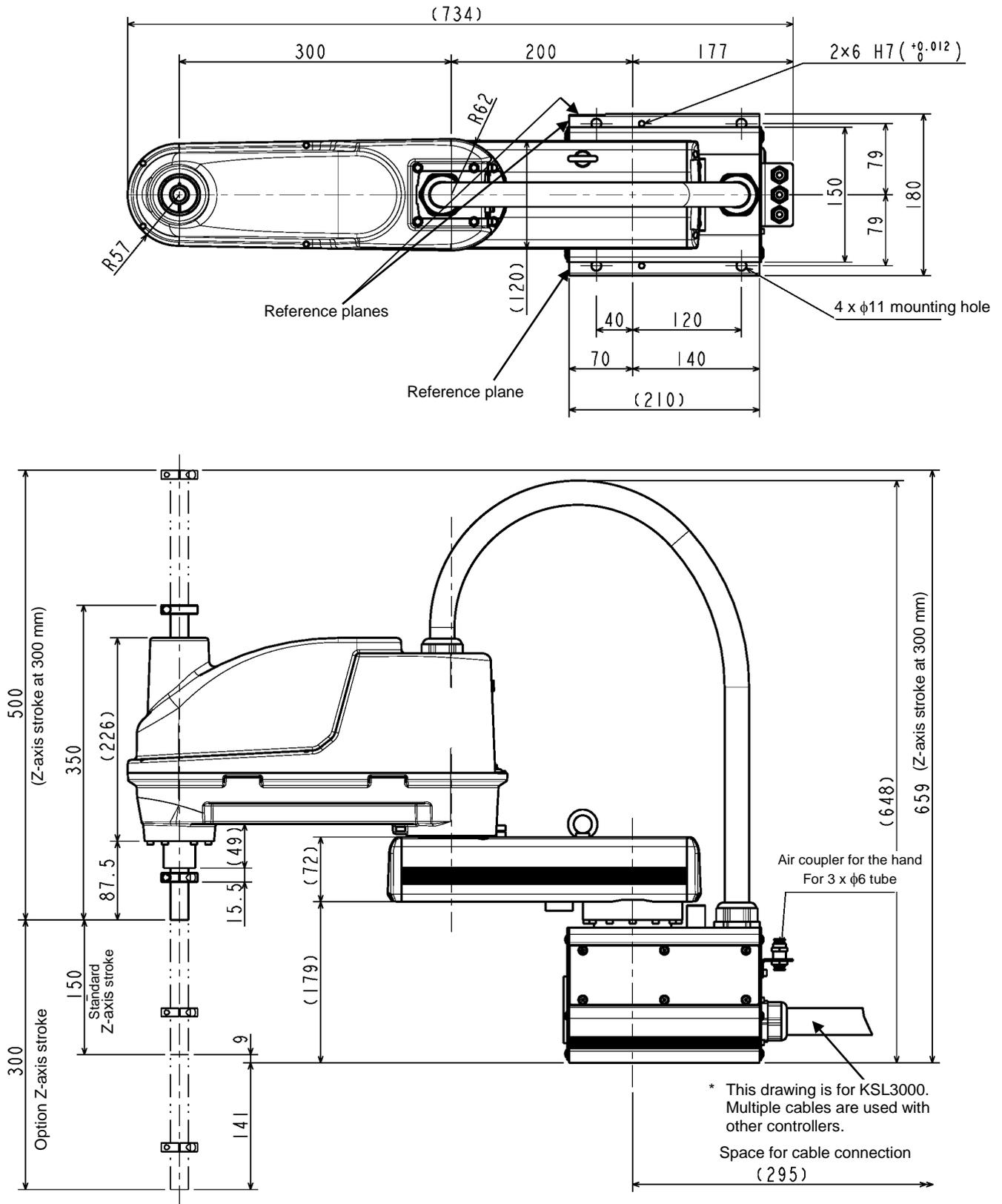
Fig. 2.2 External dimensions of robot (KHL-500)
