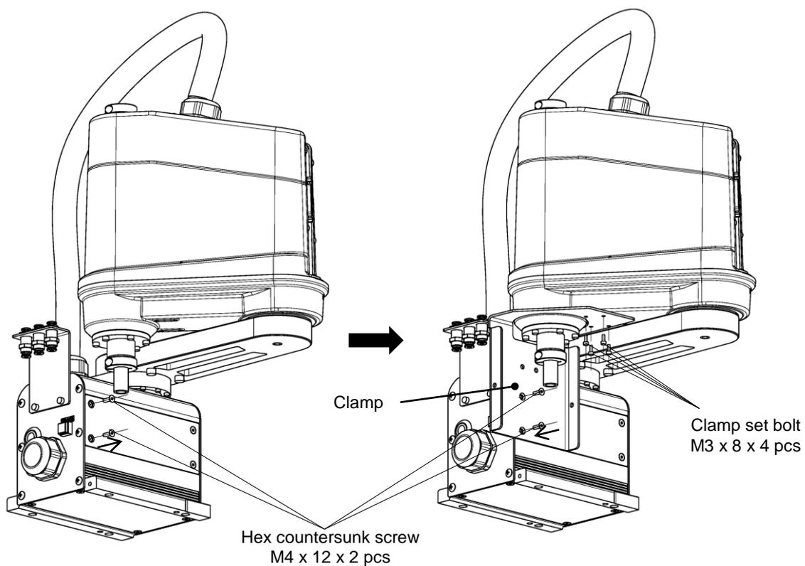
Fig. 3.4 Attaching the clamp (KHL-300/KHL-400)
