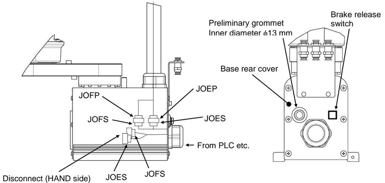
Fig. 11.1 Wiring to PLC, etc. (KHL-300, KHL-400 and KSL3000)
