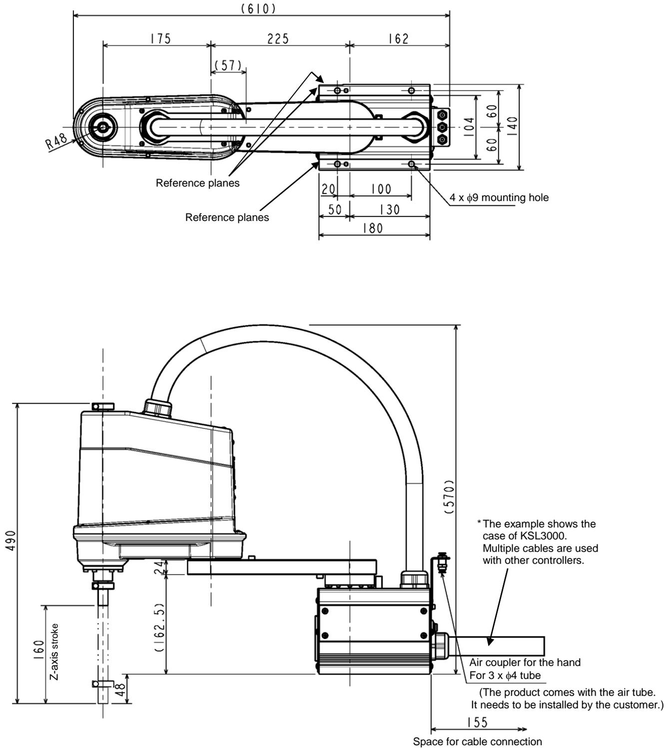
Fig. 1.4 External dimensions of robot (KHL-400)
