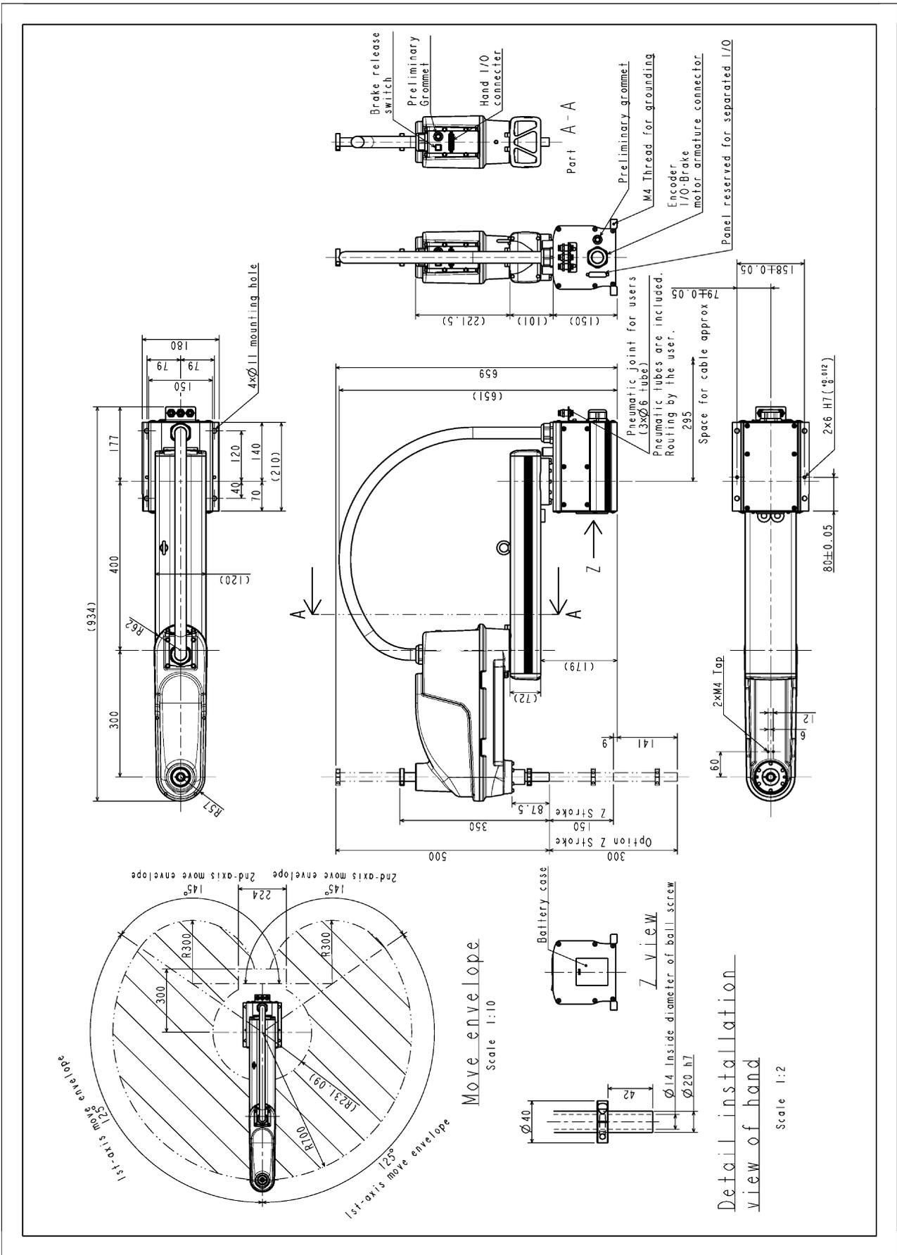
Fig. 6.3 External view and working envelope (KHL-700)
