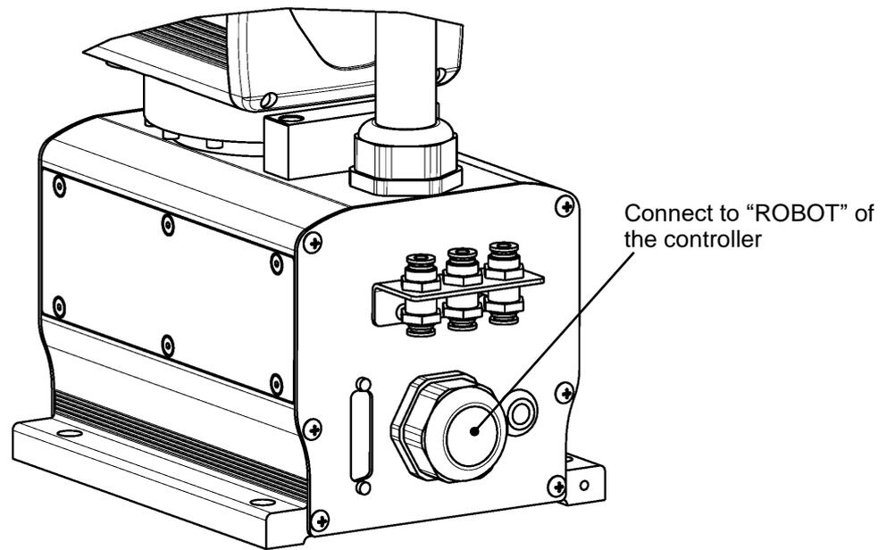
Fig. 8.2 Robot side connector arrangement (KSL3000)
