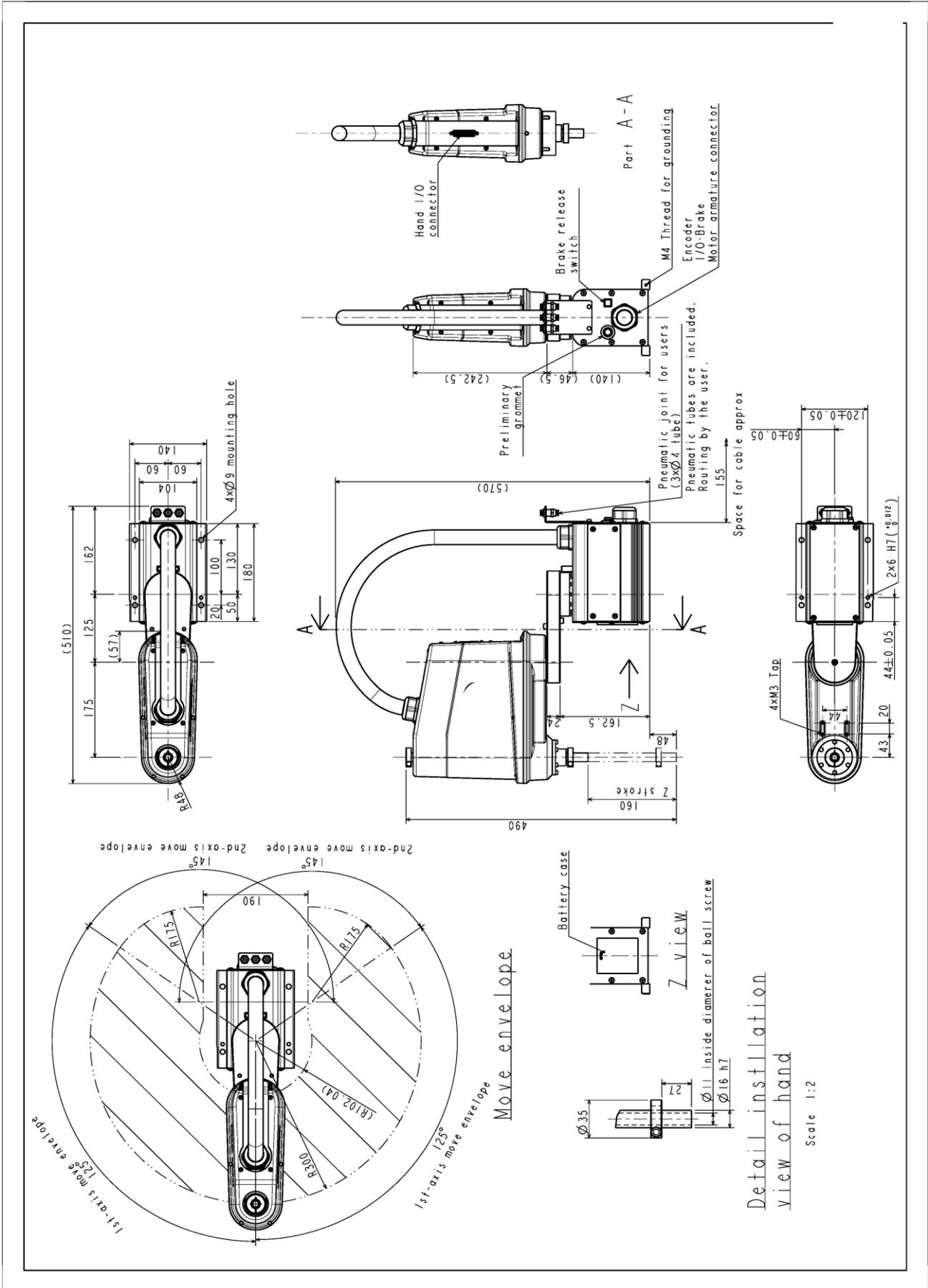
Fig. 5.1 External view and working envelope (KHL-300)
