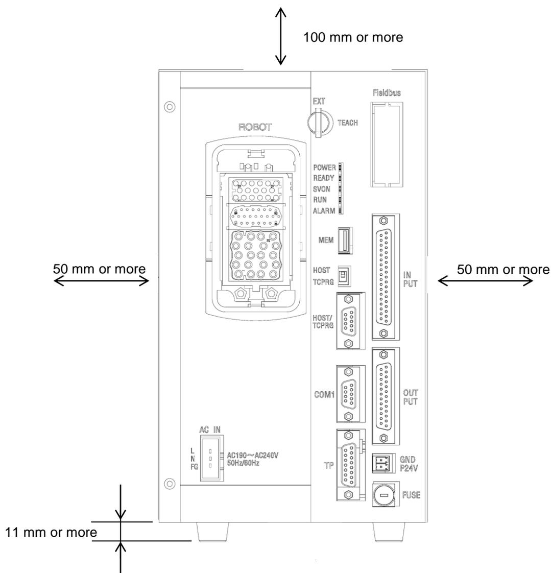
Fig. 7.2 Controller ventilation space (KSL3000)
