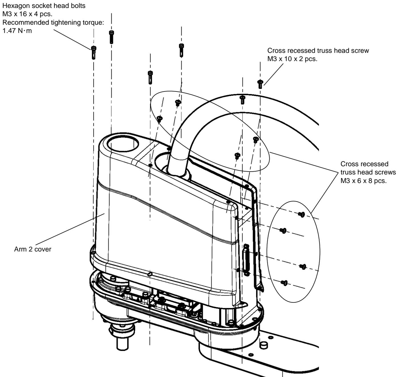
Fig. 5.9 Removing the Arm 2 Cover (KHL-300 and KHL-400)
