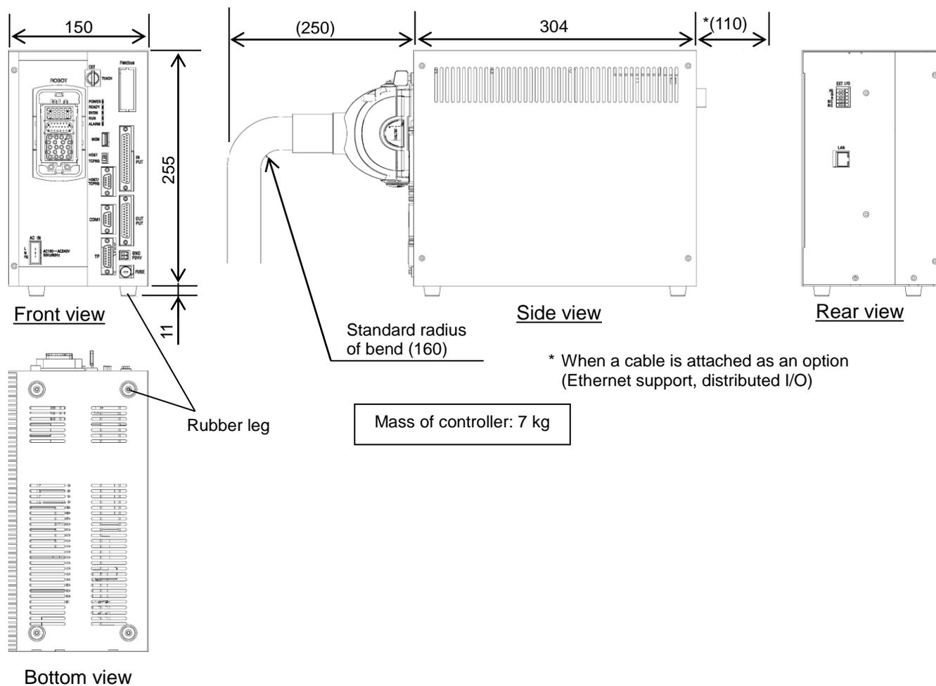
Fig. 7.1 External view of controller (KSL3000)
