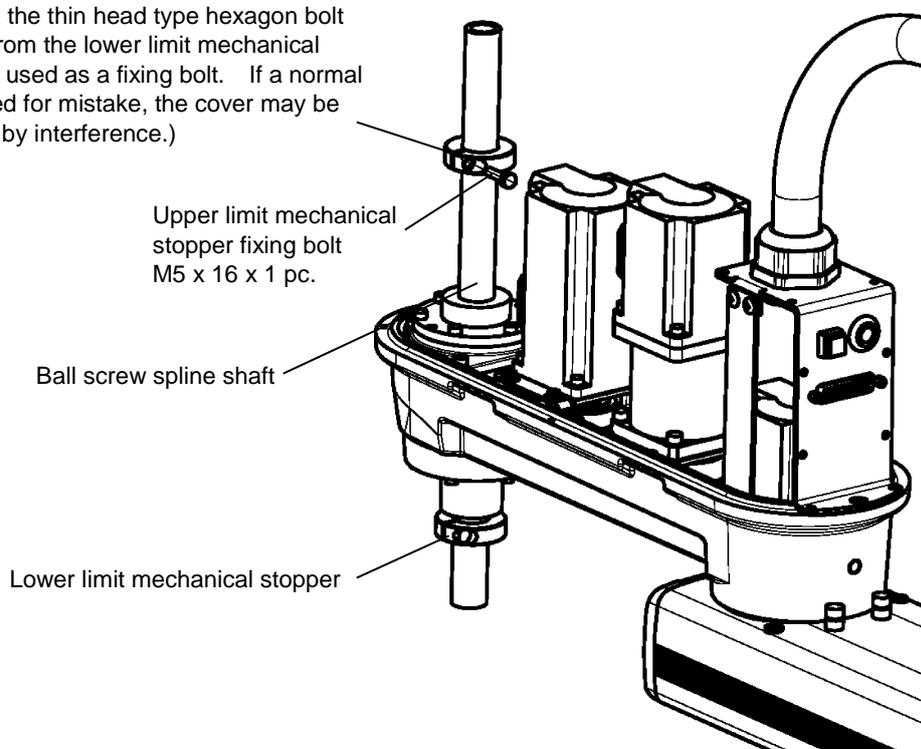
Fig. 6.7 Checking Software Limit Change (KHL-500, KHL-600 and KHL-700)
