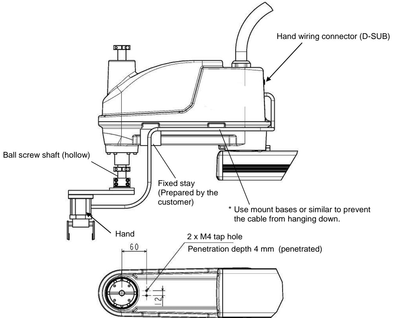
Fig. 11.7 Tool cable wiring installation example using the connector (D-SUB)
