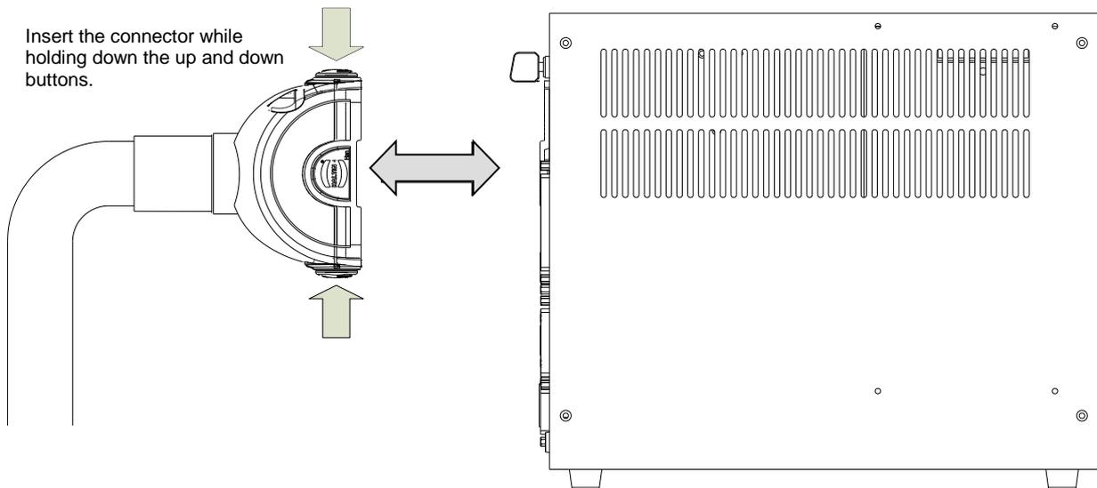
Fig. 8.3 Connecting and disconnecting the ROBOT connector (KSL3000)
