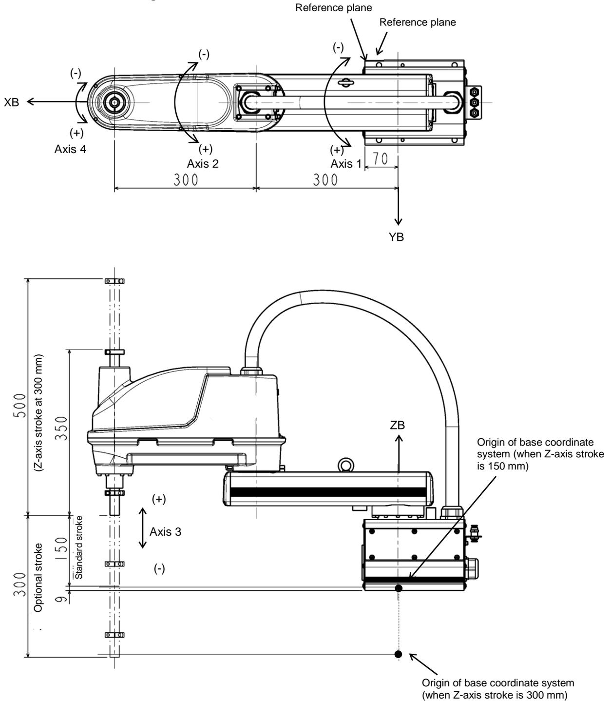
Fig. 6.12 Base coordinate system and joint angle origin (KHL-600)
