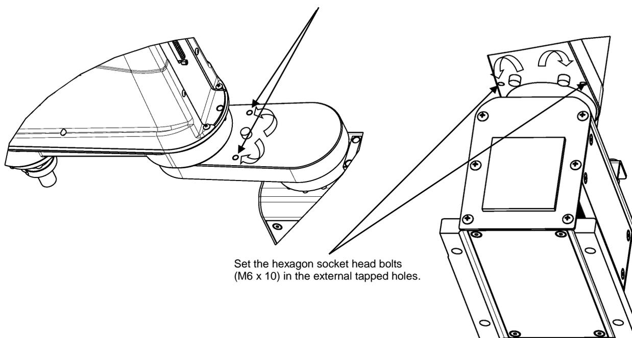
Fig. 5.3 Changing the Operating Ranges of Axes 1 and 2 (KHL-300 and KHL-400)
