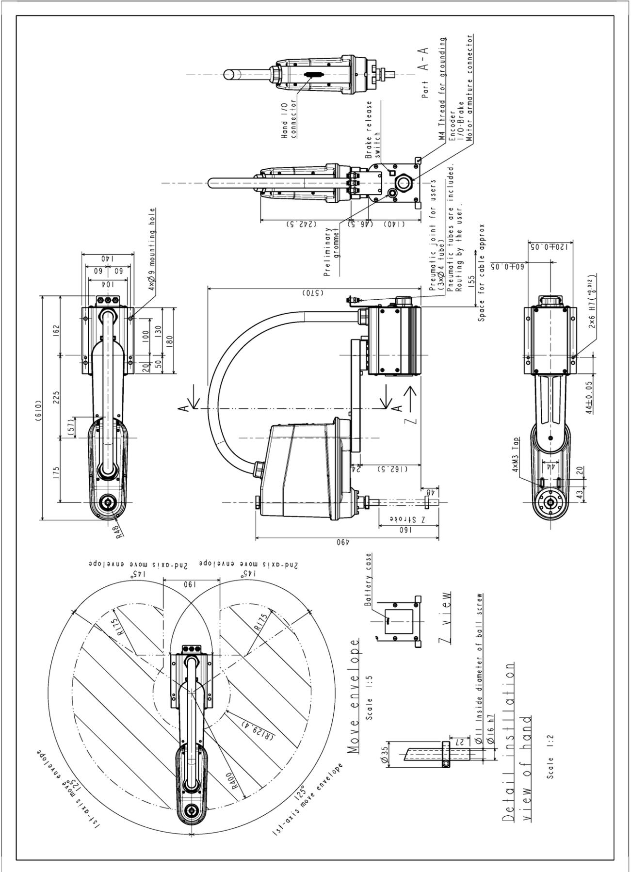
Fig. 5.2 External view and working envelope (KHL-400)
