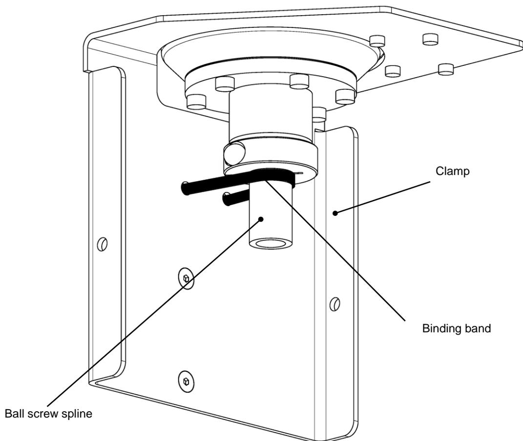
Fig. 3.5 Fixing the ball screw spline (KHL-300/KHL-400)
