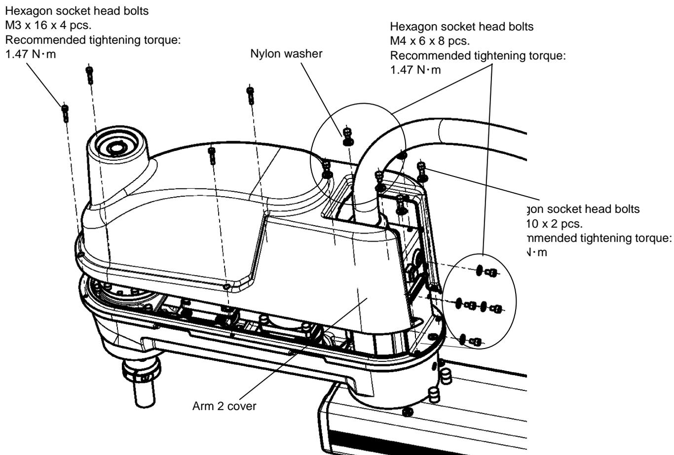
Fig. 6.11 Removing the Arm 2 Cover (KHL-500, KHL-600 and KHL-700)
