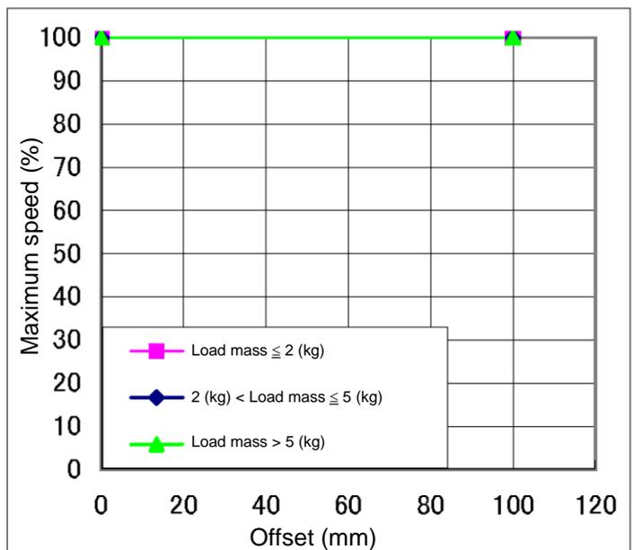
Setting of acceleration/deceleration in relation to offset (Axis 4)
