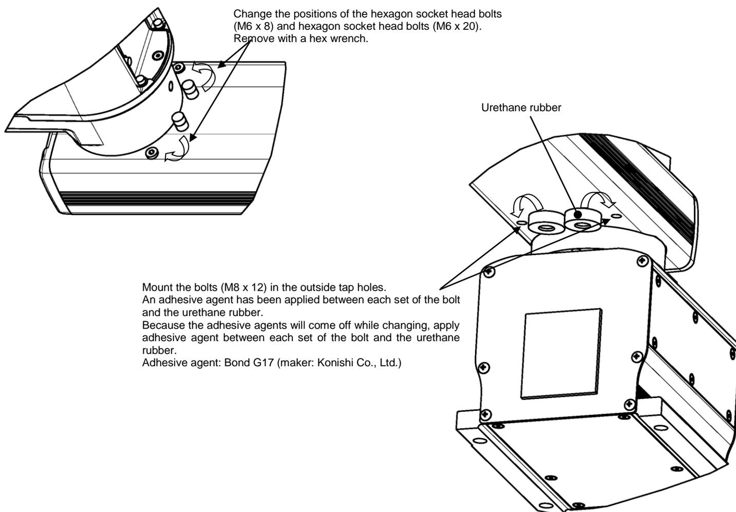
Fig. 6.4 Changing the Operating Ranges of Axes 1 and 2 (KHL-500, KHL-600 and KHL-700)
