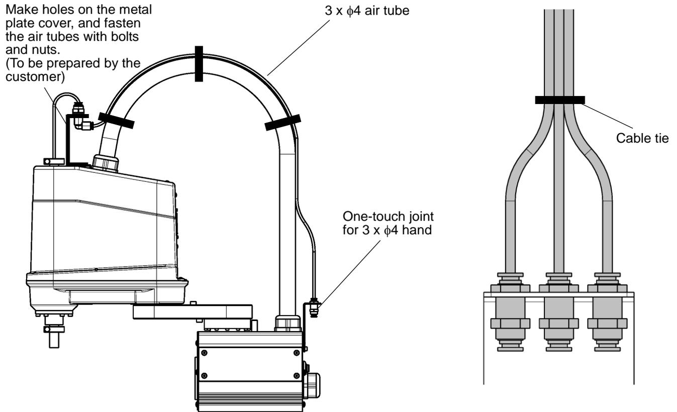
Fig. 9.2 Tool air piping installation example (KHL-300 and KHL-400)
