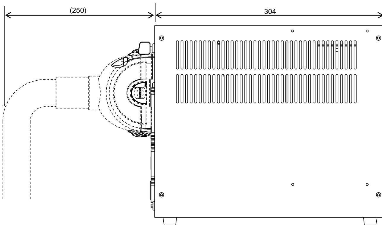
Fig. 7.5 Clearance of controller front side (KSL3000)
