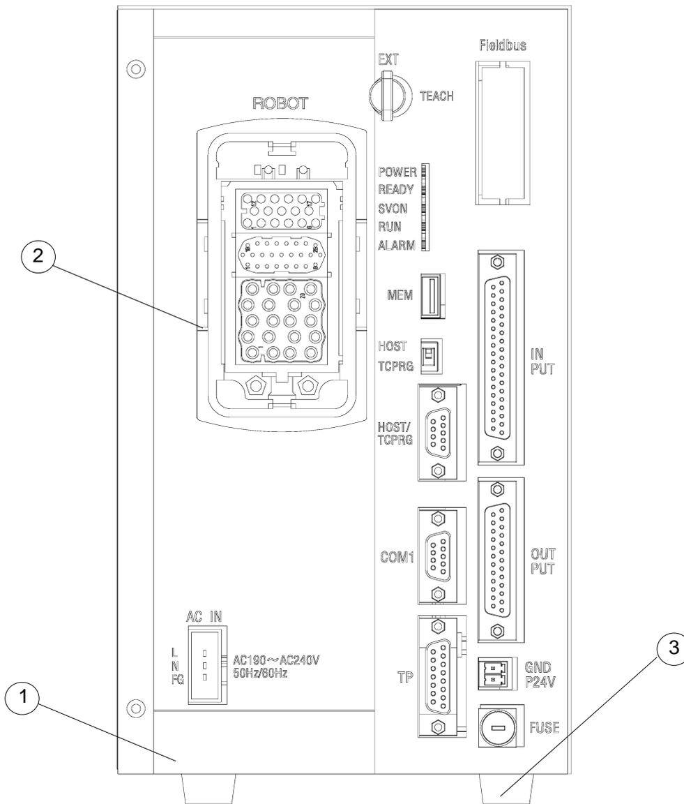
Fig. 8.1 Robot controller connector arrangement (KSL3000)
