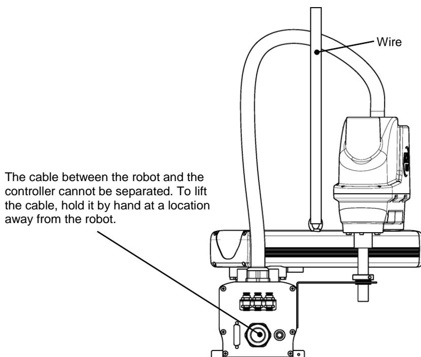
Fig. 4.6 Lifting up the robot
