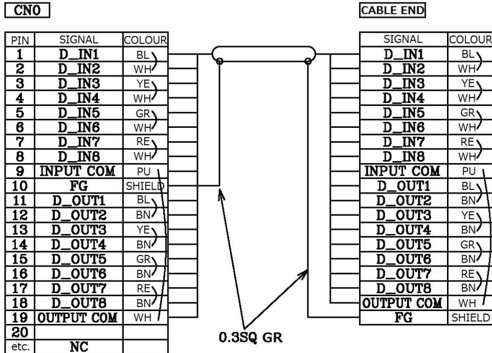
Fig. 11.11 The wiring arrangement for the hand I/O cable (Option)
