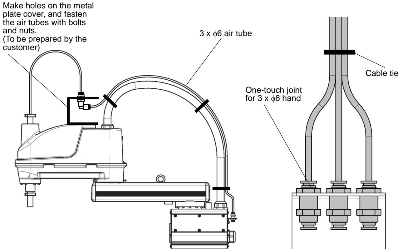
Fig. 10.2 Tool air piping installation example (KHL-500, KHL-600 and KHL-700)
