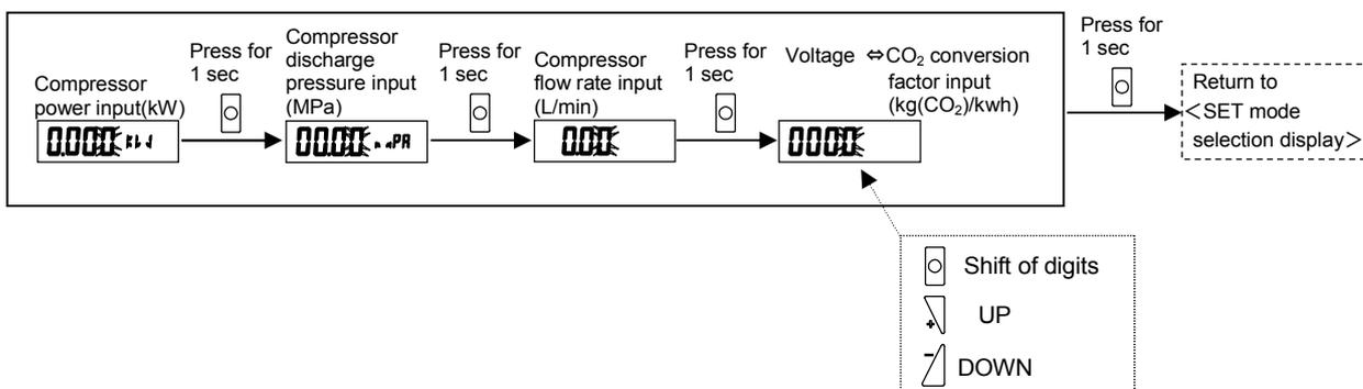
$$\frac{\text{Integrated flow (L)}}{\text{Compressor flow rate(L/min)} \times \frac{(\text{Discharge pressure (MPa)} \times 0.1013)}{0.1013}} \times \text{Compressor power (kW)} \div 60(\text{min}) \times \text{CO}_2 \text{ conversion factor (kg(CO}_2\text{)/kWh)}$$
