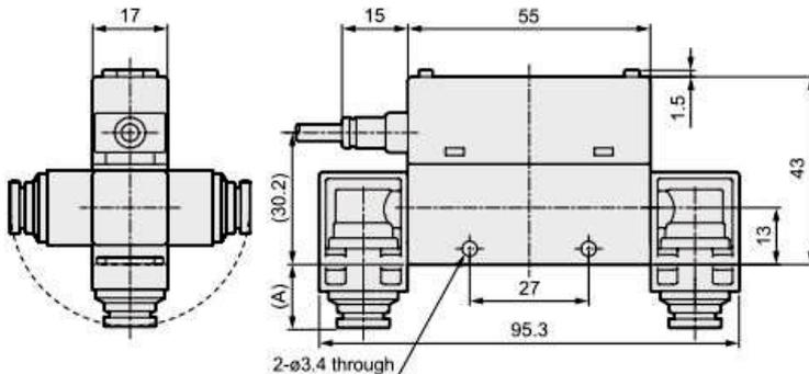
Note: Because it causes external leakage, please do not turn the joint while adding fluid pressure to this product. Also, please do not use in a way to rotate the fitting during use.
