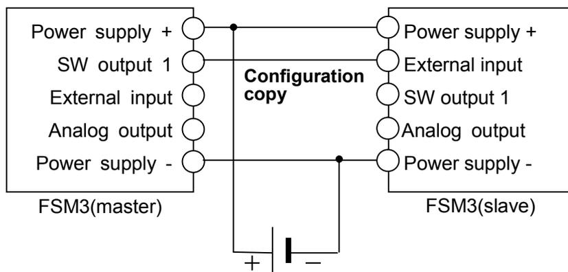
Connect CH1(SW output) of the origin of copy (master) and CH2 (copy terminal) of the copy destination (Slave).
