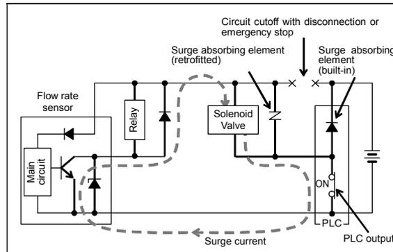
Take countermeasures as followings to prevent damage caused by reverse current.
