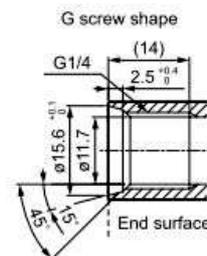
15° of the surface is the seal surface. Note that it is not the end surface seal. Also, be sure to confirm that the screw depth of the fitting matches before use.
