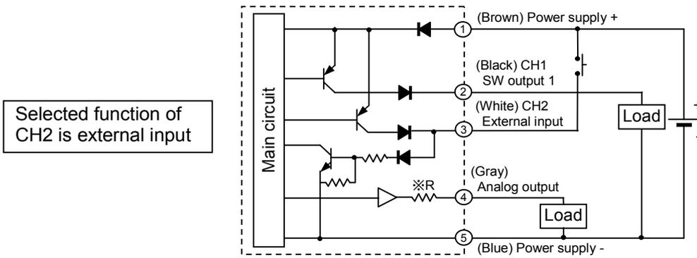
●FSM3-L\*\*\*\*C/G (One analog, One switch, Copy function)
