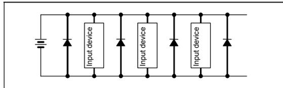
When the devices are connected to a connector, the output circuit could be damaged by the above phenomenon if the connector is disconnected while the power is ON. Turn the power OFF before connecting or disconnecting the connector.
