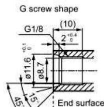
15° of the surface is the seal surface. Note that it is not the end surface seal. Also, be sure to confirm that the screw depth of the fitting matches before use.
