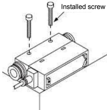
Vertical mounting (use of female thread on bottom surface)
