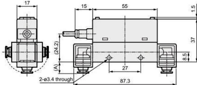
Note: Because it causes external leakage, please do not turn the joint while adding fluid pressure to this product. Also, please do not use in a way to rotate the fitting during use.
