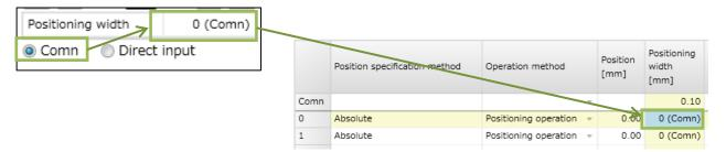
The value that is input after selecting the [Direct input] radio button is reflected in the cell selected in the Point data list. Selecting the [Direct input] radio button changes the value in the cell from "0 (Comn)" to the default value. The value can be input directly without selecting the [Direct input] radio button. Values other than "0" are reflected in the selected cell. Entering "0" switches the value to "0 (Comn)."
