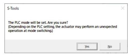
When operating the actuator from an upper level equipment, set the controller to the PLC mode. In the TOOL mode, the controller does not accept operations from tan upper level equipment (such as PLC).
