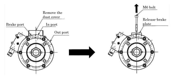
To start a normal operation, make sure that the bolt is removed and the dustproof covering is installed in position.
