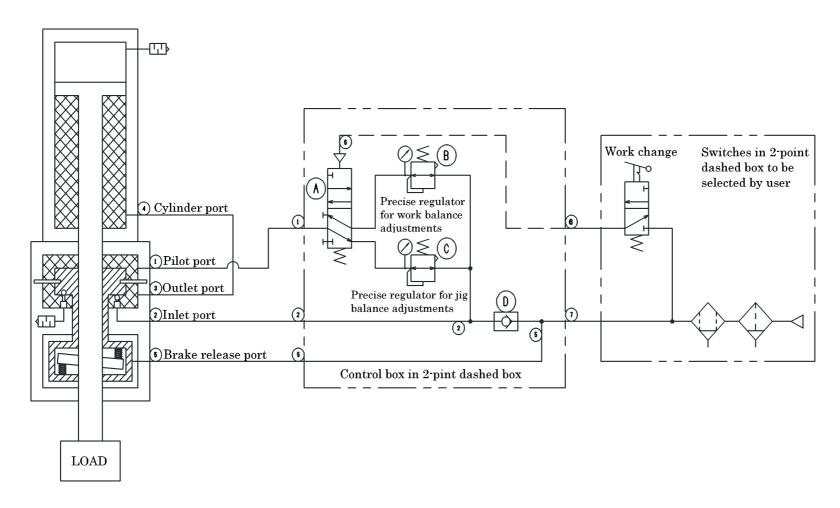
Circuit diagram above is the case that the load direction is the extend side (D), and piping of cylinder is head side. When the load direction is retracting side (U), piping of cylinder is head side.
