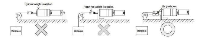
3) If the unit is used on a link basis, make sure that a constant lever ratio is maintained (for example, on a mobile fulcrum basis). If the lever ratio varies in a vertical motion, the load will ascend or descend depending on the position of detection, regardless of manual operation.
