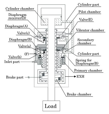
As a result, the pressure applied to the secondary chamber, pilot chamber, and cylinder chamber is increased to lift the load, elevate Diaphragm (A), open Valve (c), apply the same pressure to the vibrator chamber as in the secondary chamber (Figure 2), elevate Diaphragm (B), and release pressure from Valve (b) (Figure 3)
