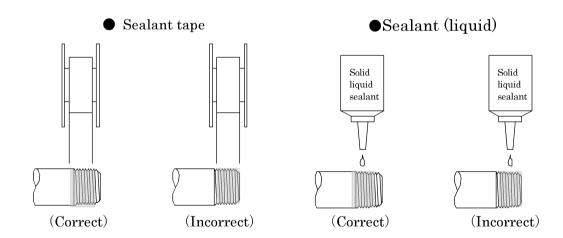
6) Refrain from applying sealant or sealing tape approx. Two pitches of thread off the tip of pipe to avoid residual substances from falling into piping system.
