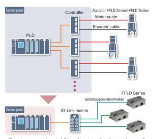
\*Separate power supply is required. Refer to the system configuration example on page 7
