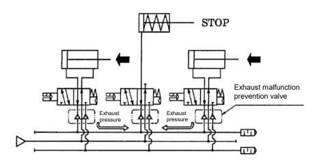
• PR check valve and exhaust malfunction prevention valve
