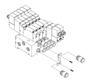
**5** Pull on the fitting and confirm that it is installed correctly.
