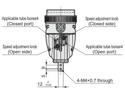
Dimensions when attachment is installed
