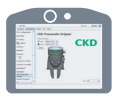
The digital I/O can be configured while viewing a graphic display of the gripper's open/closed status.
