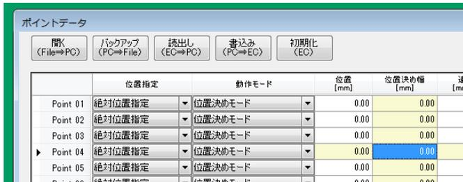
When writing the point data into the controller, click [Write (PC => EC)].
