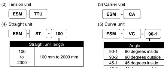
Note: We accept special orders for the length between 100 mm to 2000 45-2 45 degrees outside mm by 1 mm increment.
