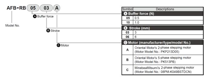
Although the motor is a special order model number for AFB-RB, refer to the above model number to check motor specifications.
