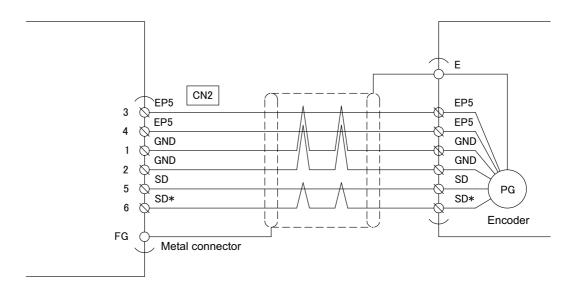
Figure 3-2 Serial encoder connecting diagram
