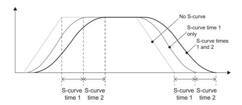
Figure 5-6 S-curve acceleration/deceleration operation example
