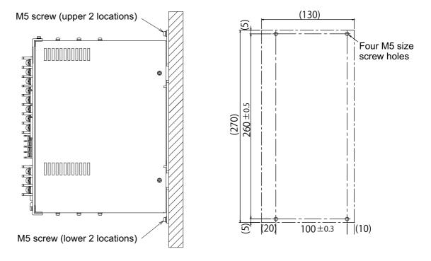
Figure 2-5 Device installation method (3.3 kW)
