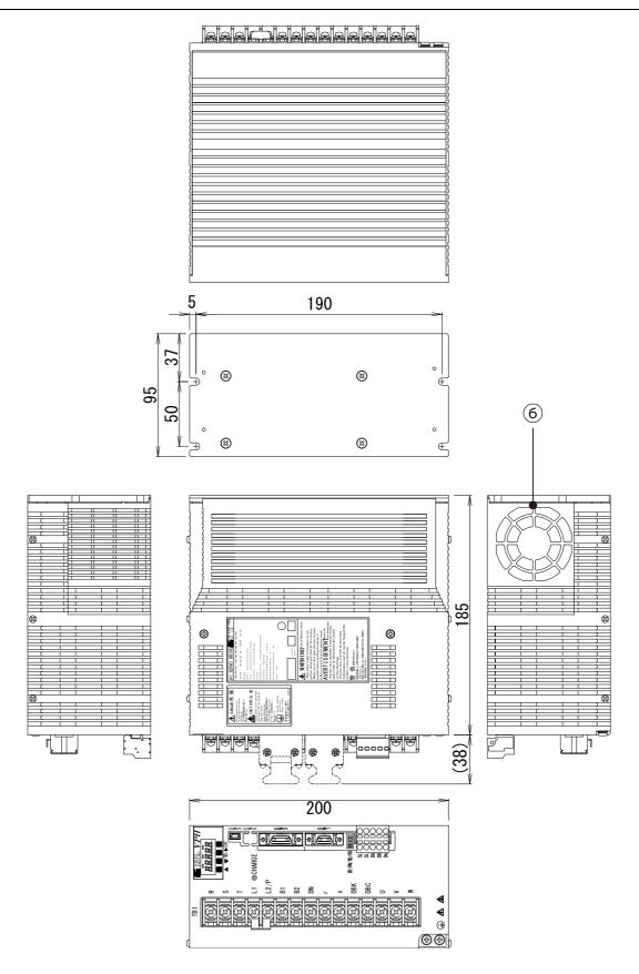
Figure 13-5 Outline drawing of the main unit of the device with 1.5 kW or 2.2 kW (Type 3)
