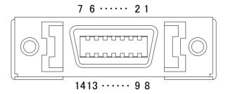
The figure below is the connector alignment of the cable side viewed from the soldering terminal side.
