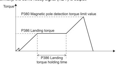
Figure 6-1 Single pattern operation of auto magnetic pole detection
