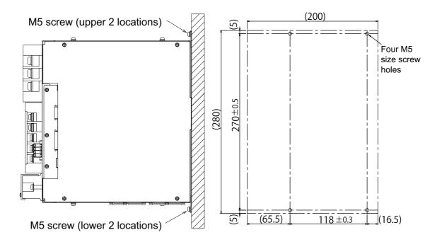
Figure 2-7 Device installation method (15 kW)
