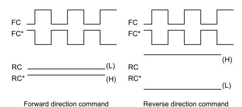
Figure 3-5 Direction signal + Feed pulse
