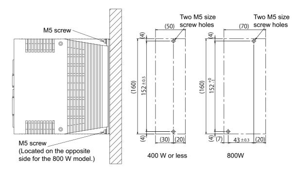
Figure 2-3 Device installation method (800 W or less)
