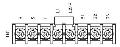
Connect the grounding to the grounding terminal on the device cabinet. When not using a DC reactor, do not remove the shorting bar between L1 and L2/P.
