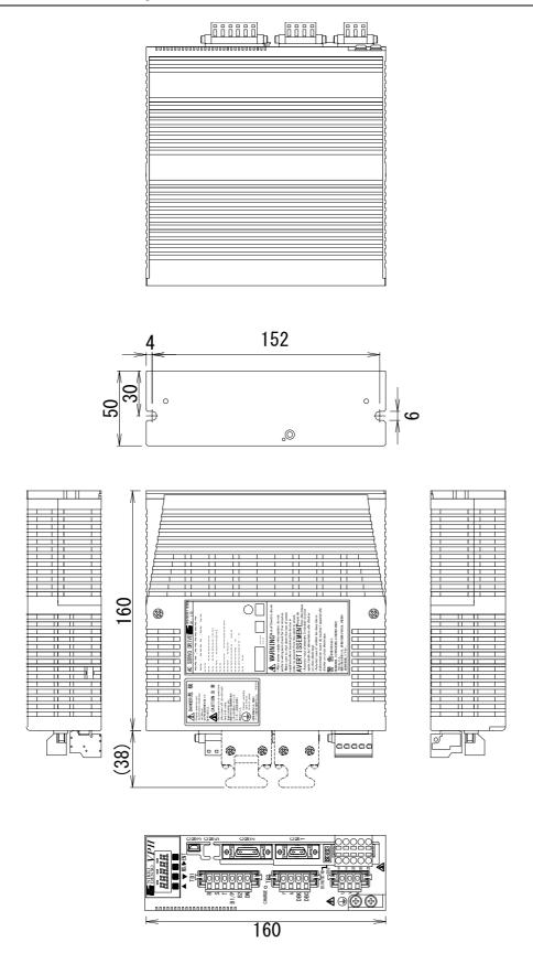
Figure 13-1 Outline drawing of the main unit of the device with up to 400 W (Type 1)
