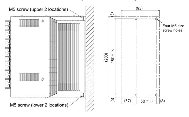
Figure 2-4 Device installation method (1.5 kW, 2.2 kW)
