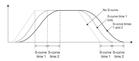
Figure 5-9 S-curve acceleration/deceleration operation example
