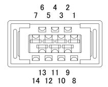
Table 3-1 Control input/output connector pin alignment
