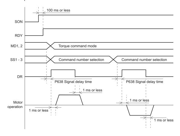
Figure 5-3 Internal torque command time chart
