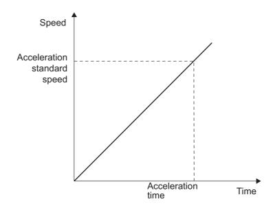
Figure 5-8 Acceleration standard speed in relation to acceleration time at built-in command mode
