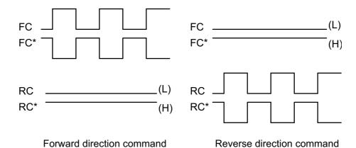
Figure 3-4 Direction-specific pulses
