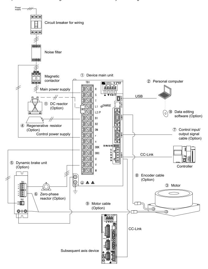
Figure 1-2 VPH HC Type system configuration for the 1.5 kW or more
