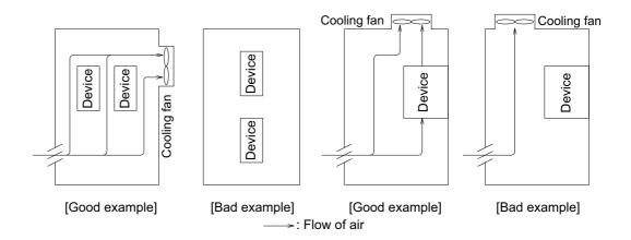
Figure 2-1 Alignment example for storing devices
