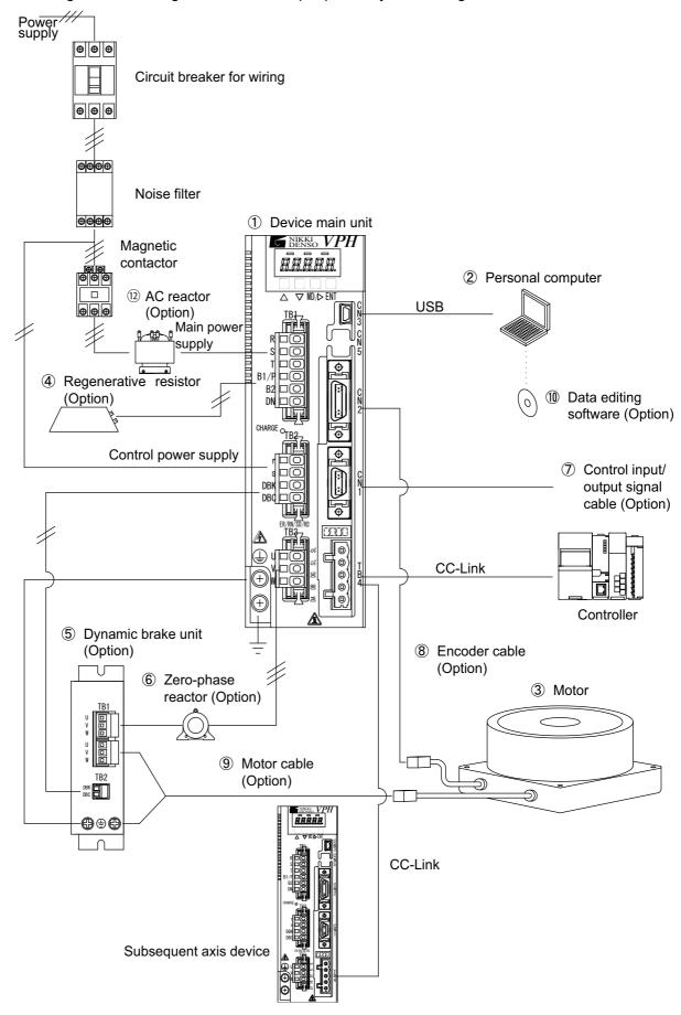
Figure 1-1 VPH HC Type system configuration for the 800 W class or less
