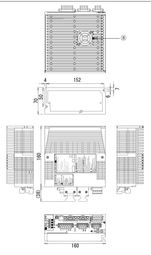
Figure 13-3 Outline drawing of the main unit of the device with 800 W (Type 2)
