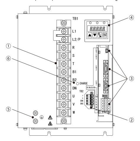
Figure 13-10 Front view of the main unit of the device with 7 kW (Type 5)
