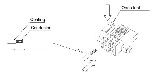
Figure 2-13 Plug connector wiring diagram
