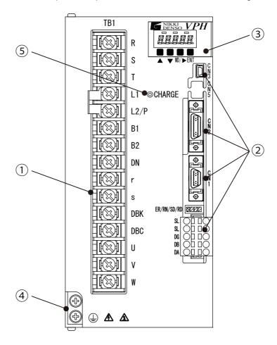
Figure 13-6 Front view of the main unit of the device with 1.5 kW or 2.2 kW (Type 3)
