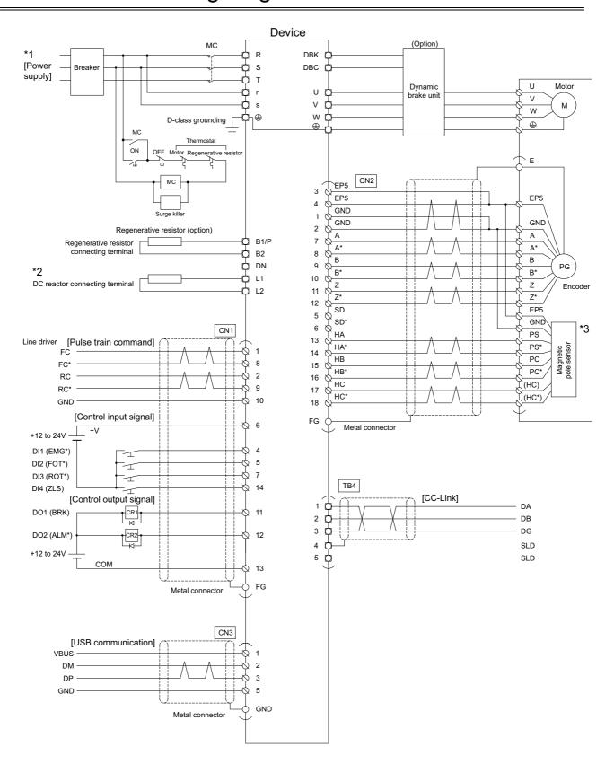
Figure 3-1 External wiring diagram
