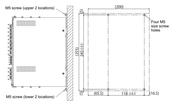
Figure 2-6 Device installation method (7 kW)
