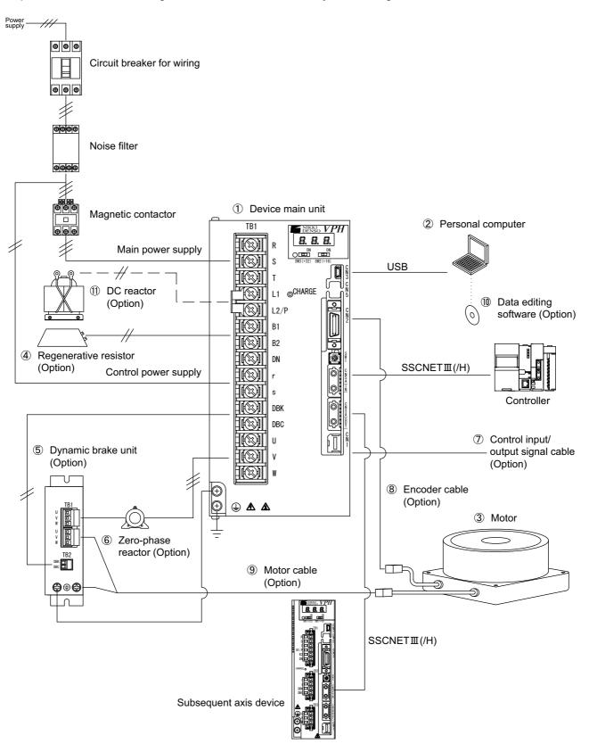
Figure 1-2 VPH HB Type system configuration for the 1.5 kW or more
