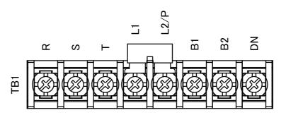
Connect the grounding to the grounding terminal on the device cabinet. When not using a DC reactor, do not remove the shorting bar between L1 and L2/P.
