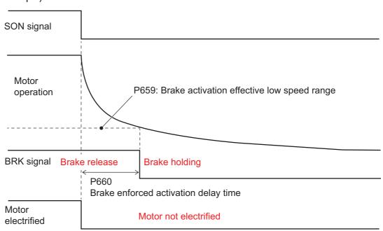
3 If the emergency stop signal (EMG) is turned ON during motor operation
