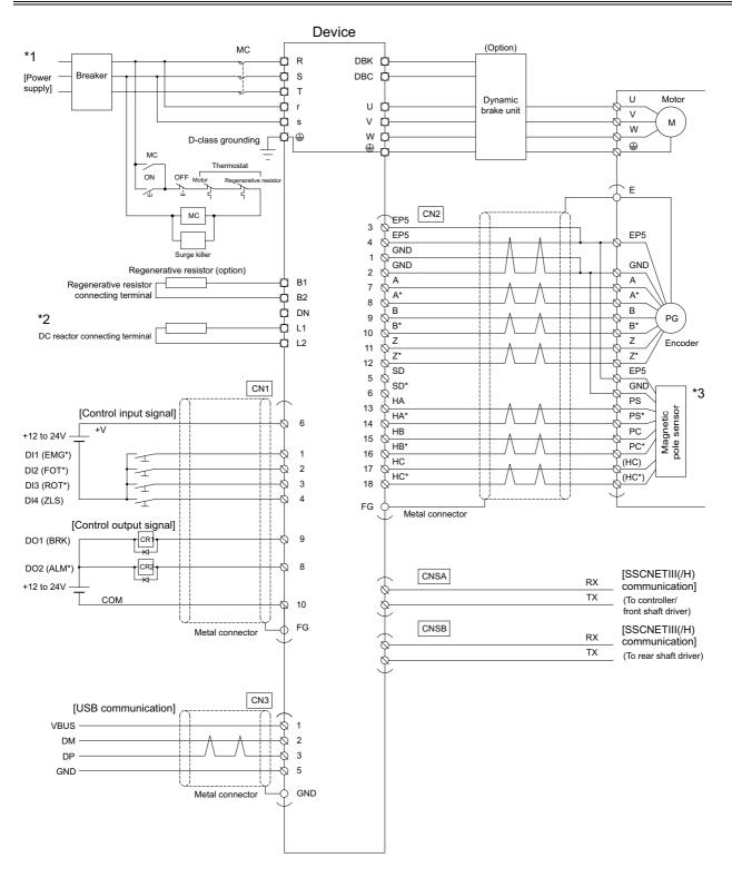
Figure 3-1 External wiring diagram
