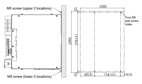
Figure 2-7 Device installation method (15 kW)
