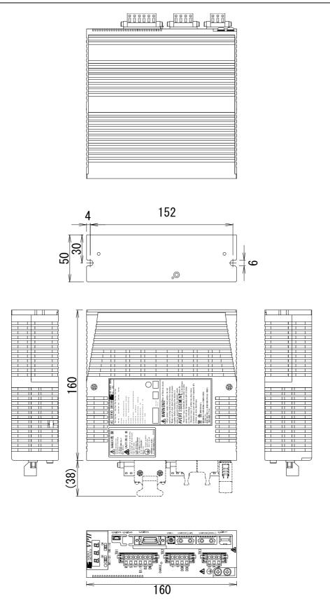
Figure 12-1 Outline drawing of the main unit of the device with up to 400 W (Type 1)
