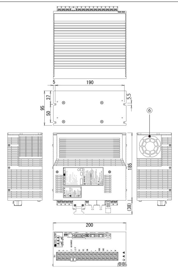
Figure 12-5 Outline drawing of the main unit of the device with 1.5 kW or 2.2 kW (Type 3)
