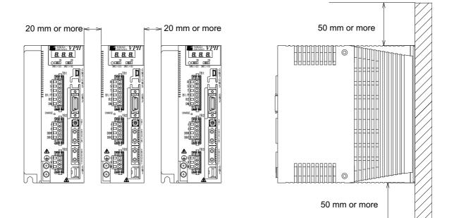
Figure 2-2 Installation and ventilation of the device
