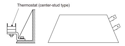
Figure 2-11 Mounting a thermostat on a cement resistor
