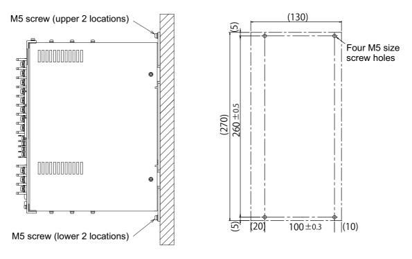
Figure 2-5 Device installation method (3.3 kW)
