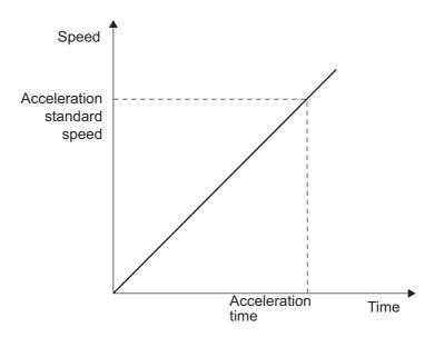
Figure 5-2 Acceleration standard speed in relation to acceleration time at speed command mode
