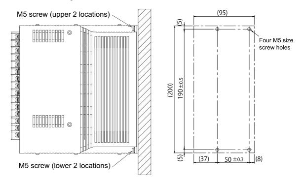
Figure 2-4 Device installation method (1.5 kW, 2.2 kW)
