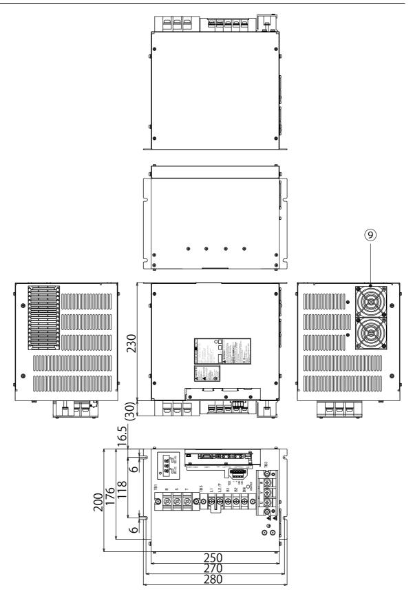
Figure 12-11 Outline drawing of the main unit of the device with 15 kW (Type 6)
