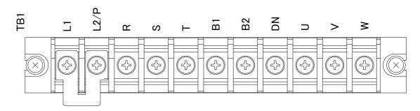
Connect the grounding to the grounding terminal on the device cabinet. When not using a DC reactor, do not remove the shorting bar between L1 and L2/P.
