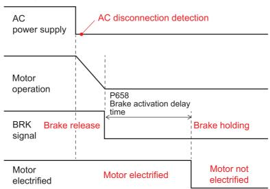
\* Depending on the status of the device, the motor un-electrified status may be assumed before the elapse of the [P658 (8th - 5th digits)] time.
