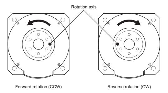
Figure 4-1 Run direction of the TDISC motor
