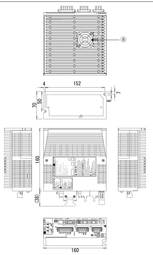
Figure 12-3 Outline drawing of the main unit of the device with 800 W (Type 2)
