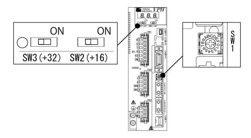
Figure 1-4 Control axis selection switches
