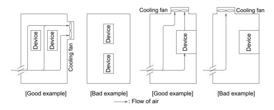
Figure 2-1 Alignment example for storing devices
