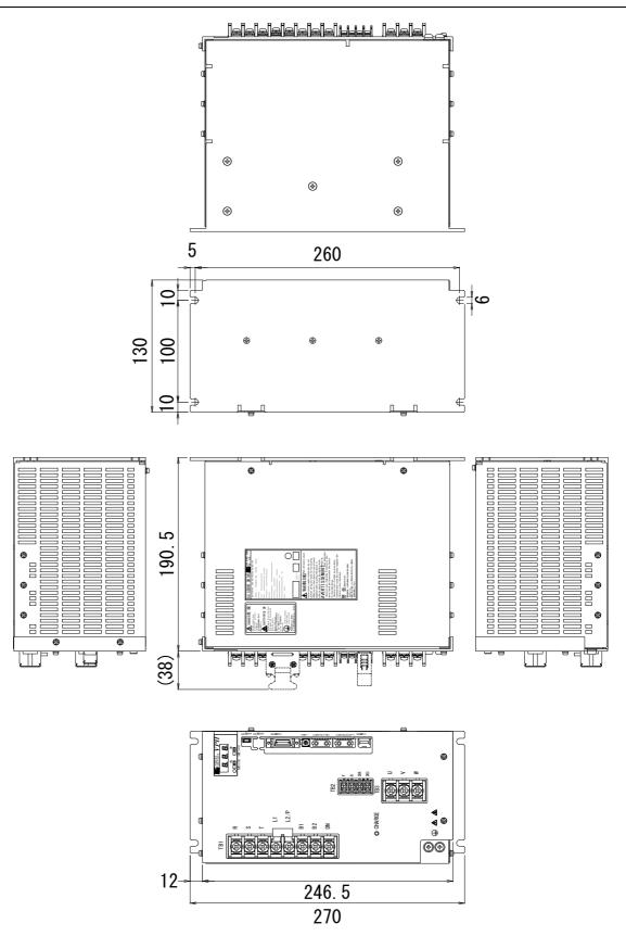
Figure 12-7 Outline drawing of the main unit of the device with 3.3 kW (Type 4)
