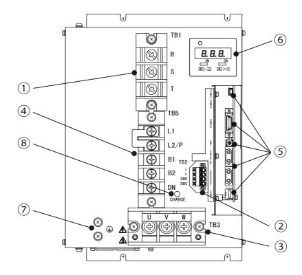
Figure 12-12 Front view of the main unit of the device with 15 kW (Type 6)
