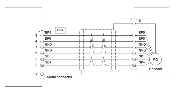
Figure 3-2 Serial encoder connecting diagram
