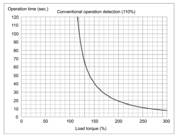
Figure 8-1 Load torque in relation to detection time
