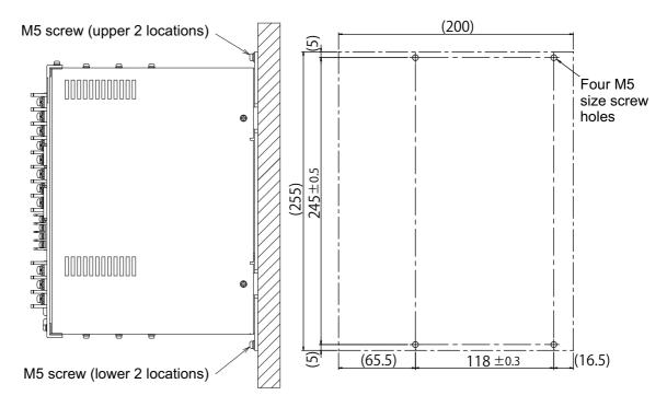
Figure 2-6 Device installation method (7 kW)
