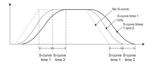
Figure 5-7 S-curve acceleration/deceleration operation example
