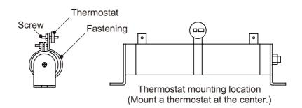
Figure 2-12 Mounting a thermostat on a vitreous enamel resistor
