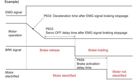
\* In the case of coasting to stop ([P633 (1st digit)] = Servo OFF), the motor operates as described in ① or ② above.
