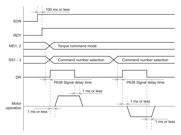
Figure 5-3 Internal torque command time chart
