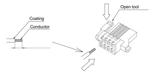
Figure 2-13 Plug connector wiring diagram
