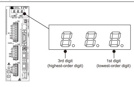
Figure 1-3 Appearance of the data display LED panel
