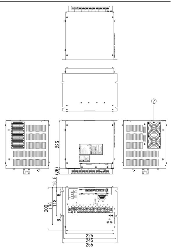
Figure 12-9 Outline drawing of the main unit of the device with 7 kW (Type 5)
