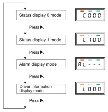
Figure 10-1 Status display mode configuration and transition
