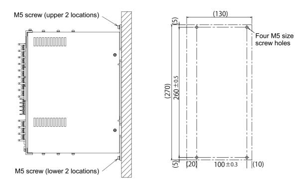
Figure 2-5 Device installation method (3.3 kW)
