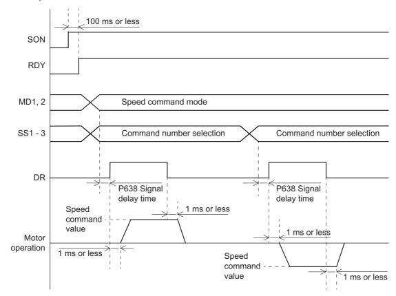
Figure 5-3 Internal speed command time chart
