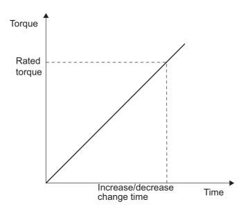
Figure 5-9 Torque command increase/decrease change in relation to rated torque
