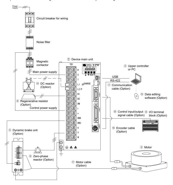
Figure 1-2 VPH HA Type system configuration for the 1.5 kW class or more
