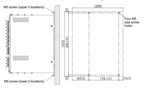
Figure 2-6 Device installation method (7 kW)
