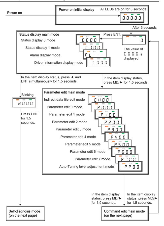
Figure 12-2 Operation mode configuration and transition (1/2)
