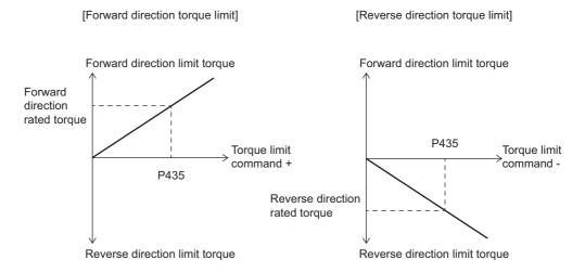
Figure 5-13 Torque limit with the analog torque command
