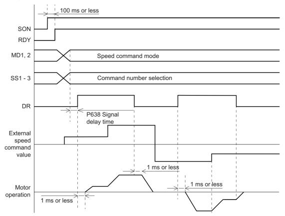
Figure 5-2 Analog speed command time chart
