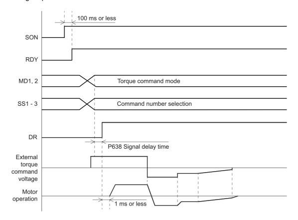
Figure 5-7 Analog torque command time chart
