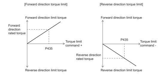
Figure 5-5 Torque limit with the analog torque command
