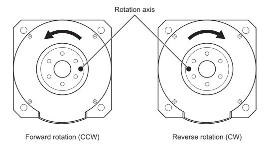
Figure 4-1 Run direction of the τDISC motor
