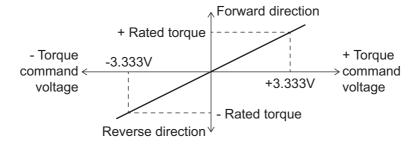
Figure 5-6 Analog torque command in relation to motor output torque
