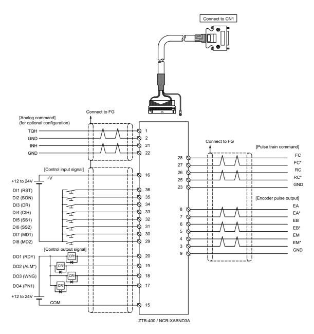
Figure 3-3 I/O terminal block (option) connecting diagram
