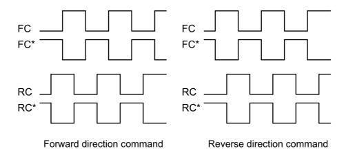
Figure 3-4 90 deg phase difference signals
