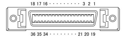
The figure below is the connector alignment of the cable side viewed from the soldering terminal side.
