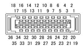
Table 3-1 Control input/output connector pin alignment
