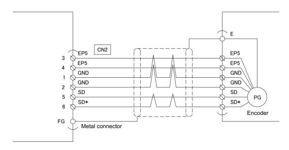
Figure 3-2 Serial encoder connecting diagram
