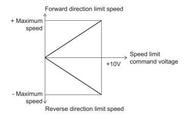
Figure 5-10 Speed limit with the analog speed command
