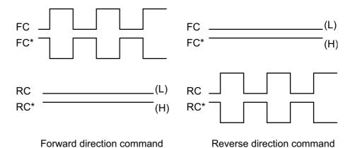
Figure 3-5 Direction-specific pulses
