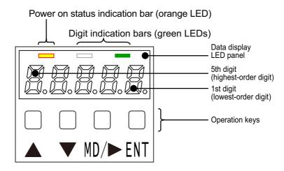
Figure 12-1 Configuration of the operation panel
