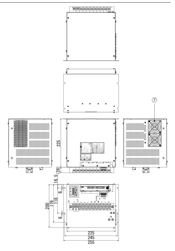
Figure 13-9 Outline drawing of the main unit of the device with 7 kW (Type 5)
