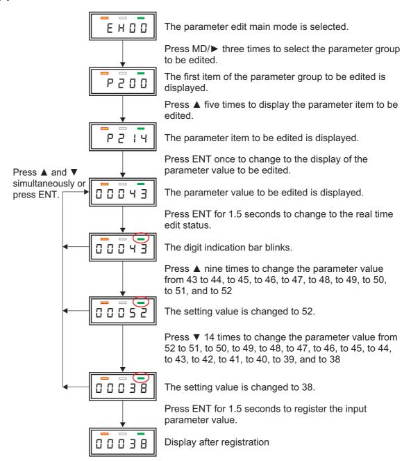
Figure 12-8 Changing P214 parameter value (up to 5 digits) from 00043 to 00052 and to 00038
