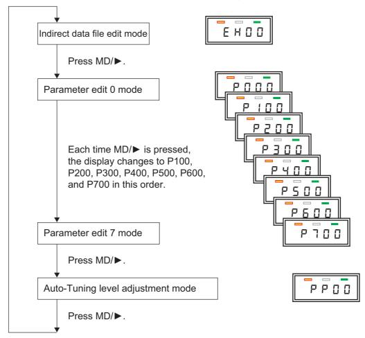
Figure 12-4 Parameter edit mode configuration and transition
