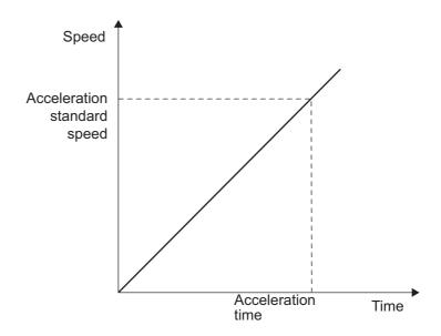
Figure 5-4 Acceleration standard speed in relation to acceleration time at speed command mode
