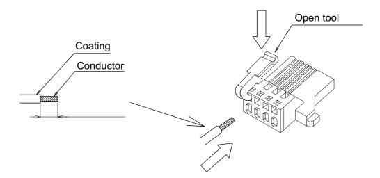
Figure 2-13 Plug connector wiring diagram
