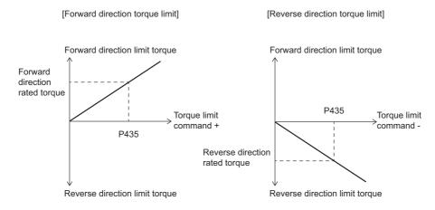
Figure 5-17 Torque limit with the analog torque command
