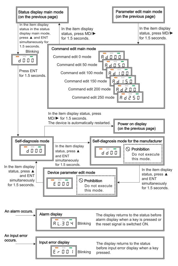
Figure 12-3 Operation mode configuration and transition (2/2)
