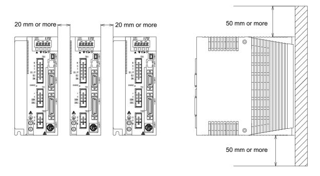
Figure 2-2 Installation and ventilation of the device
