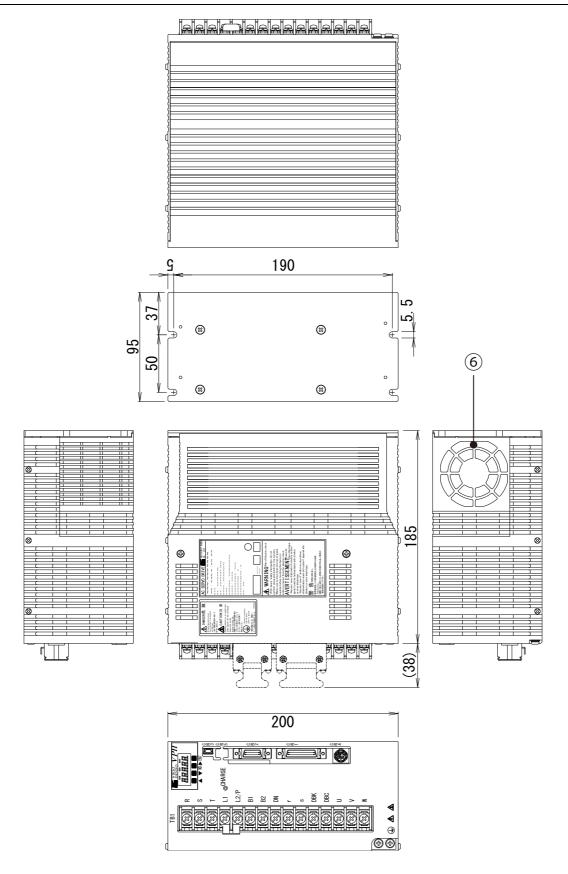
Figure 13-5 Outline drawing of the main unit of the device with 1.5 kW or 2.2 kW (Type 3)
