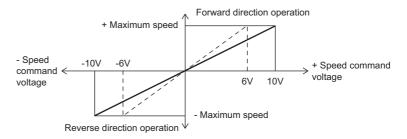
Figure 5-1 Analog speed command in relation to motor operation speed
