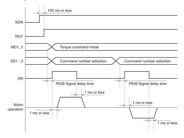
Figure 5-8 Internal torque command time chart
