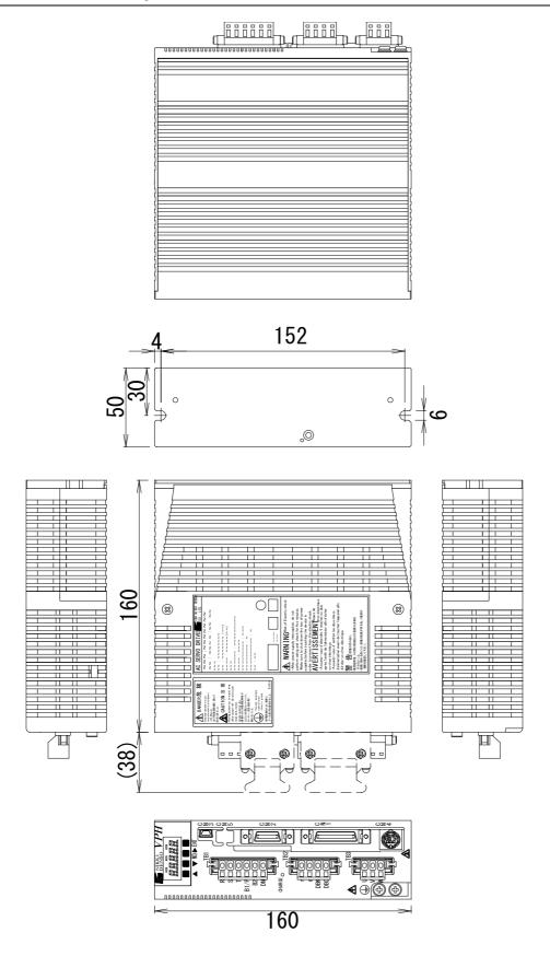
Figure 13-1 Outline drawing of the main unit of the device with up to 400 W (Type 1)
