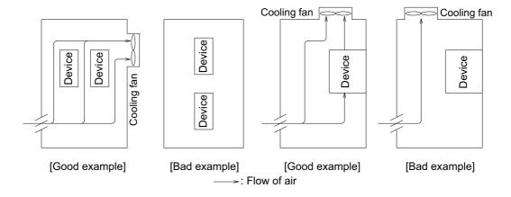
Figure 2-1 Alignment example for storing devices
