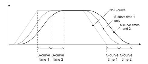
Figure 5-16 S-curve acceleration/deceleration operation example
