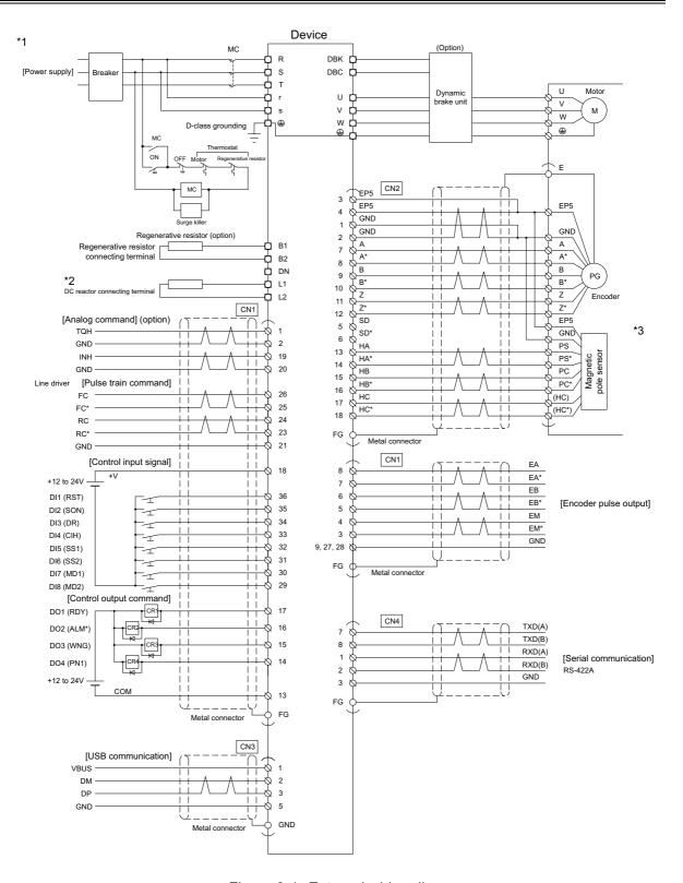
Figure 3-1 External wiring diagram
