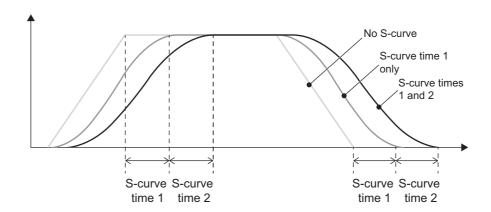
Figure 5-12 S-curve acceleration/deceleration operation example
