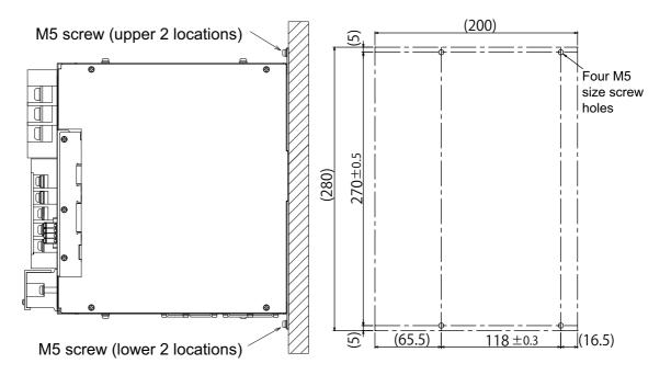
Figure 2-7 Device installation method (15 kW)
