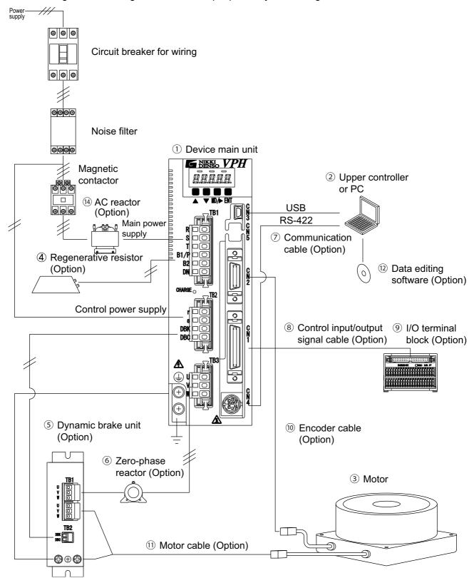
Figure 1-1 VPH HA Type system configuration for the 800 W class or less
