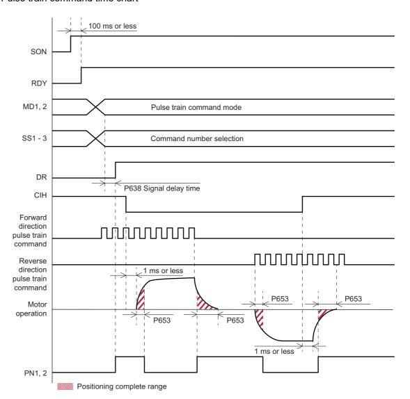
Figure 5-11 Pulse train command time chart
