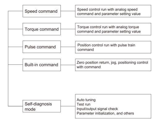
Figure 1-3 Mode configuration diagram
