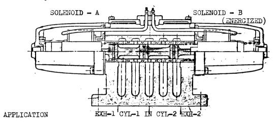
FDO Series valves combine a standard 4-way action with a neutral position (Solenoid de-energized) in which all ports are open and air is exhausted in both ends of the cylinder.
