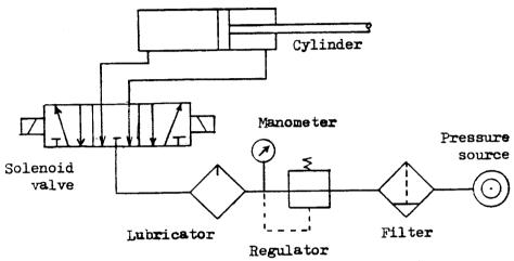
1. Clean pipes (inside) as thoroughly as possible before fixing an electro-magnetic valve.
