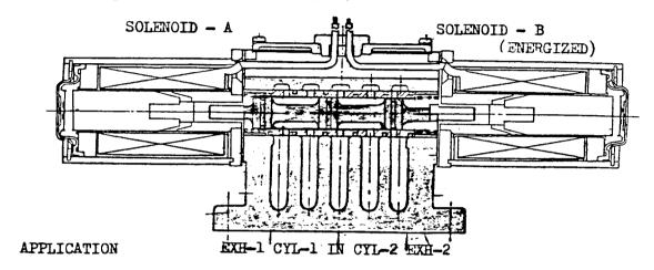
FDO Series valves combine a standard 4-way action with a neutral position (Solenoid de-energized) in which all ports are open and air is exhausted in both ends of the cylinder.
