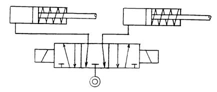
These valve may be used as dual pressure 4-way or 3-way by piping tow pressures into exhaust ports "EXH-1" & "EXH-2". The center port "IN" then becomes a common exhaust.
