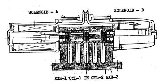
FDO Series Valves are direct solenoid operated, spring centered, 3-position, 4-way air valves.
