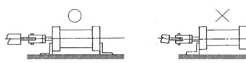
Prevent fixedly connection of excessive load to Rod. Damage to the rod may be caused due to large kinetic energy.
