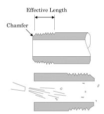
6) Refrain from applying sealant or sealing tape approx. two pitches of thread off the tip of pipe to avoid residual substances from falling into piping system.
