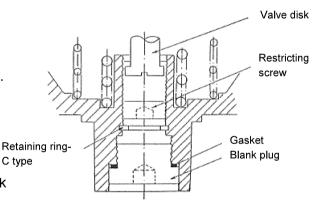
Note) When adjust the flow rate of the valve with micro switch inside (HK1E, HK1E-B, HK1E-ZZ type), the electric signal of the valve position may not be detected.
