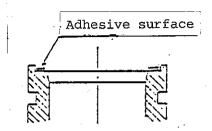
f) Insert the rubber flange into the body flange groove and adhere the rubber sleeve and rubber flange. As the rubber sleeve and rubber flange surfaces are not uniform, hold them for some time until they are completely adhered. Use the above procedure for both flanges.
