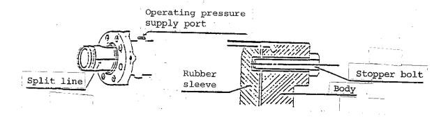
e) Apply an appropriate amount of instant adhesive to the flange surface with the rubber sleeve position unchanged. (Too much adhesive requires time until the flange is completely adhered.)
