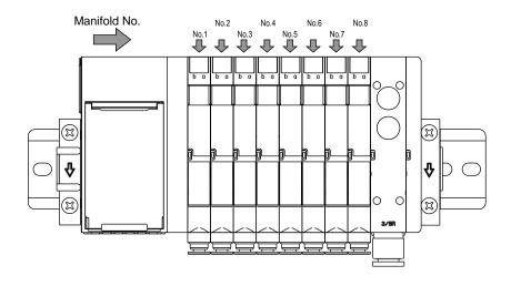
The figure is an example of mounting eight stations of double-solenoid type valves. There is no solenoid on the b-side for single-solenoid type.
