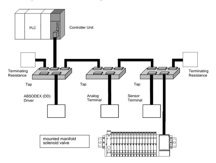
Controller unit: A unit which controls device units and requests to open connection. Tap: A device which is used for branch connection.
