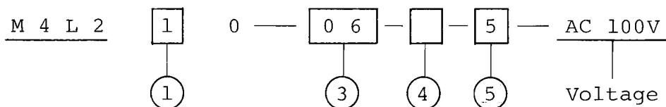
\* The model number shown above means 4L2 manifold, 2-position single solenoid, solenoid valve, connecting pipe size, A·B port PT 1/8, P·R1·R2 port PT 1/4, 5 series, AC 100V, and 50/60 Hz.
