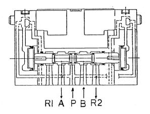
3-position closed center (4L230) 3-position exhaust center (4L240)
