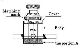
12) To mount or remove the bracket, hold the octagonal portion of the cover with a spanner or other tool to keep the alignment between the matching marks on the body and the cover. Then, firmly tighten or loosen the panel mount nut. To change the position of the bracket, lock the octagonal portion of the cover and loosen the panel mount nut.
