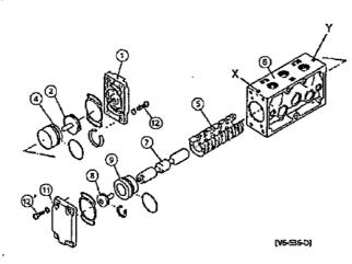
Carefully place each components during disassembling work because the positions and direction of piston ass'y ②,®, cylinders ④, ⑨ and seal ass'y ⑤ are fixed.
