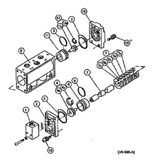
Carefully place each components during disassembling work because the positions and direction of piston ass'y ④ ②, cylinders ⑧ ① and seal ass'y ⑤ are fixed.
