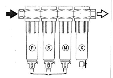
Drain discharge port of P·S·M series is Rc1/8.
