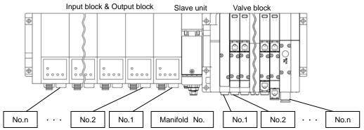
2) Example of Valve No. assignments corresponding to Slave Unit Solenoid Output No Valve Nos. 1a, 1b, 2a, 2b, etc., Number indicate the first and second stations. Letters a and b refer to solenoid a or solenoid b.
