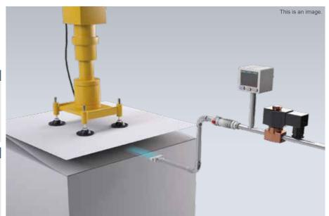
Prevents overlap in transport of thin workpieces by using a flat air nozzle that blows uniformly into various crevices. Can also be used to prevent overlap in suction of thin oily boards.
