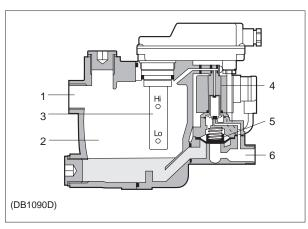
● DB Series double sensor (DB1090D/3090D, DB3700)
