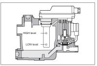
HIGH and LOW level sensors discharge drainage only, preventing wasteful air consumption. (DB1090D/3090D/3700)
