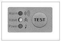
The electronic circuit with self-diagnosis function constantly monitors the discharge status displaying it with LEDs. (excluding DB3003D)
