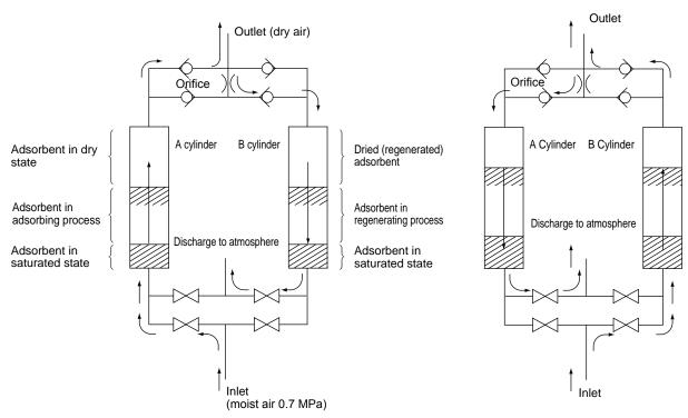
Moist air coming in from the inlet will enter the A cylinder, have its moisture removed due to the adsorbent, and then leave from the outlet as dry air. Part of the dry air coming out of the A cylinder will flow through the orifice, be reduced in pressure to an atmospheric pressure, enter the B cylinder, remove moisture from the moist adsorbent, and be exhausted into the air.
