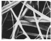
High 96% porosity inside the element fibers helps achieve low pressure loss and a long life
