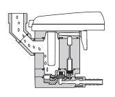
Lower water level is detected again and drainage stops
