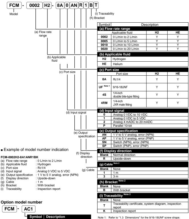
AC1 Analog 9-conductor cable, 1 m Note 2: Items (g), (h), and (i) are delivered with the product when selected. AC3 Analog 9-conductor cable, 3 m
