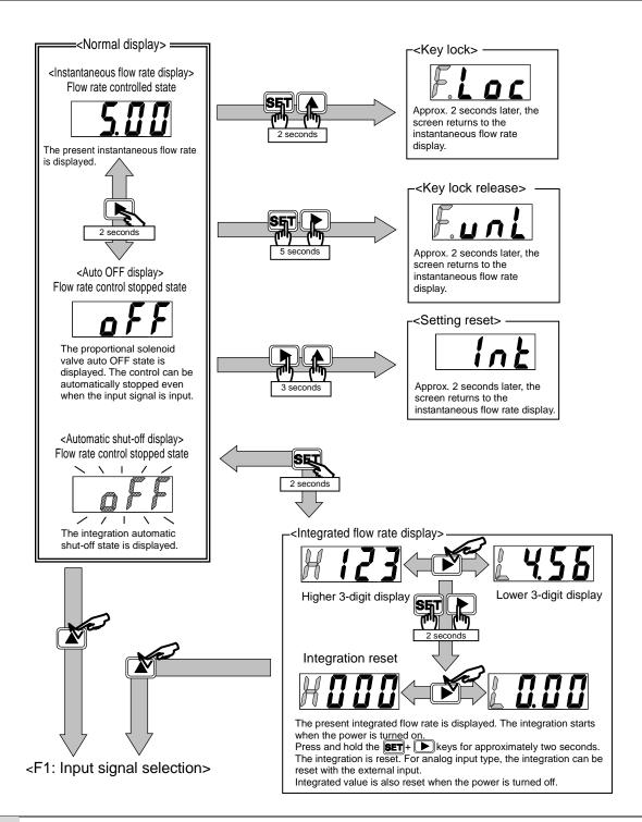
The key lock is disabled before shipping from the factory. Lock the key as necessary. The key lock state (enabled/disabled) is maintained even if the power is turned off.
