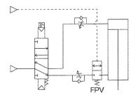
•Used in cylinder intermediate stop circuit
