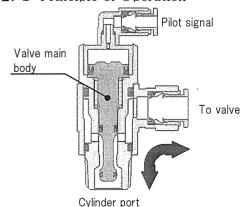
When a pilot signal is present, the valve main body opens, connecting the valve and cylinder. When no pilot signal is present, however, the valve main body is closed, cutting off the valve and cylinder port.
