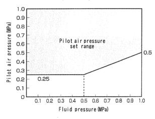
The pilot air pressure in which the fluid pressure is 0.5 MPa max. must be 0.25 MPa or higher.
