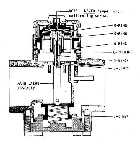
The factory packs all moving seals with a heavy lubricating grease. Under normal conditions this will last through millions of cycles. However, under conditions of wet air, unusually high flows, or if light oil from a lubricator somewhere in the circuit gets into the Dial-Air regulator, the original lubricant can be washed out in a relatively short time.
