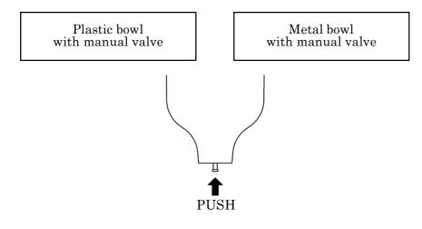
Push up the valve (in the direction indicated by the arrow) to drain the bowl, and release it to stop draining.
