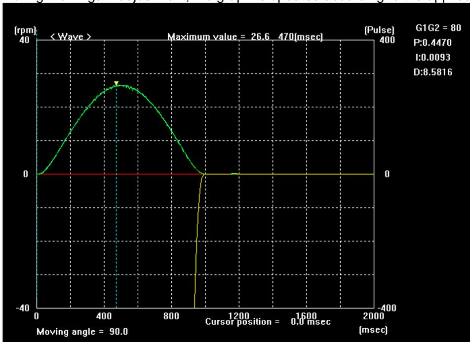
The displayed graph displays the G1 value, G2 value, and PID gain parameter value applied.
