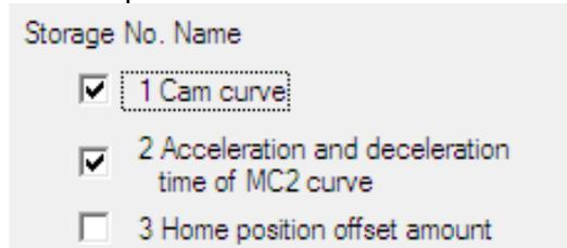
The checkboxes for each parameter determine whether the parameters are stored in ABSODEX. If the checkbox is ticked, the parameter is stored in ABSODEX. If the checkbox is left blank, the parameter is not stored in ABSODEX.
