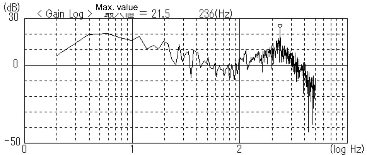
A gain of about 35dB at about 228Hz in the first graph is reduced to about 21dB.
