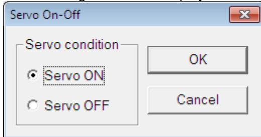
The current servo status is displayed. If the value set in parameter 52 is 1, the status can be changed by selecting ON or OFF and then by clicking the [OK] button.
