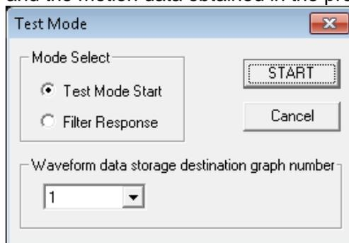
Use [Test Mode Start] to observe the response of the actuator. Use [Filter Response] to observe the response of the filter.
