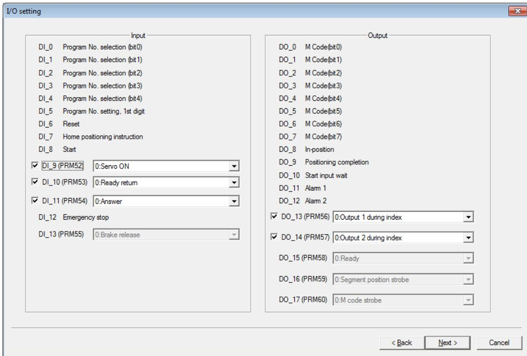
※The I/O setting function can be used with TS, TH, MU and XS type drivers.
