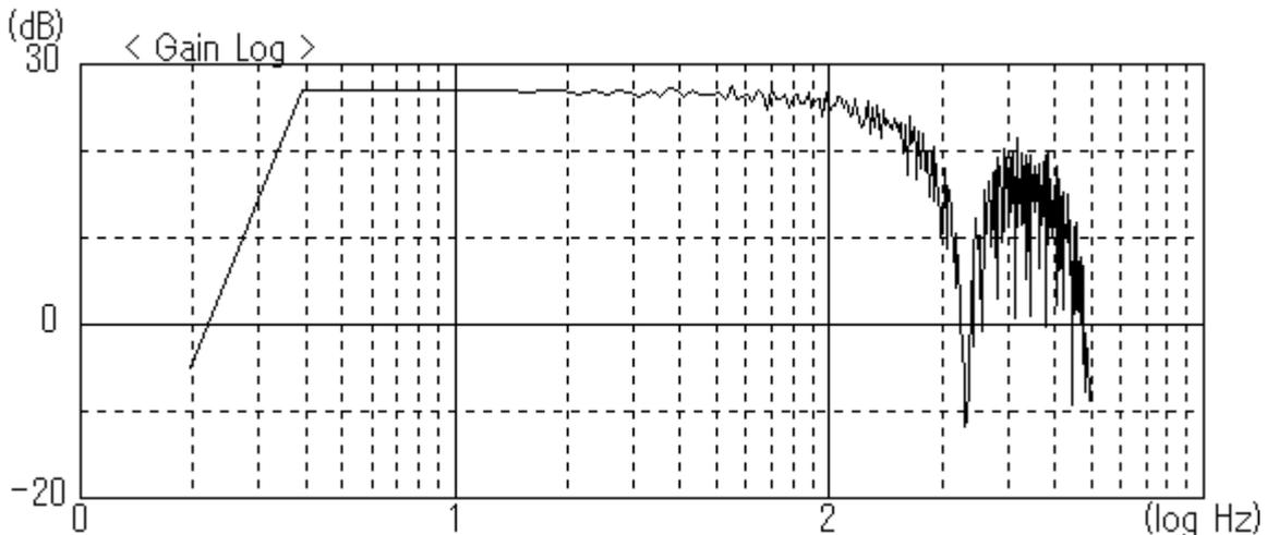
Because the low pass filter is set at 200Hz, the right side of the graph line declines after "200Hz."
