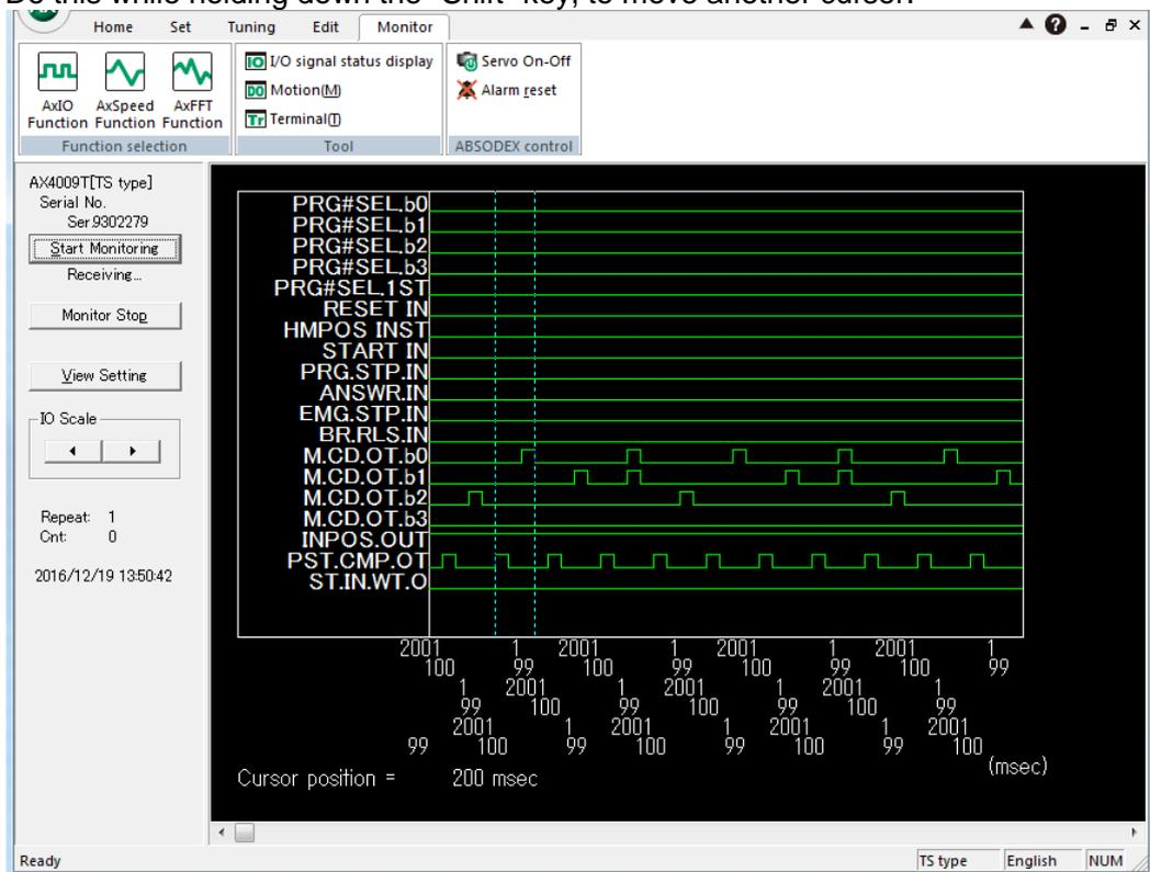
Click the right mouse button to display the interval between signals at a time.
