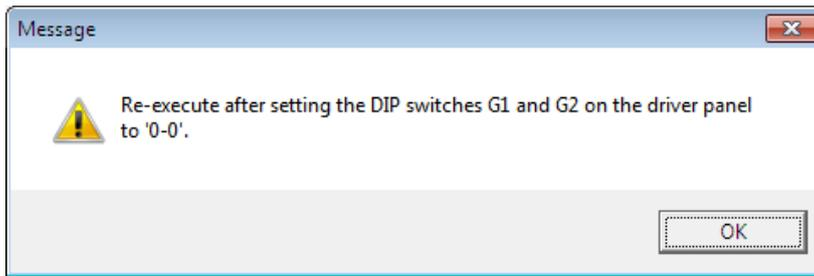
Adjust the DIP switches to "0 - 0", and click the [OK] button.
