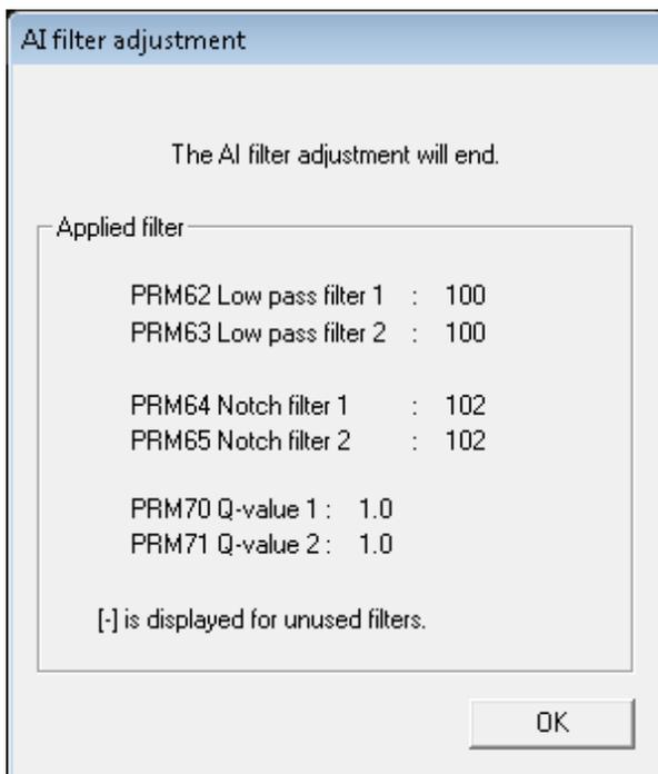
As the AI filter adjustment result, the set digital filter setting is displayed.
