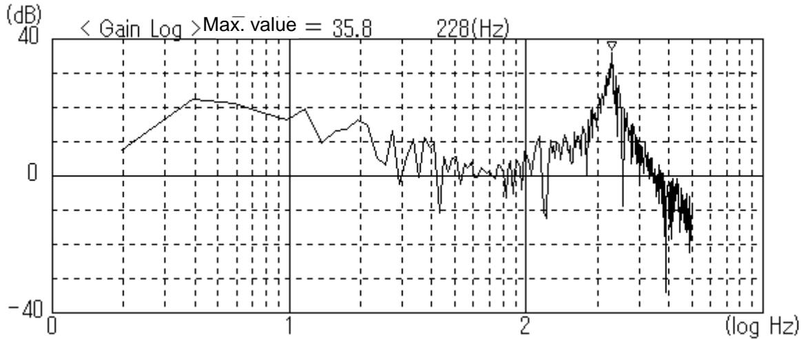
Because resonance is observed at about 228Hz, specify "228" for notch filter 1 to reduce the gain of the resonance point.
