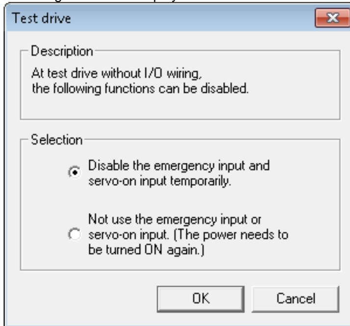
1. Disable the emergency input and servo-on input temporarily.
