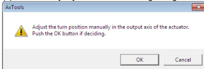
(4) Click the [OK] button after adjusting the position manually.
