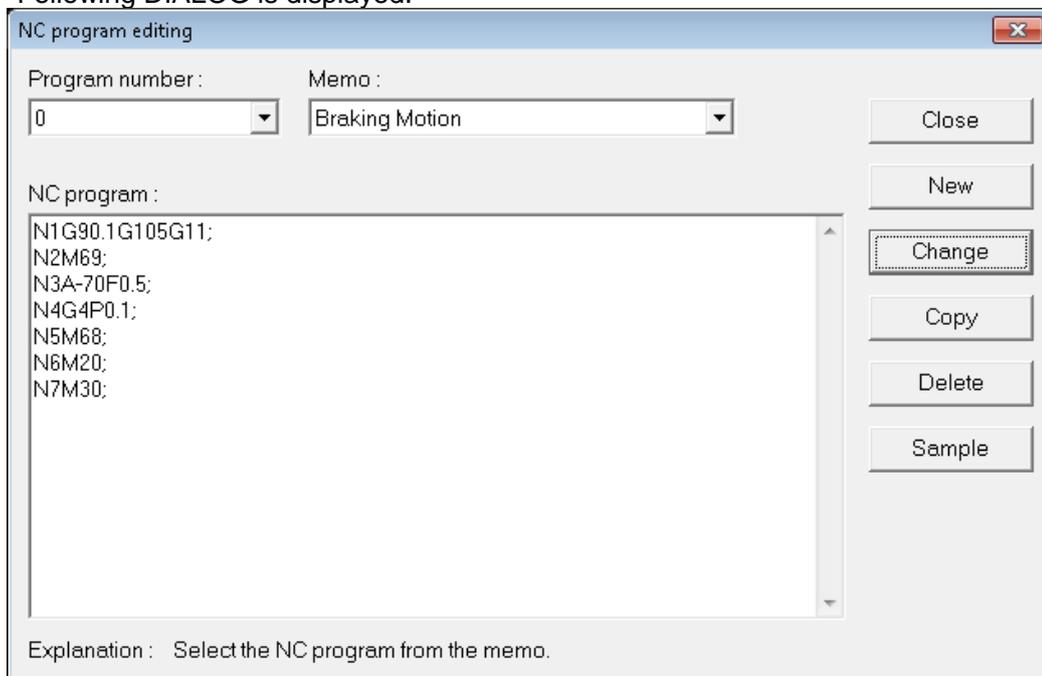
The contents of each input are displayed in "Explanation :" on display screen.
