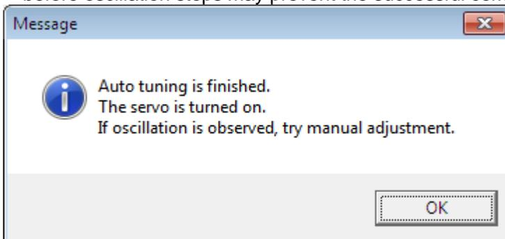
※If the gain adjustment DIP switches G1 and G2 on the driver panel are not '0 - 0' the dialog box shown below is displayed.
