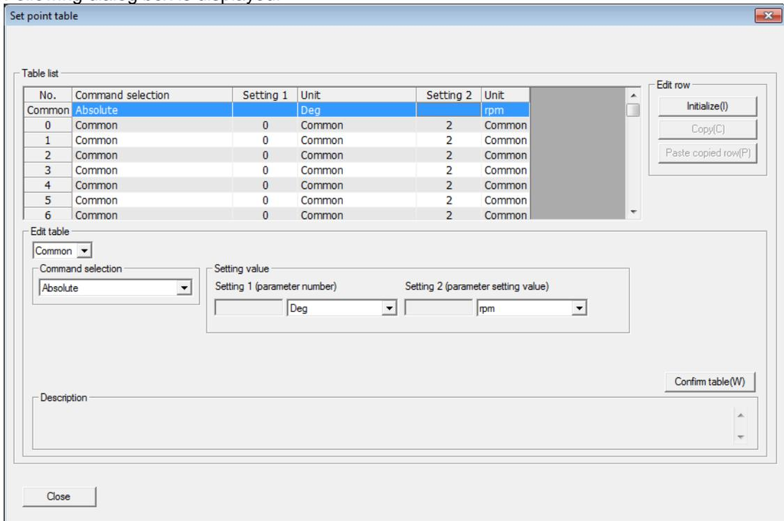
The contents of each input are displayed in "Explanation" on display screen.
