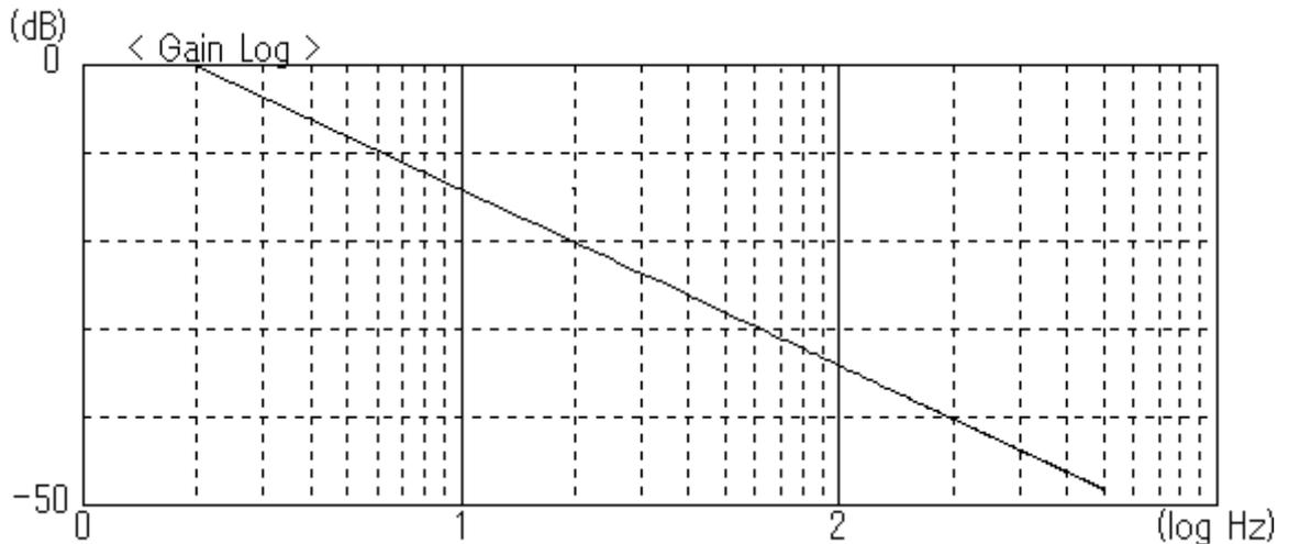
If there is resonance, projection or swelling is observed near the resonance frequencies in this gain waveform.
