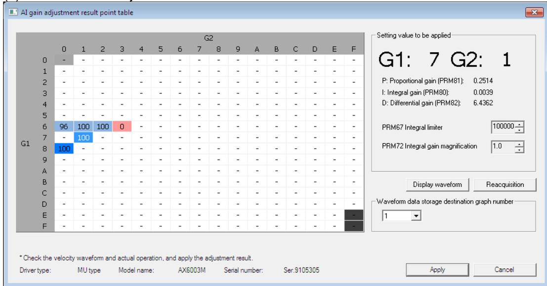
(2) When the file saving the AI Gain adjustment execution result (extension [.axa]) is opened
