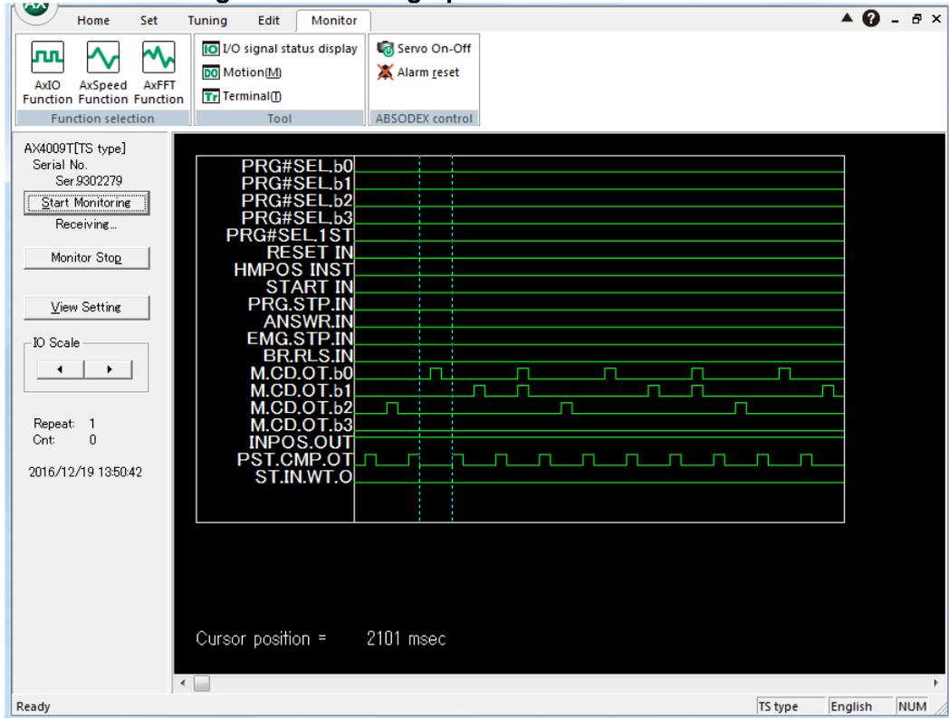
If you click and drag the mouse, "Cursor position" below the graph shows the time between the cursor movement starting and ending positions.
