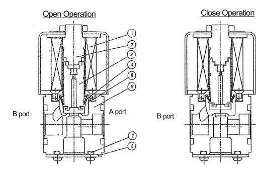
PLUNGER ASS'Y ③ absorbs CORE ASS'Y ② when energizing to the Coil ① ,and the Valve Sheet opens.
