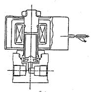
When the coil 1 is de-energized, the plunger 4 lowers down due to the force of spring 3 to close the valve seat 5. Then the chamber A and B closes.
