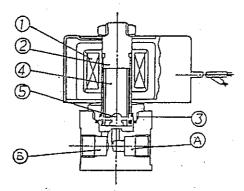
When the coil (1) is energized, the fixed iron core (2) absorbs the plunger (4) to open the valve seat (5). Then the chambers (A) and (B) open.
