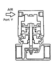
Charging air into port Y lowers the main valve plate (of the piston assembly (2)) which causes the valve seat to close, sealing the fluid.
