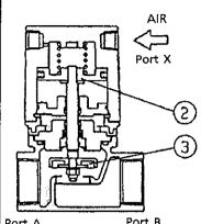
Charging compressed air into port X raises the main valve plate ③(of the piston assembly②) which causes the valve seat to open, allowing the fluid to flow.
