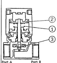
Removing air from port Y allows the spring①to raise the main valve plate③(of the piston assembly②) which causes the valve seat to open, allowing the fluid to flow.
