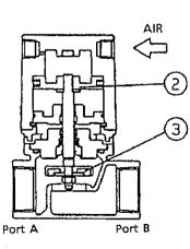
Charging compressed air into port X and, at the same time, discharging air from port Y, raises the main vaive plate (of the piston assembly ) which causes the valve seat to open, allowing the fluid to flow.
