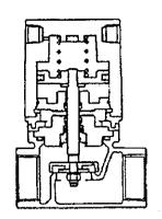
Discharging compressed air charged in port X allows the spring ①to lower the main valve plate(of the piston assembly②) which closes the valve seat, sealing the fluid.
