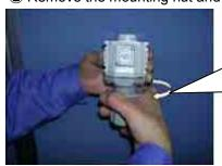
The knob goes off with turn of mounting nut. (Turn needs a slight force)
