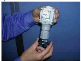
4 Tighten the mounting nut.
