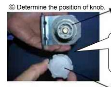
Align □ mark of knob with the □ position of adjusting screw and put the knob on.
