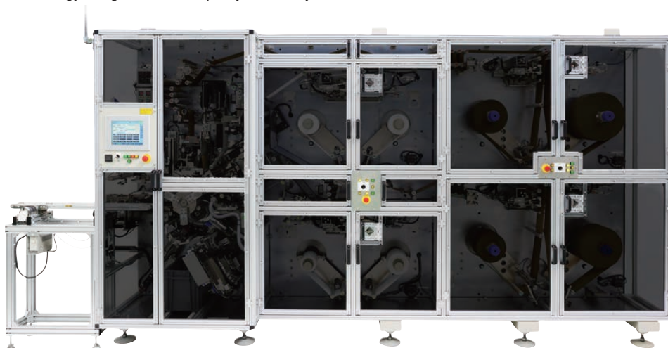
Winding machines for lithium-ion batteries
